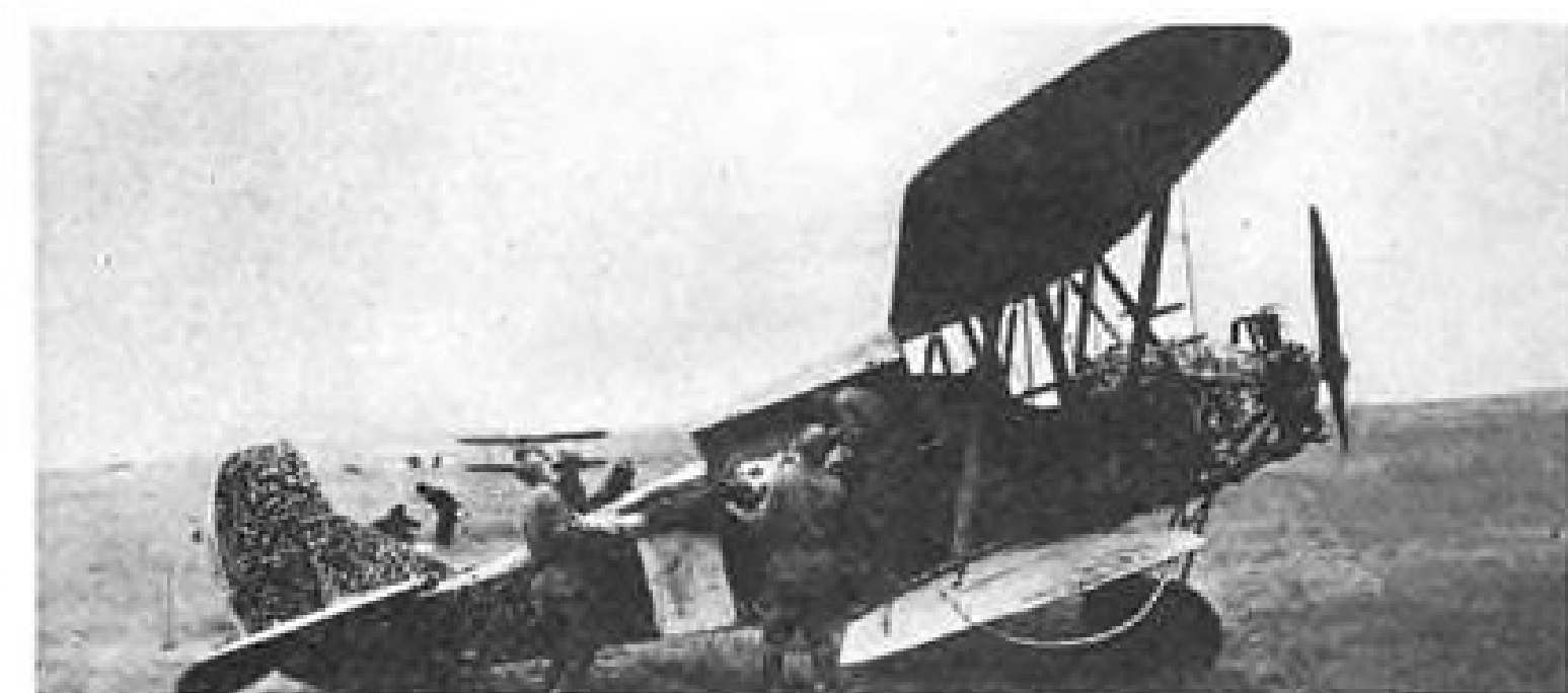
M-11F, 145-HP. radial developed from French Lorraine 5P, powers trainers such as U-2 and UT-2, which have been in service since before World War II. Larger versions of the M-5 have not been used extensively.
