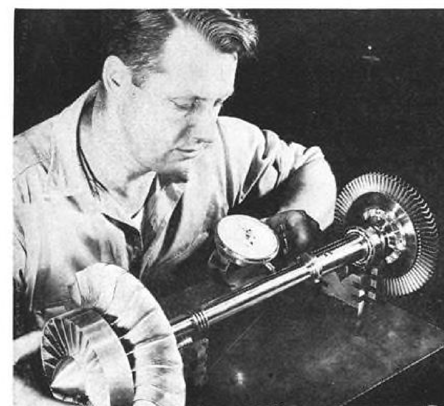
COMPRESSOR AND TURBINE of Boeing Aircraft Model 500 turbojet which develops 150 lb. static sea level thrust for weight of 85 lb. Though reportedly built solely to gain research information, unit is seen readily available as auxiliary power plant for large aircraft.
