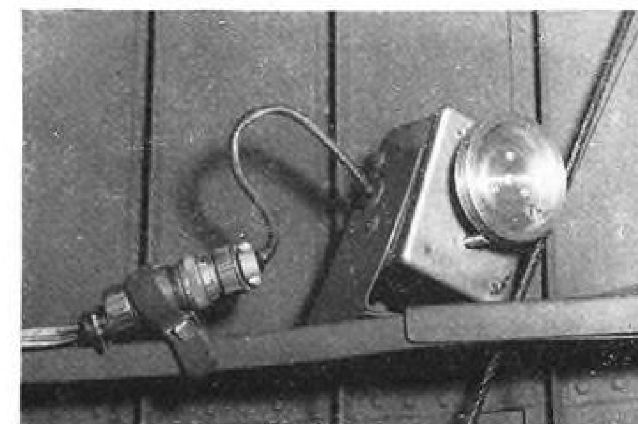
SELSYN MOUNTING: Selsyn transmitters are linked by braided steel cables to B-45 control systems. To provide extreme accuracy of readings, each transmitter actually contains two selsyns, one geared to rotate at four times speed of other. On indicator dial in photo recorder one pointer makes four revolutions to one revolution of other pointer.
