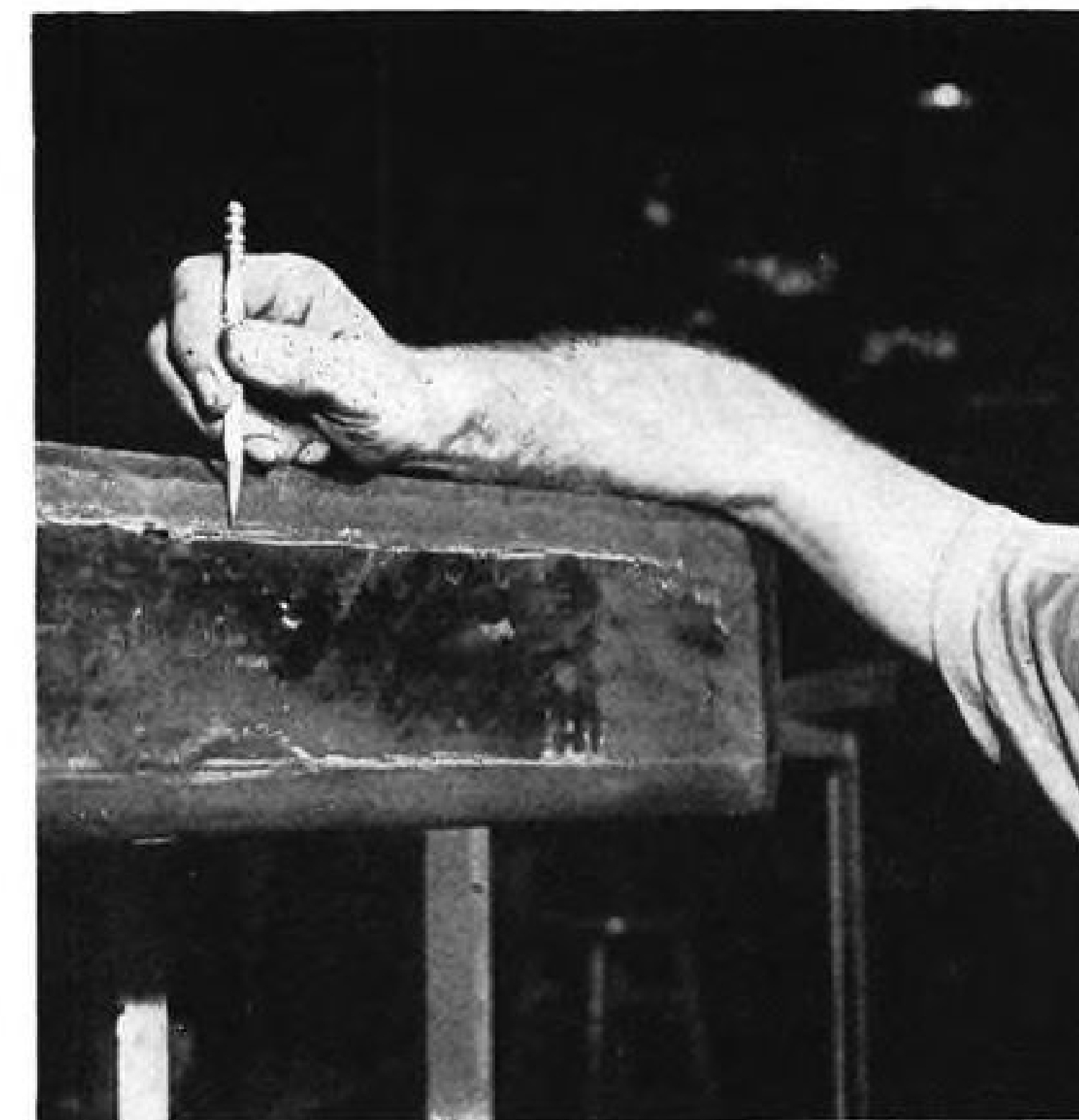
INDICATED BY PENCIL is seam where 1-in. layer of new rubber is vulcanized to old hydropress pad to boost its life.
