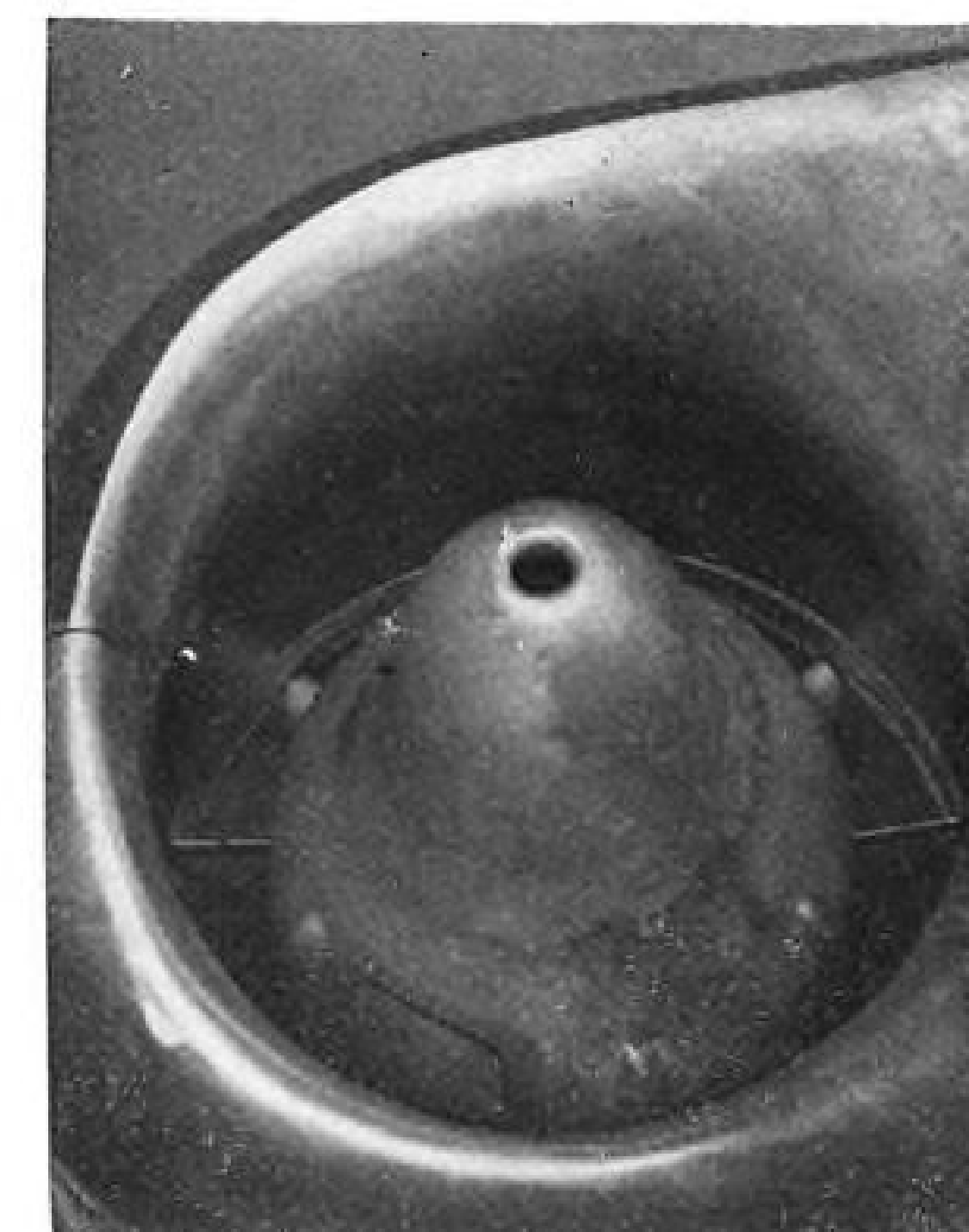
MEASURING INTAKE: Symmetrically-located pitot tube rakes are shown mounted within B-45 engine air inlet duct. For recording air flow at this point North American chose to connect tubes to F-1 sensitive air speed indicators rather than direct-reading pressure gages. Easier reading and greater accuracy was obtained.
