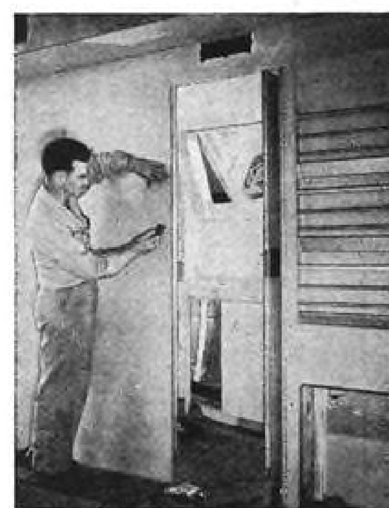
Installing Armorply Honeycomb wall of ladies' dressing room in the Boeing 377 Stratocruiser.
