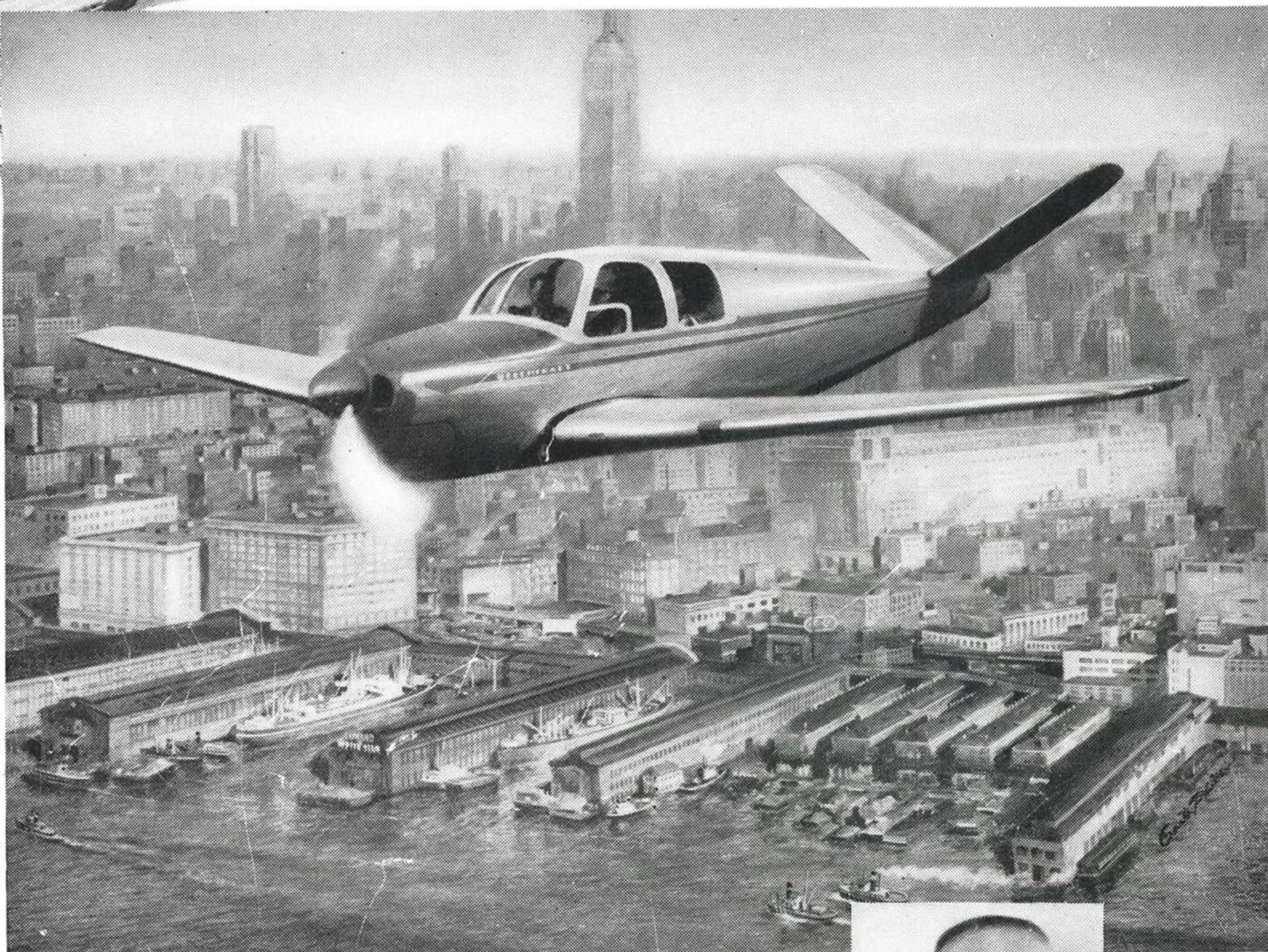
Top Speed, 184 mph; Cruising Speed, 172 mph; Range, 750 miles
