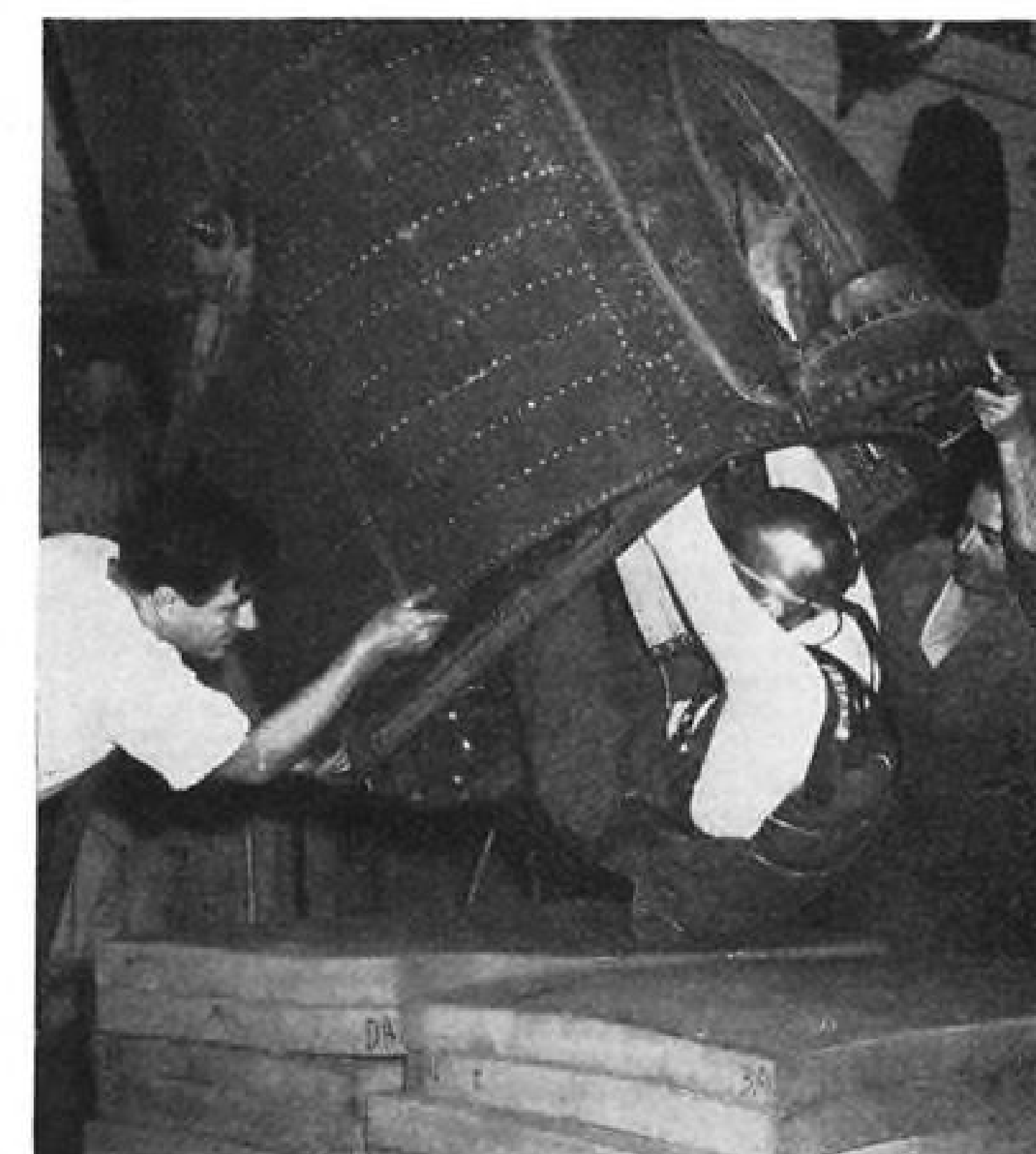
Photos show two methods of leaving nose section after emergency detachment. At left pilot rolls out. At right pilot backs from cockpit.
