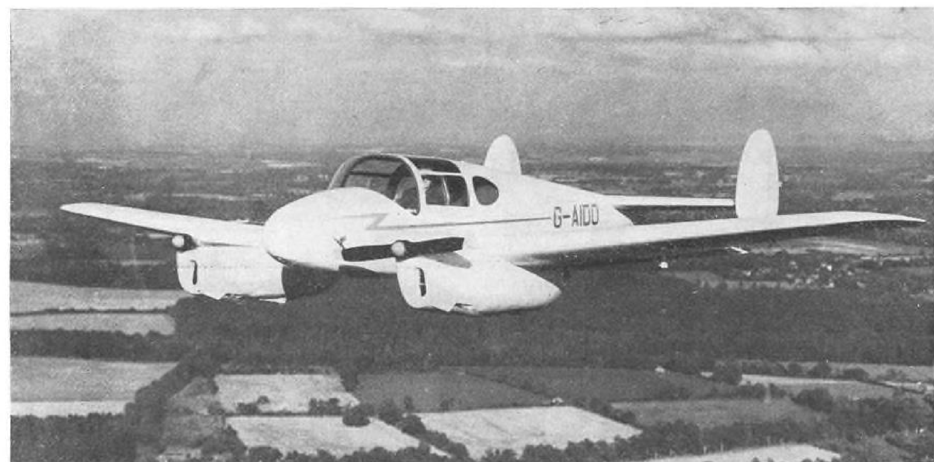
Three-quarter view of Miles Gemini flying on one engine (non-featherable prop). Craft has large unobstructed windshield and side windows. Gear retracts into engine nacelles, with wheel bottoms exposed. Photo clearly shows dihedral of wings and clean lines.
