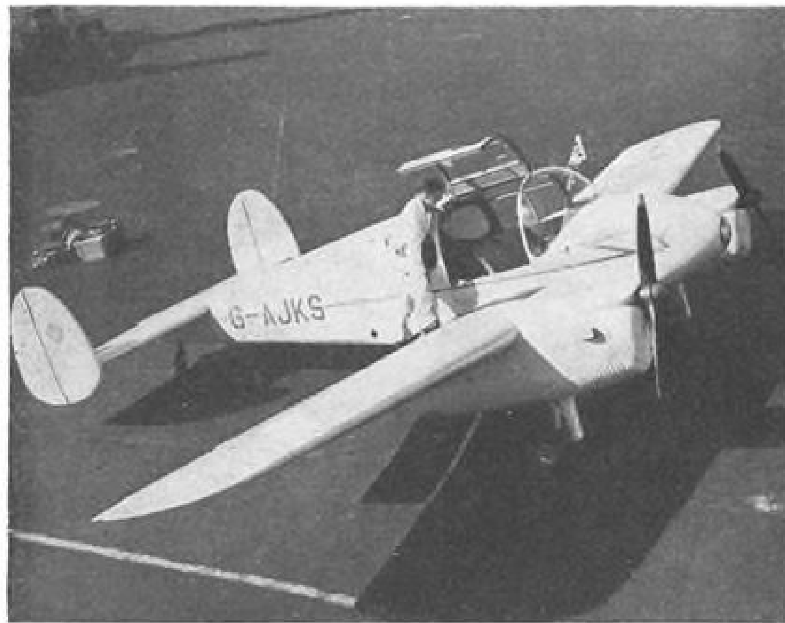
Hatch has left and right liftable sections for quick, easy access from either side of plane. Front right seat has hinged back to facilitate loading. Cockpit (right) affords ample room and the instrument panel features "package" radio equipped with loudspeaker.
