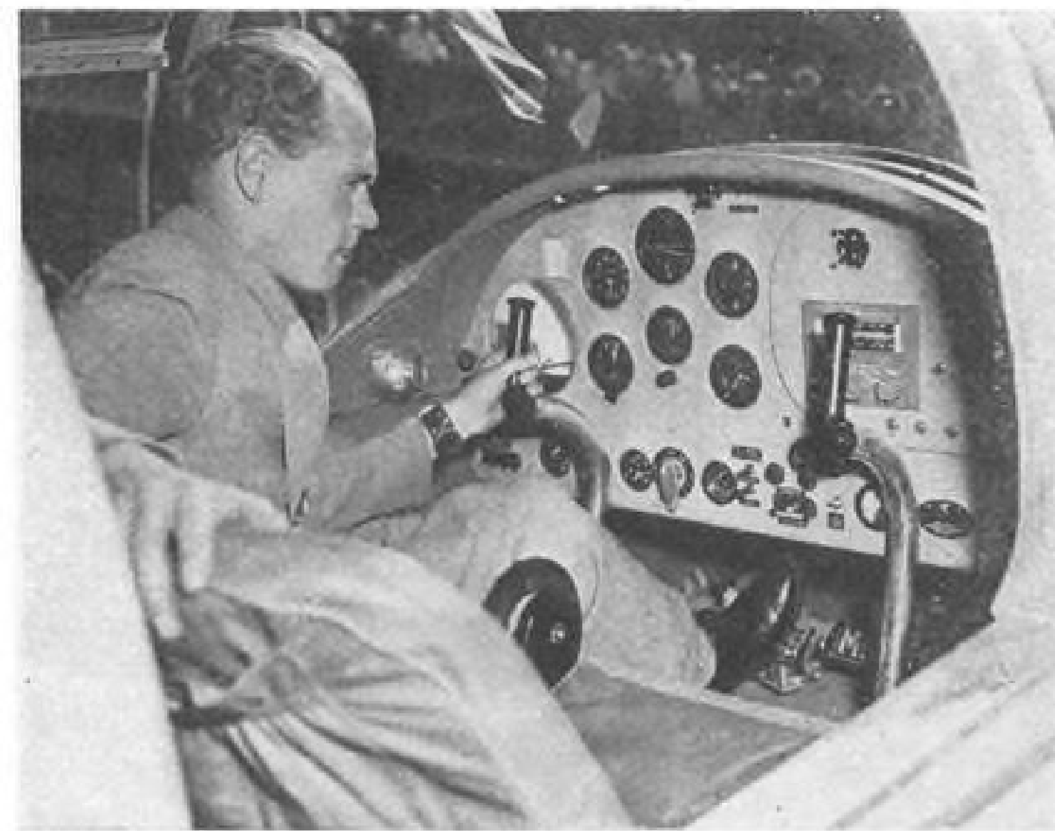
Hatch has left and right liftable sections for quick, easy access from either side of plane. Front right seat has hinged back to facilitate loading. Cockpit (right) affords ample room and the instrument panel features "package" radio equipped with loudspeaker.
