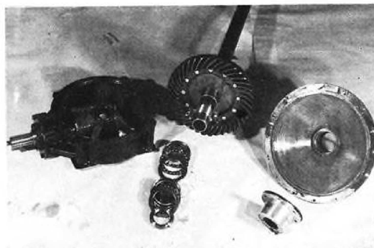
Builder has carried simplification down to transmission. Purpose was to obtain results with standard commercial gears, readily available. Main rotor transmission components are shown. Seibel says gears can be purchased for $35.
