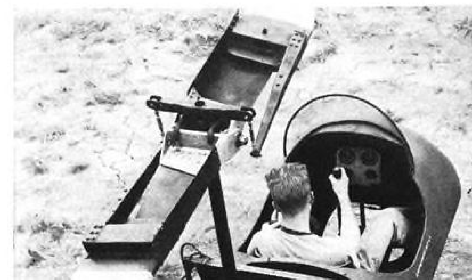
HIGH PITCH: Simplicity of the rotor hub of the Seibel helicopter is apparent. Movement of the blade attaching angle (dark section between lighter blade and hub) controls pitch changes.
