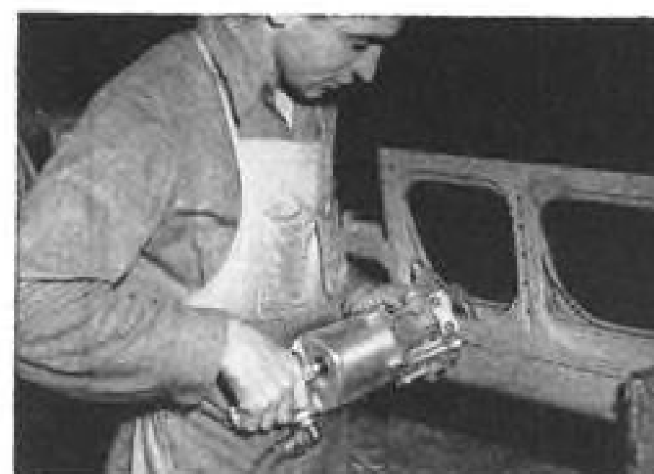
CP-214 Pneumatic Compression Riveter is especially suited for fast work in close quarters . . . its strong "squeeze" action insures exceptionally accurate and uniform results.
