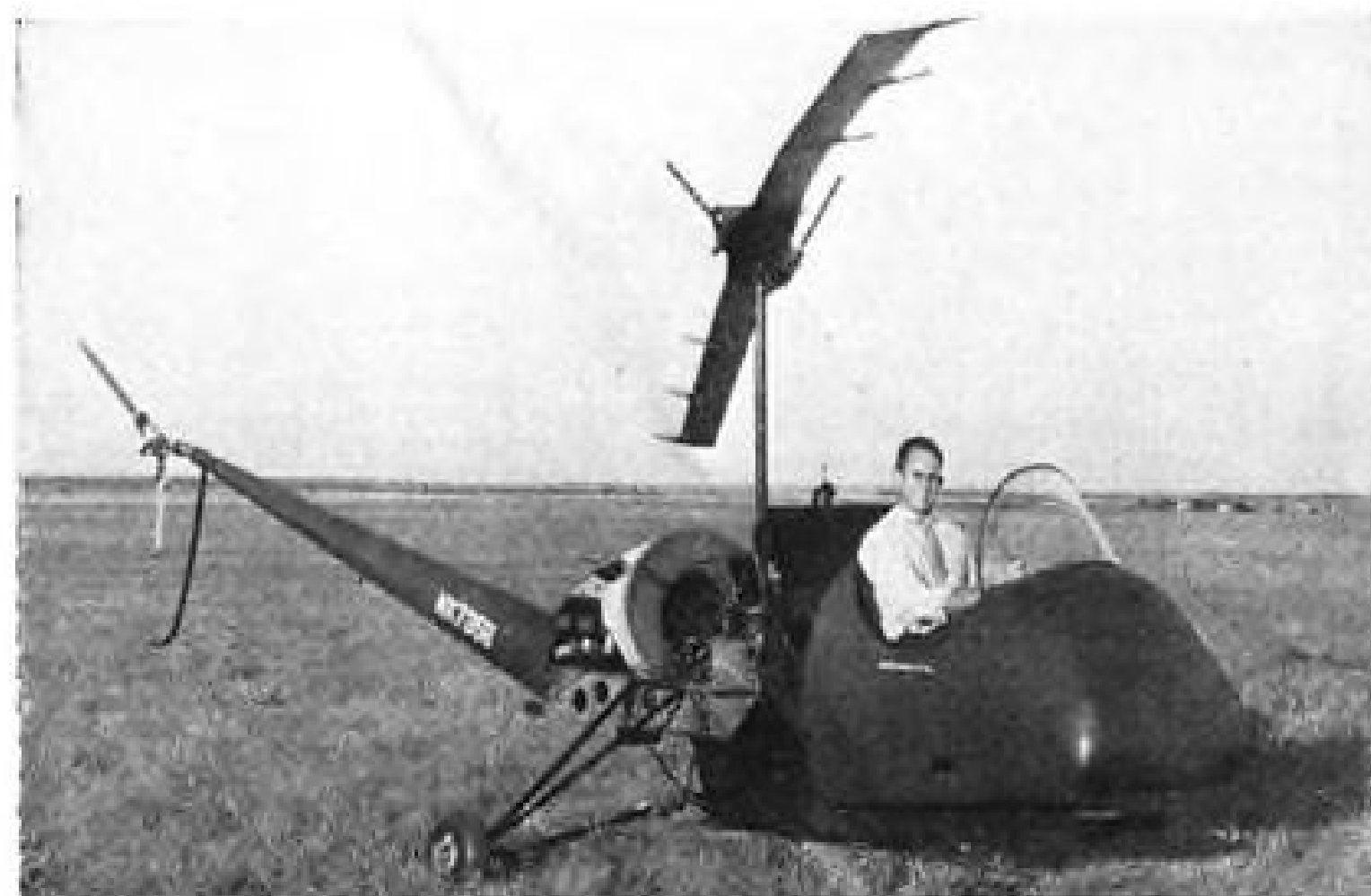
Lateral and longitudinal control is obtained by moving the forward part of the fuselage which slides and pivots on trestle-like structure beneath cockpit. In this view, cabin and central control are in normal neutral position.
