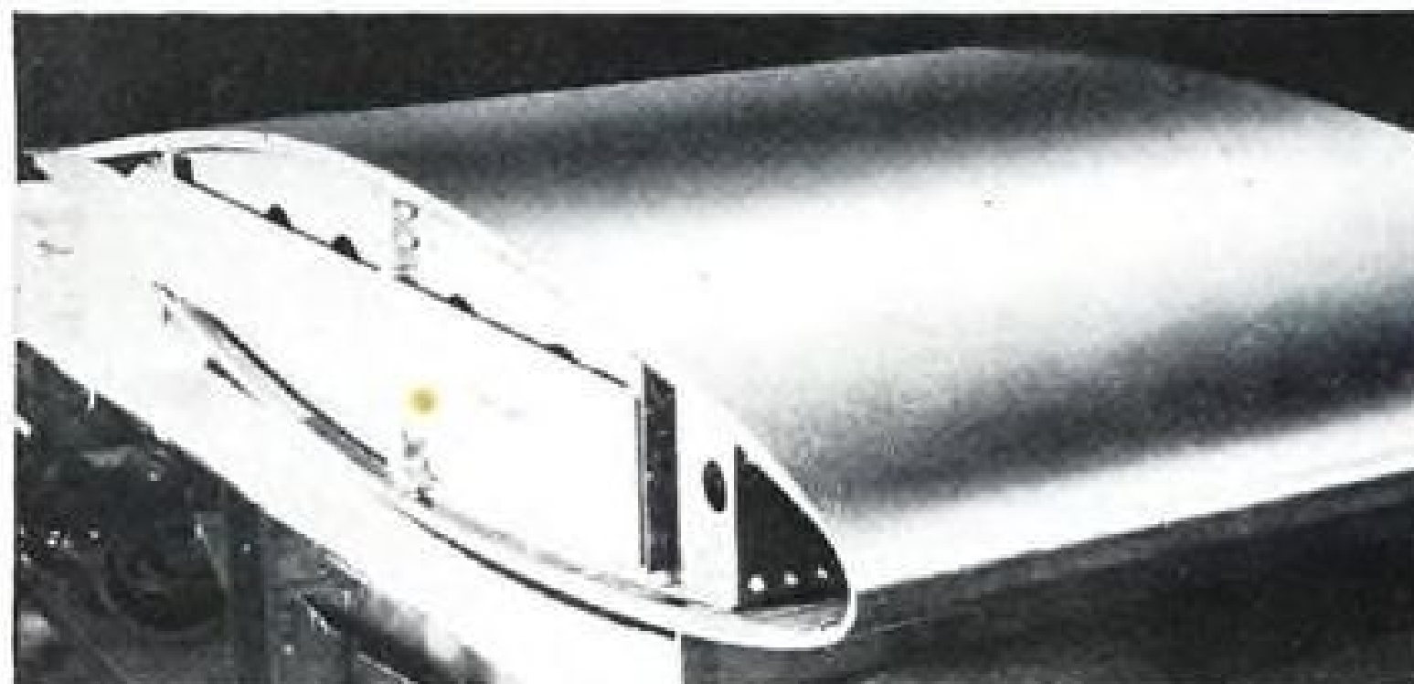
Illustrating sandwich structural material is this wind tunnel model of a Metalite airfoil section—duplicating XF6U-1 construction.
