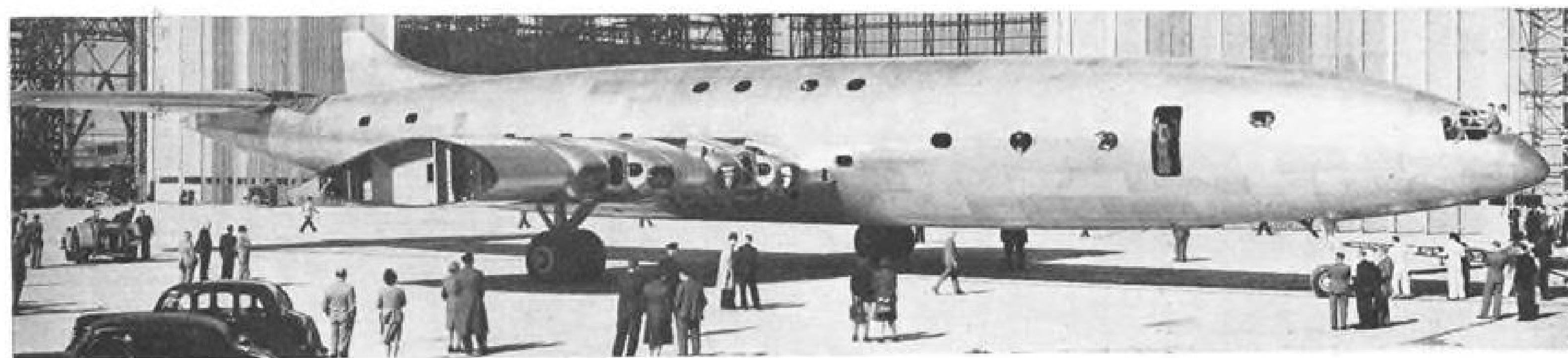
Extreme fuselage length of the Brabazon I shown outside new assembly shop prior to installation of outer wing panels and rudder.
