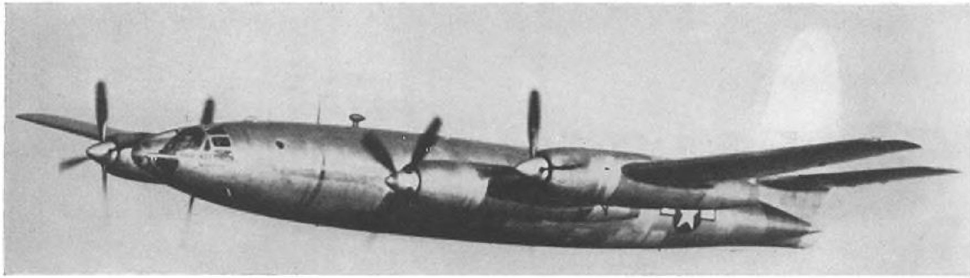
The sharp nose and cylindrical cigar shape of the XF-12 fulfills a designer's dream of no compromise with aerodynamic considerations.
