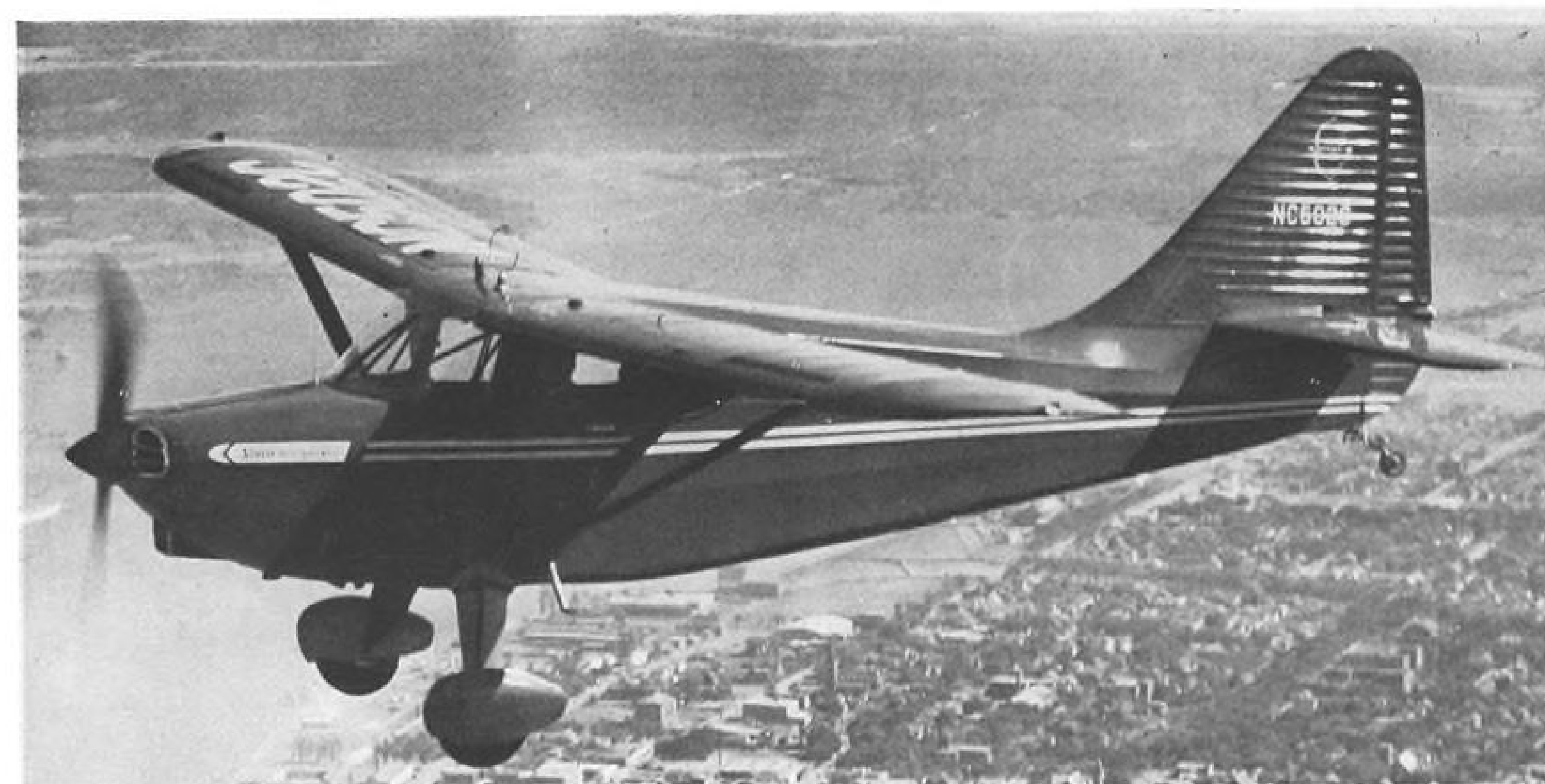
NEW: 1948 Stinson Flying Station Wagon, showing larger tail section, with adjustable rudder trim. New type Vee antenna extends from tail to wing tips. New seats have also been designed.
