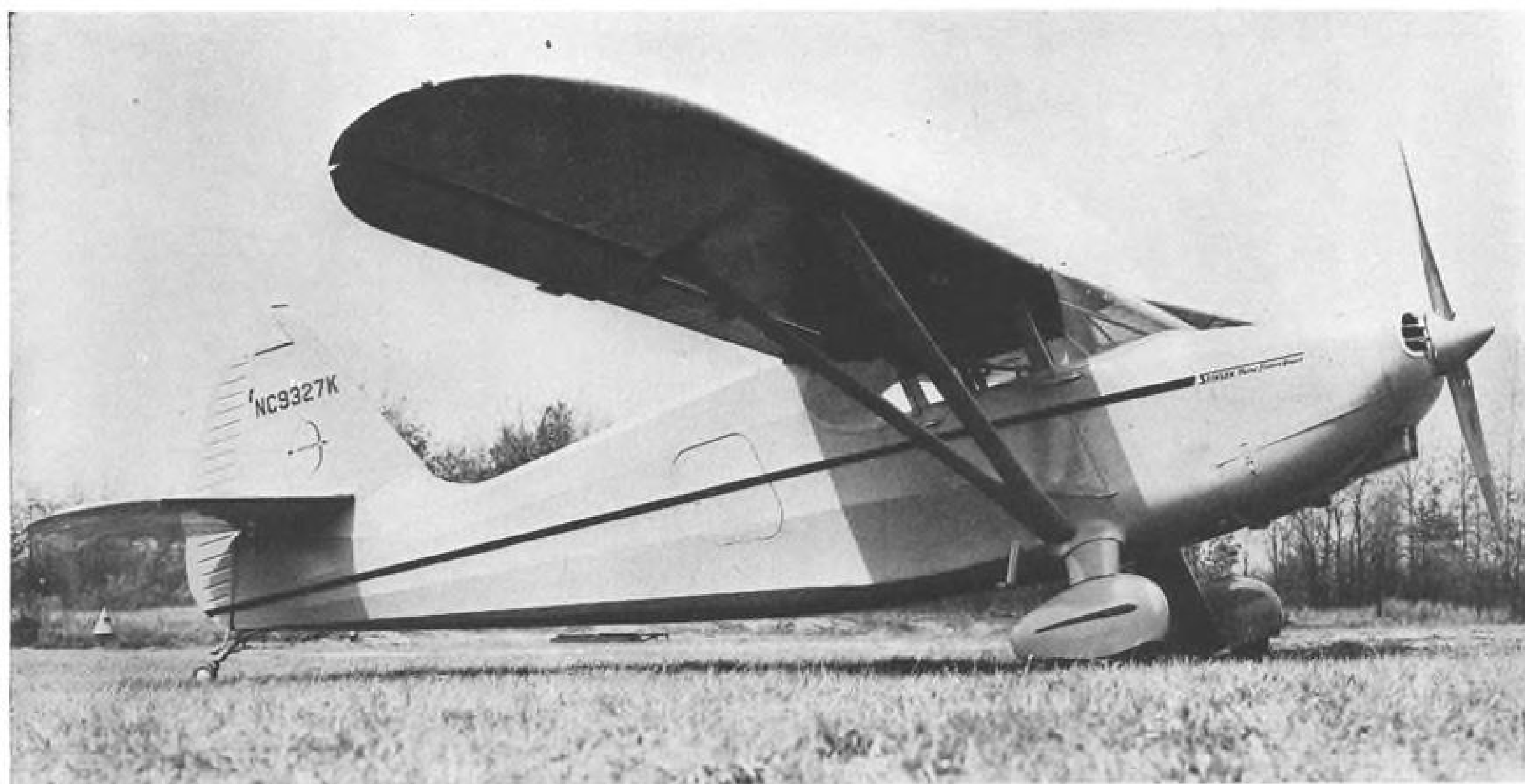
OLD: 1947 Station Wagon Stinson has lower vertical stabilizer and no adjustable rudder trim. The aircraft uses single fore-and-aft antenna for sending and receiving. No major changes are in sight.
