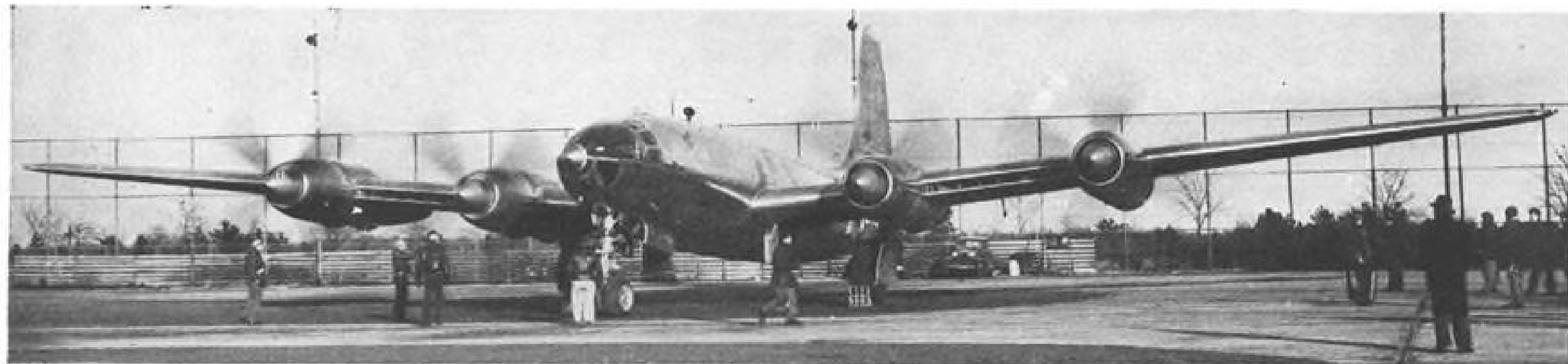
The air intakes in the leading edge of the wing created problems that were solved in a specially-constructed wind tunnel.
