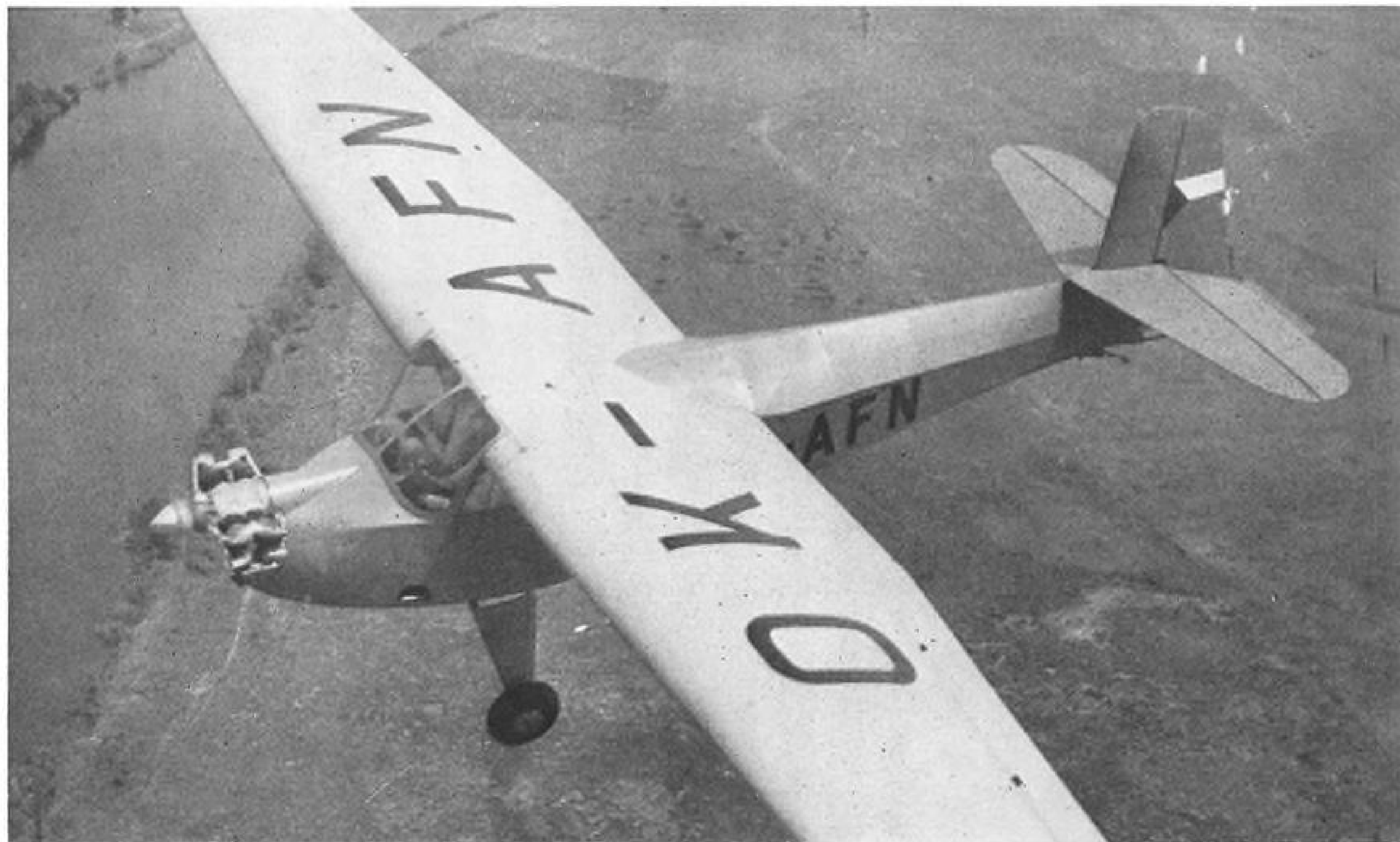
Praga Air Baby, powered by either PRAGA D 75 bhp. or WALTER MIKRON 65 bhp., is shown in actual flight.
