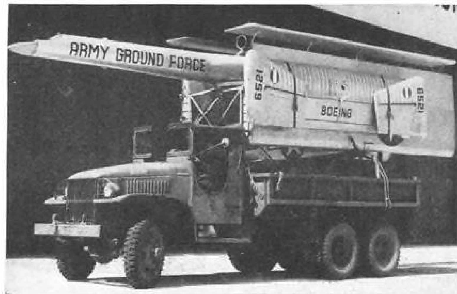
The Boeing XL-15 fits any standard 2 1/2-ton Army truck. Wings and tail section are removed, wheels rotated inboard.
