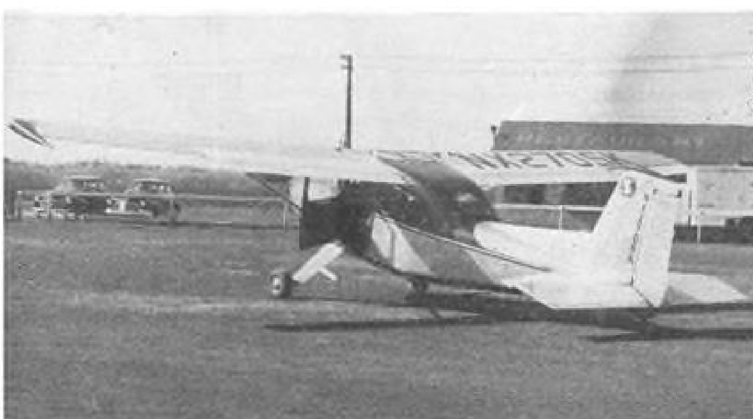
Side views show the odd fairing structure at the empennage. Note the placement of the rear cabin window and the decided down sweep of the after cabin wall, and large top windows.
