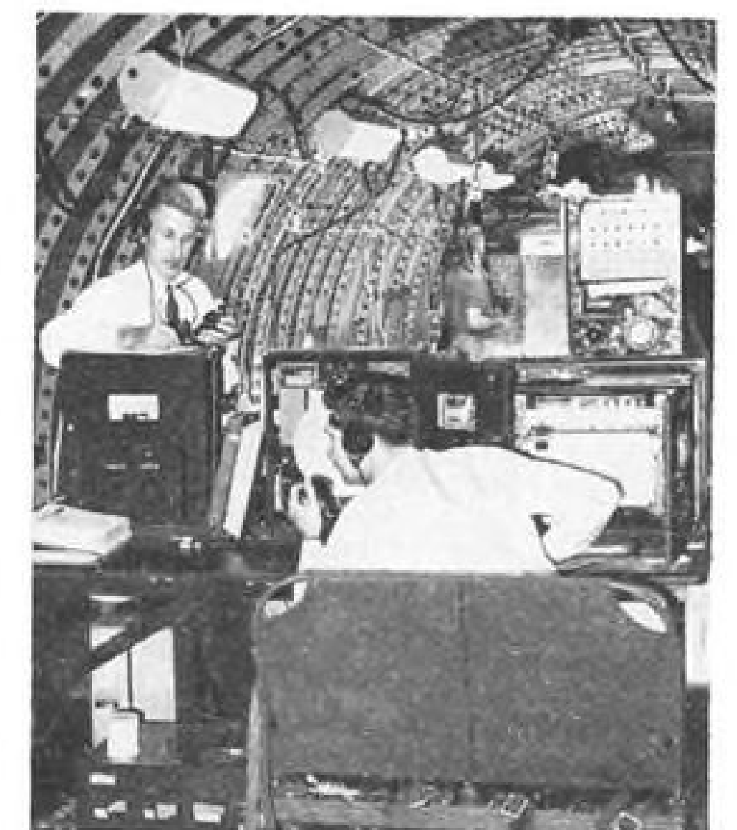
Instead of luxurious passenger accommodations, the roomy interiors of Stratocruisers being tested are filled with batteries of instruments. Literally they are flying laboratories. Thousands of vital instrument readings are recorded on every flight.
