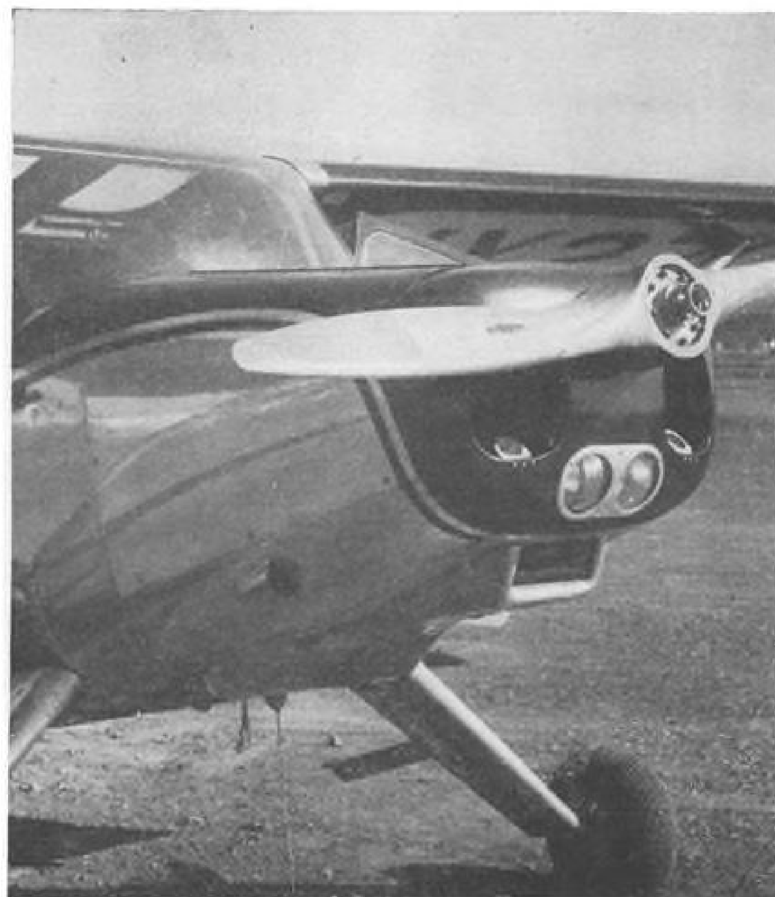
Section of nose cowl clearly shows the unusual placement of the twin landing lights. Intakes for cabin heater air are located just inside the opening of the cowl. (All photos Aviation Week)
