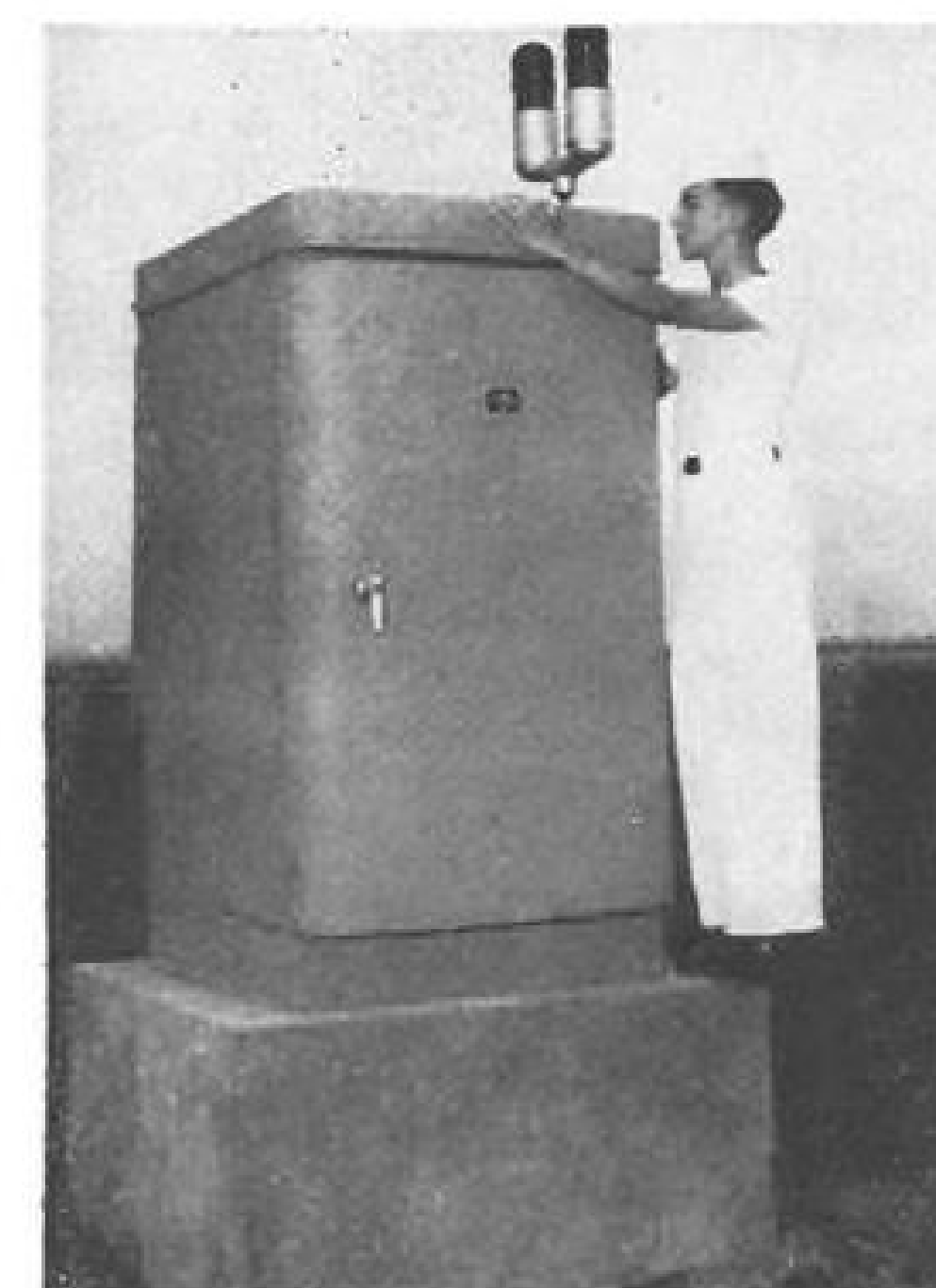
CEILING TRANSMITTER: Light source which projects pulsating beam vertically to cloud base on instrument being tested by Navy. (U. S. Navy photo)
