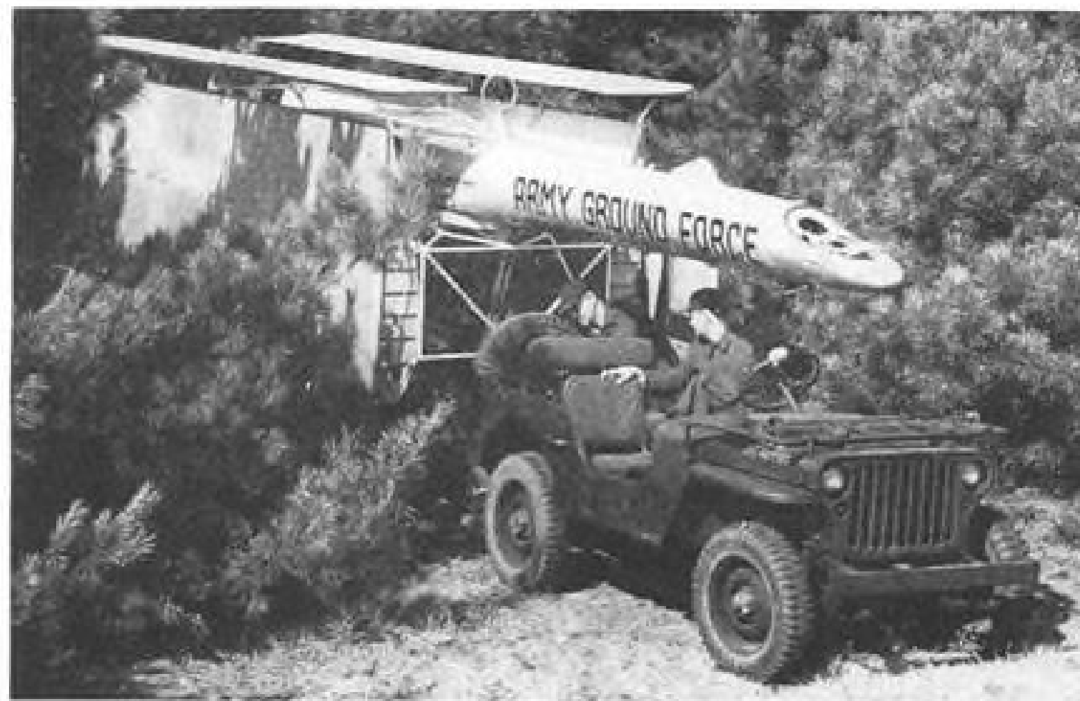
With wings disassembled and latched to the sides, the plane is towed by a jeep and tucked out of sight in the forest.
