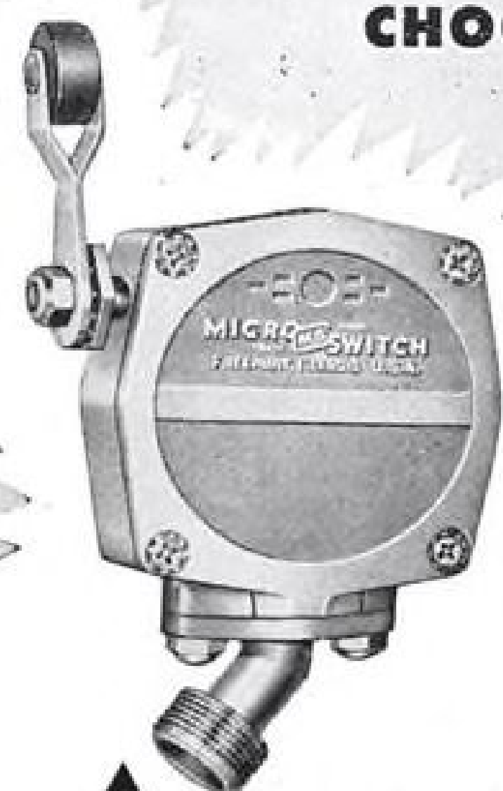
MICRO LMR Aircraft Switch has sturdy die cast aluminum housing. Mounting holes make possible four position mounting on either face. Rotary lever arm actuator is adjustable through 360 degrees. Total travel of roller arm is 90° in either direction.
