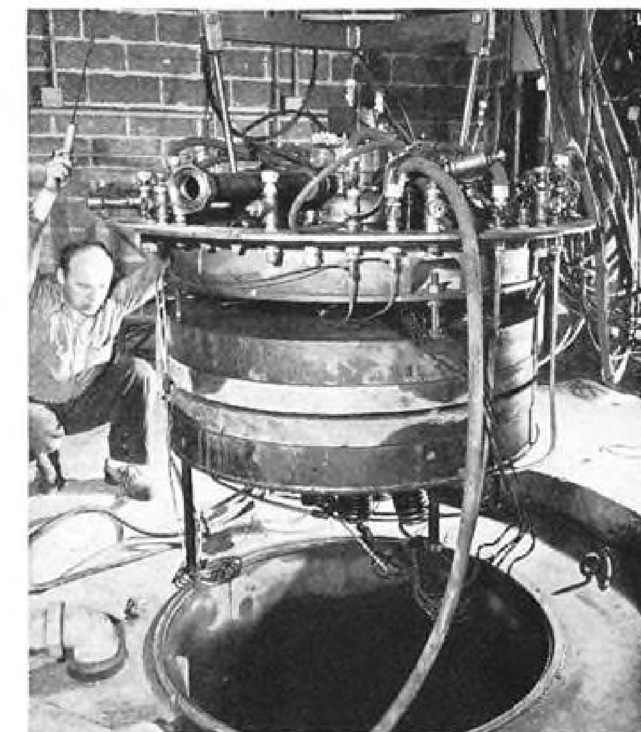
HOT-SPIN TEST PIT evaluates high-temperature properties of disk and blade alloys. Full instrumentation records results. Pit is heavily armored for destruction tests.
