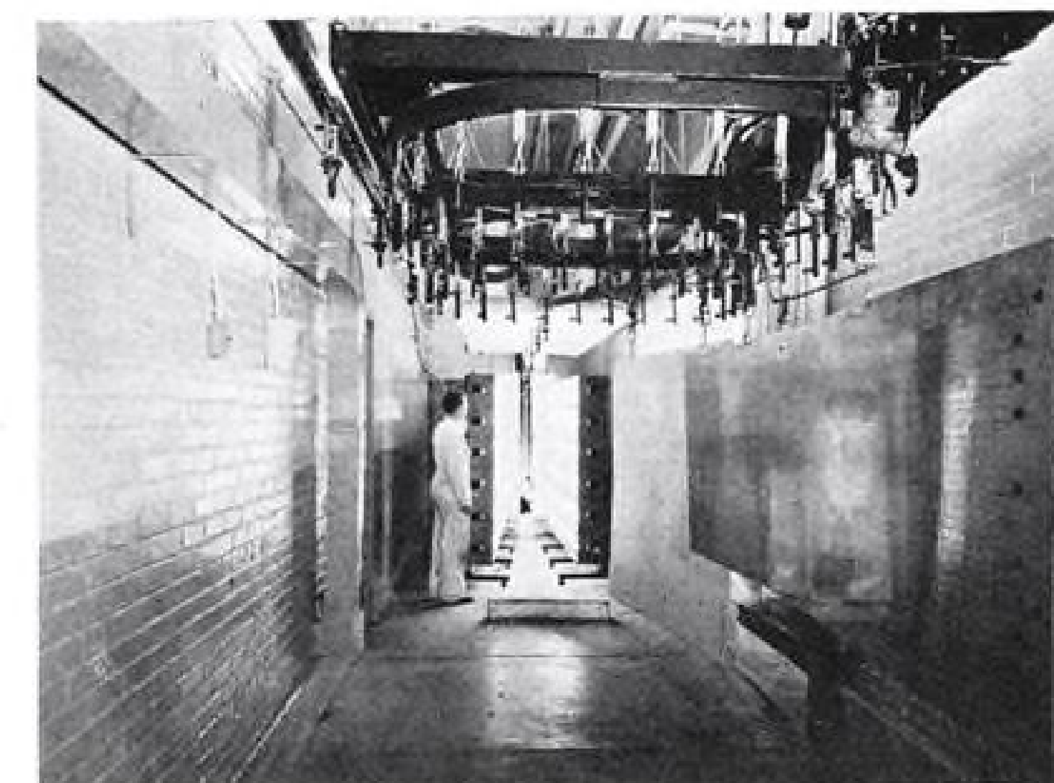
Two banks of infra-red lamps dry photo templates as they are carried by on conveyor to final inspection area. Sheet at the right is being transferred automatically to overhead turntable.
