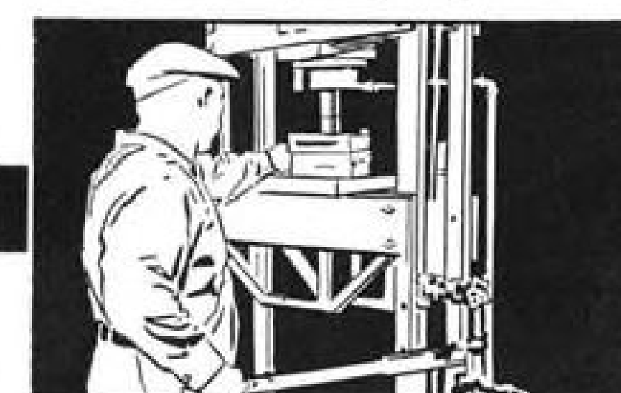
Blanking is easy with simple die set for short-run operations. Releases regular equipment for quantity production.
