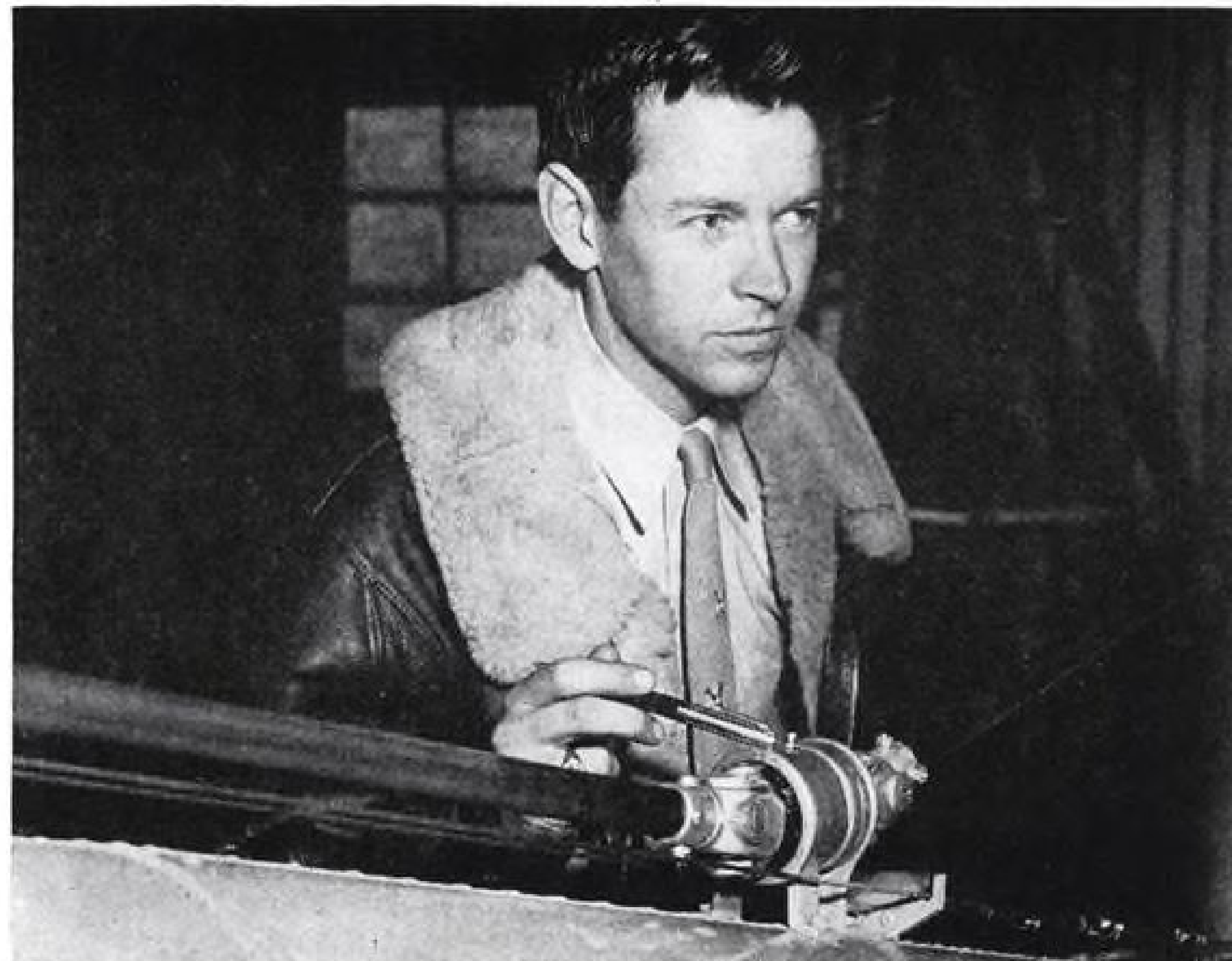
Low cost universal joint, rather than gear assembly, is used to carry power to tail rotor drive shaft of Hiller "360". Mounting is inexpensive aluminum casting. Langhorne Washburn, United Helicopters operations manager, points to assembly.
