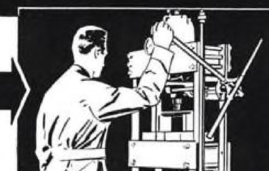
KRW Built-in Mechanical Press permits up to 3 tons pressure for straightening small diameter work.
