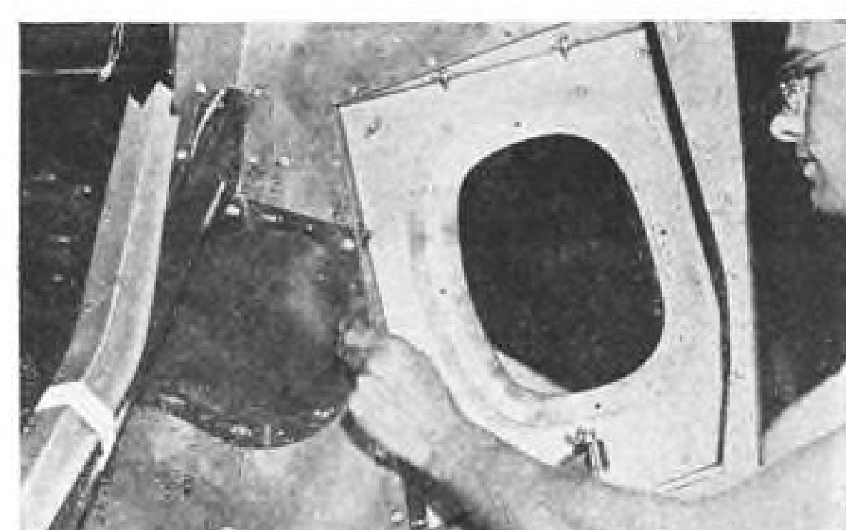
J-M No. 95 Neoprene-Asbestos Sheet Packing installation in fire wall of B-36 nacelle.
