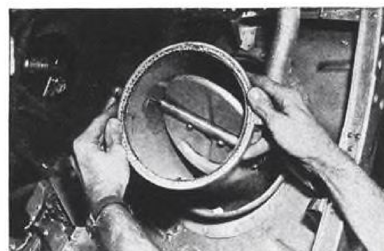
Inconel Packing installation in slip joint just aft of heat exchanger in B-36.
