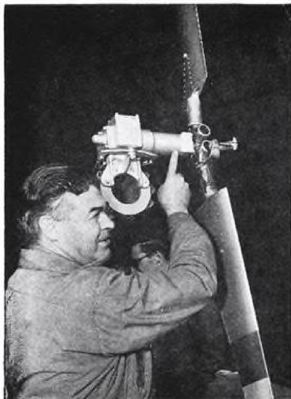
Magnesium casting indicated by Otto Sant-off, shop superintendent, holds tail rotor gears and shaft and cuts costs by requiring only inside finishing. Beaded skin of tail boom gives structural rigidity and eliminates expensive inner frame. Metal tail rotor blades are Hiller design.
