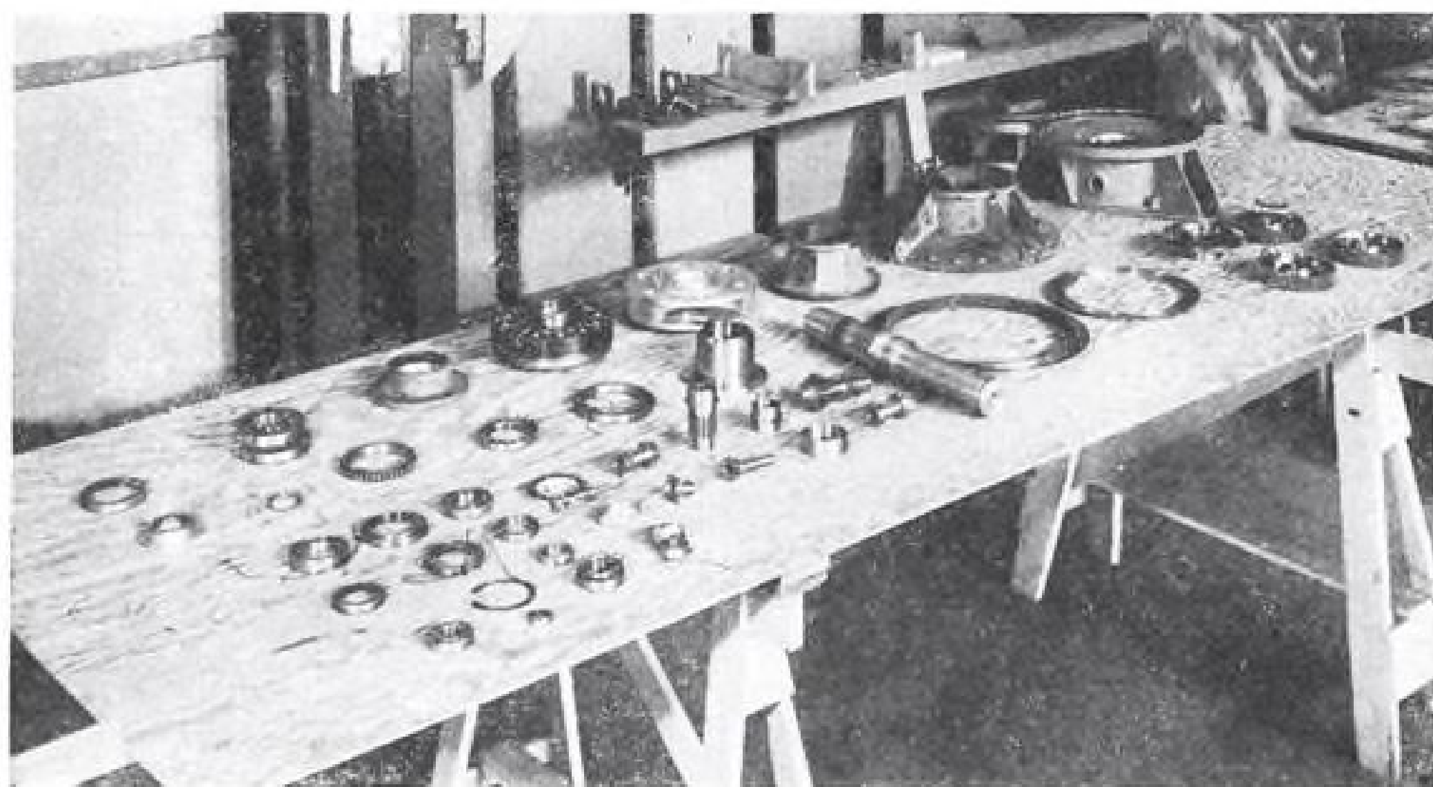
Layout of parts of simplified transmission of Hiller 360 single planetary gear assembly.
