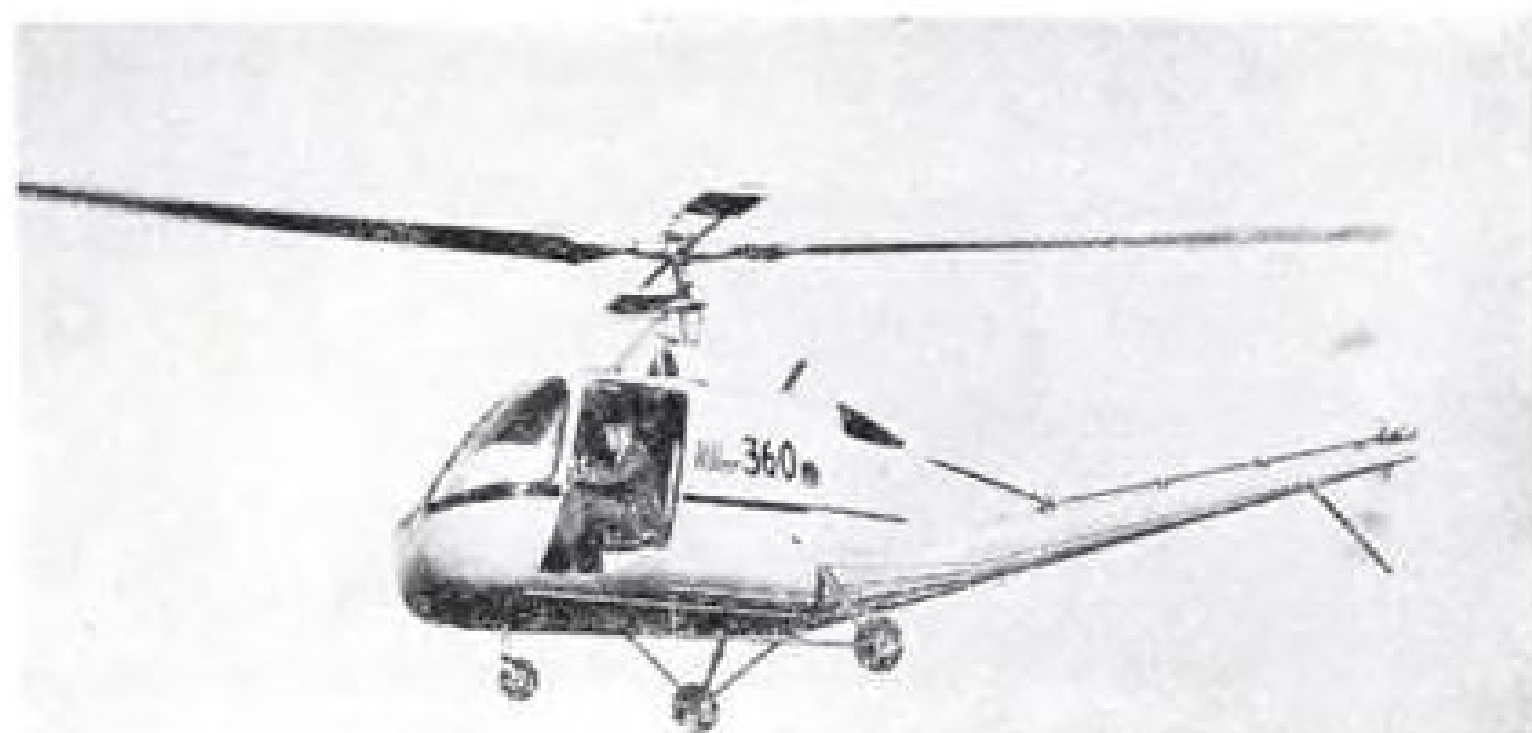
Test flight on third day out of shop shows configuration simplicity of United Helicopters, Inc. production model. Pilot and two passengers sit abreast in wide cabin. Aviation Week's Pacific Coast editor is studying instrument panel. Manufactured units will have doors in place and fairing over tail rotor drive shaft.
