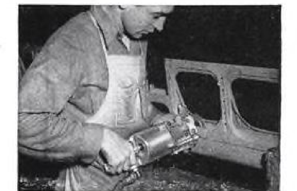
CP-214 Pneumatic Compression Riveter is especially suited for fast work in close quarters . . . its strong "squeeze" action insures exceptionally accurate and uniform results.
