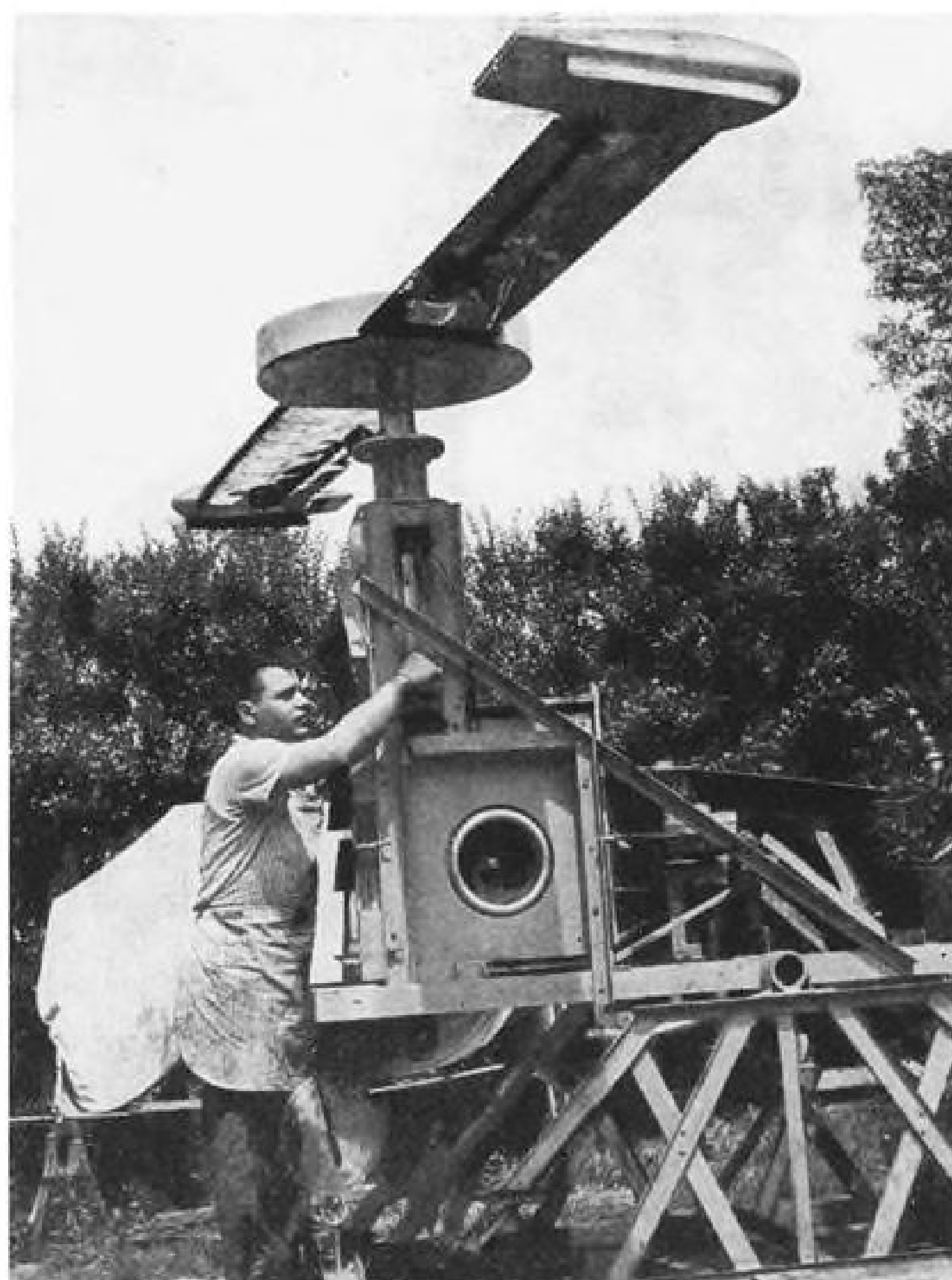
Early experimental Carlat leading-edge-jet rotor with lobes for elimination of tip vortex. Rotor is ducted to blower.
