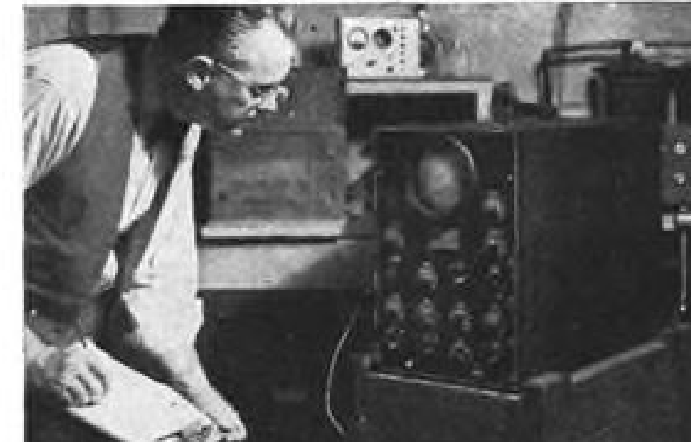
Janitrol engineers can visibly analyze on the screen of an oscillograph, the electrical characteristics of heater control devices.
