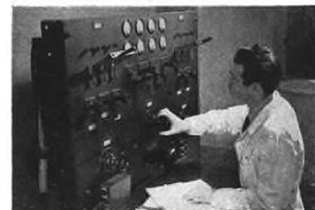
Thorough testing and inspection of heater ready for shipment on specially built Janitrol motor-generator testing machine.
