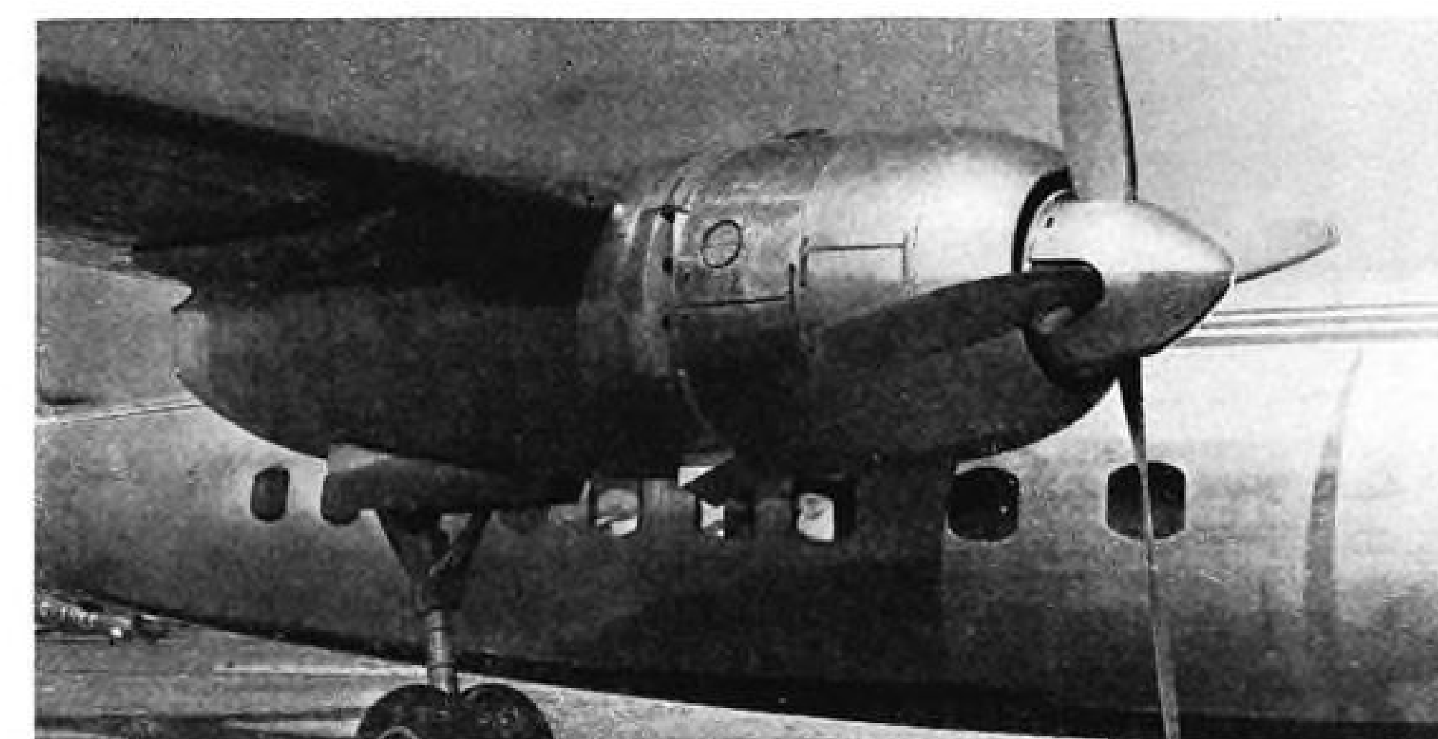
Photo shows excellent visibility provided by high wing design. Note that engine nacelle has only one protuberance extending into the slip stream. Cowl flaps and oil cooler shutters operate internally and are thermostatically controlled with a manual over-ride for emergency operation. Power-egg installation facilitates quick engine change.
