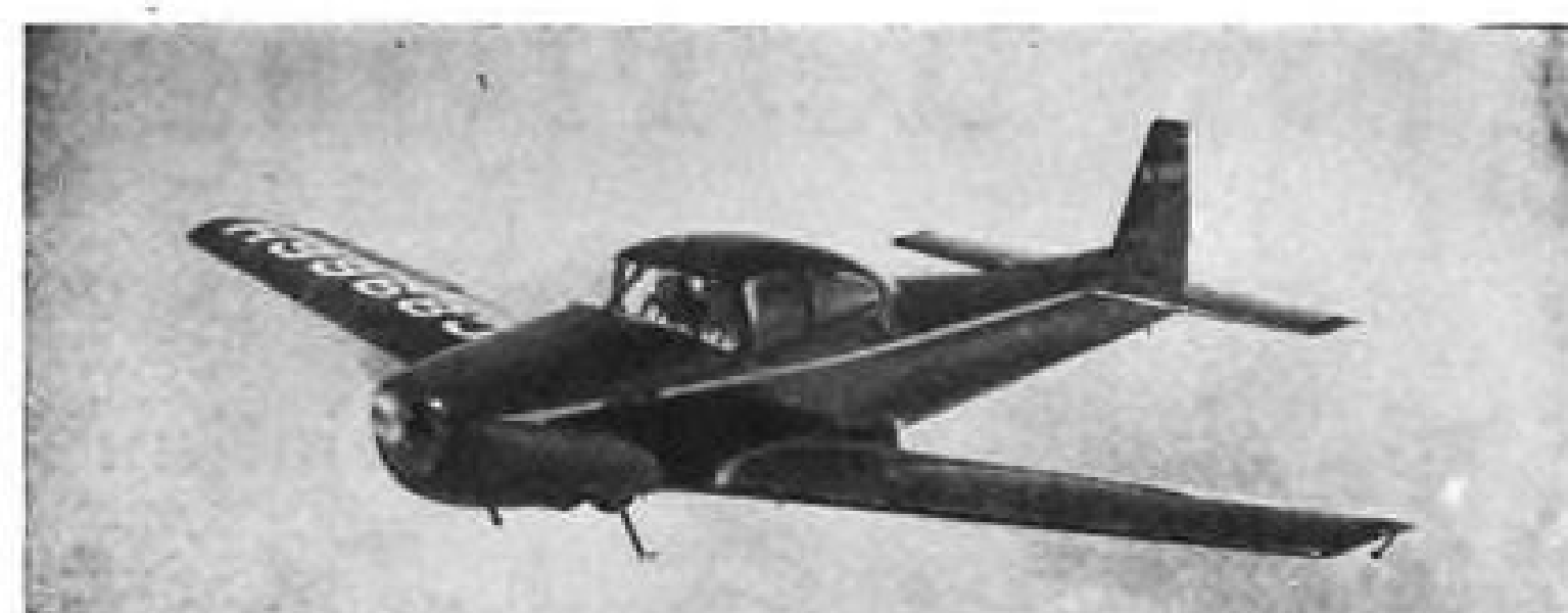
RYAN NAVION has seating capacity of four and climbs 830 fpm. Stalling speed is 54 mph. and fuel capacity 39½ gal. Propeller is made by Hartzell.
