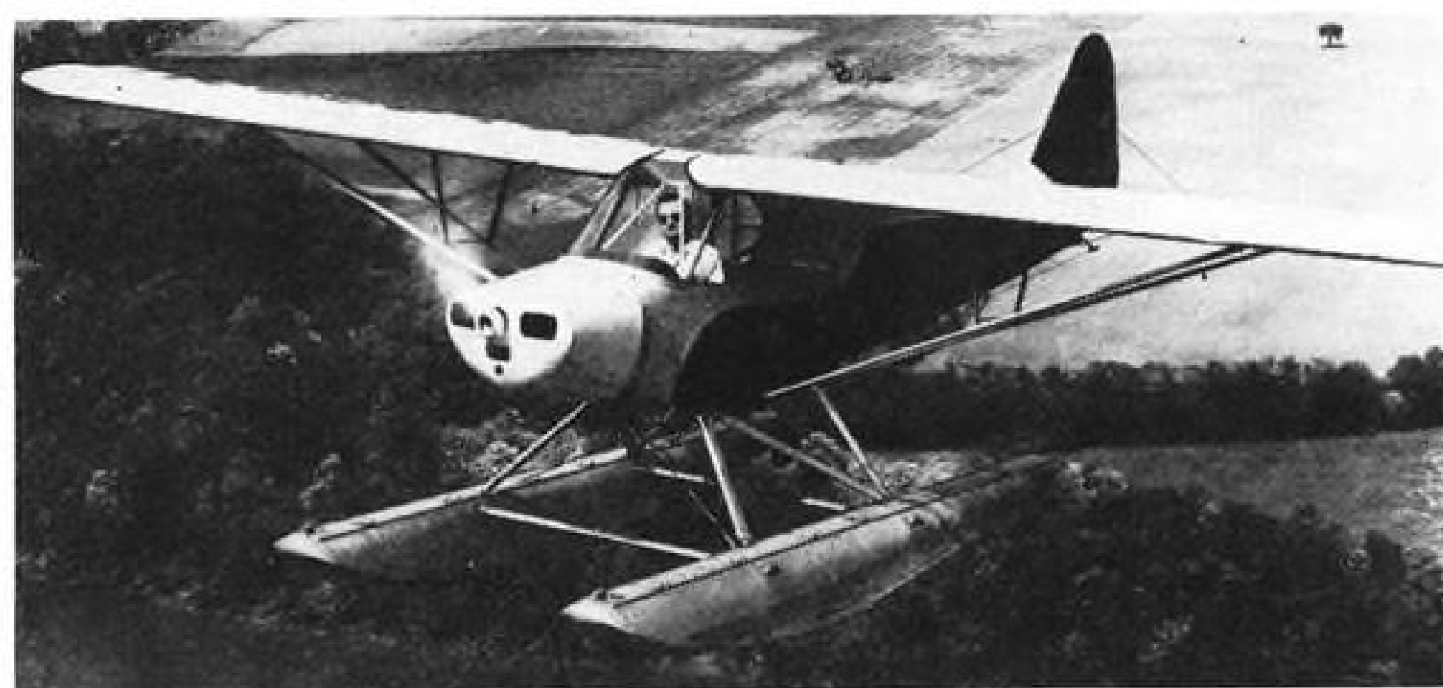
PIPER CUB SPECIAL MODEL PA-11 is two-placer. Rate of climb is 514 fpm. Has fuel capacity of 17 gal.
