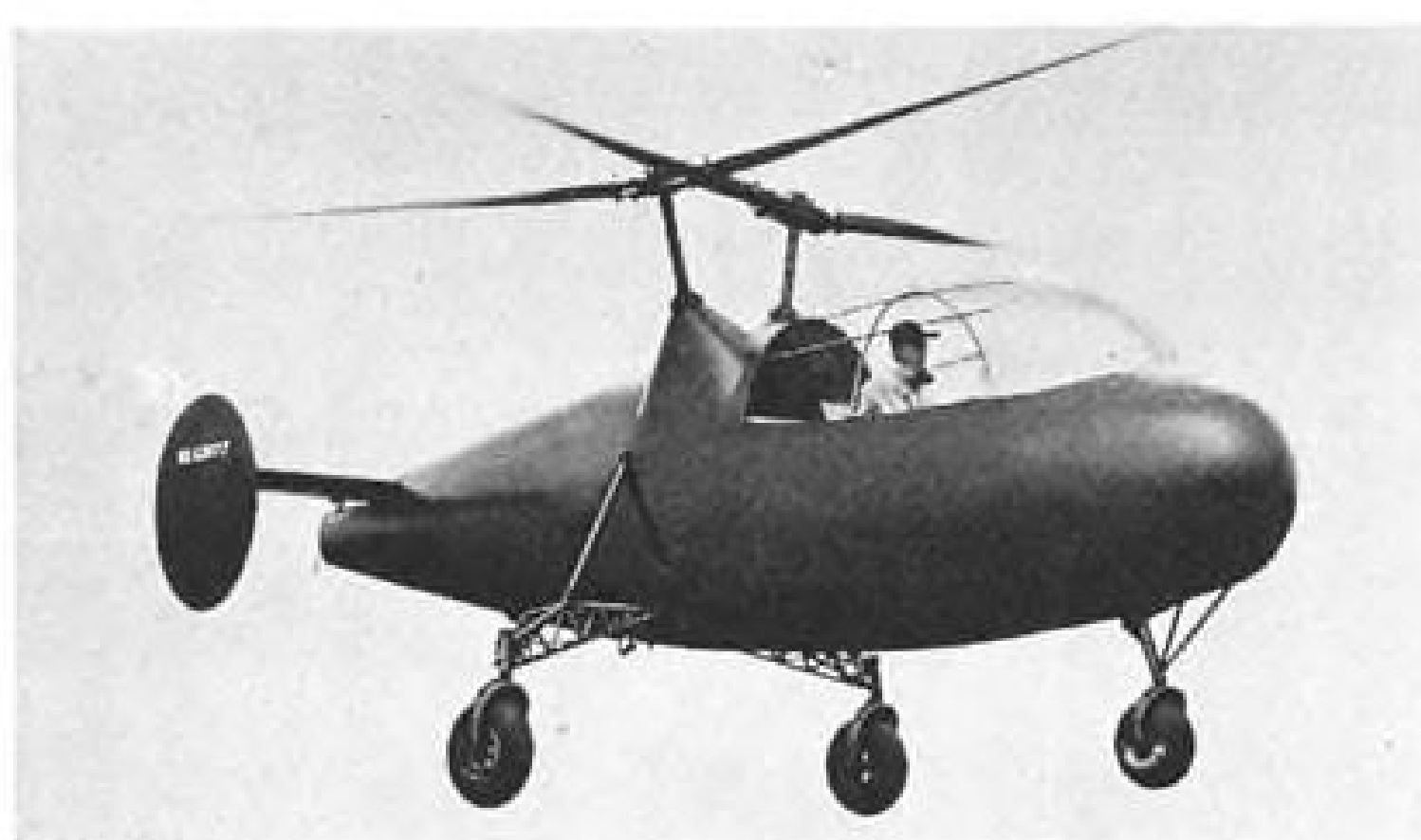
KAMAN K-125-A was designed as an engineering test stand for the development of their rotor systems.
