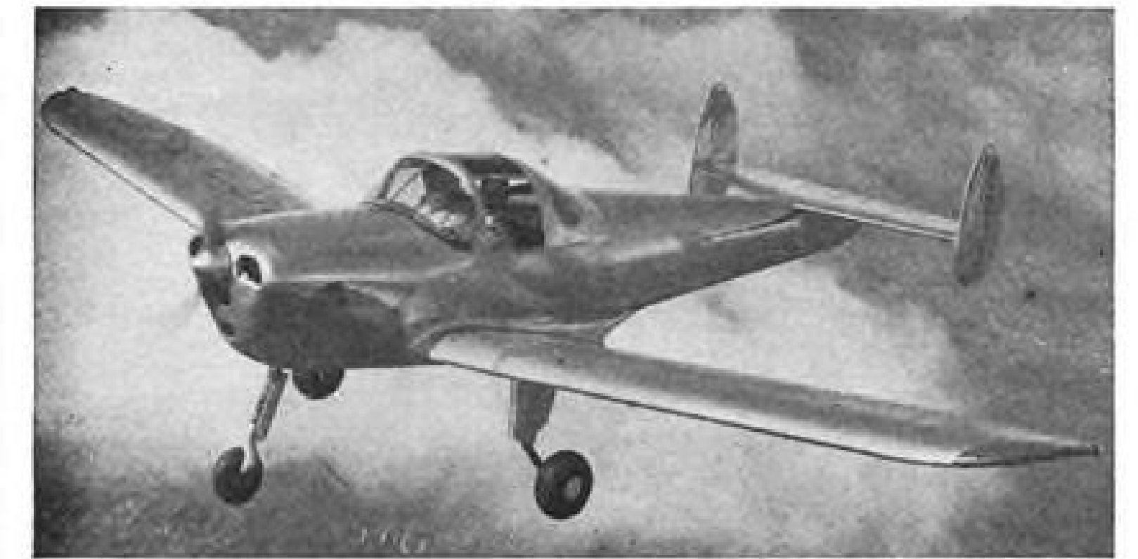
ERCOUPE MODEL E and F, two-place, climbs 560 fpm. Fuel capacity is 23 gal. Equipped with McCauley 1-A-90 or Sensenich Model 74FKT-48 propeller.
