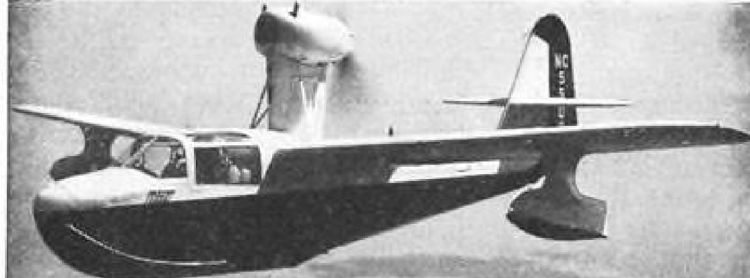
GOODYEAR AMPHIBIAN MODEL GA-2, three-place, climbs 650 fpm. Stalling speed is 56 mph., and fuel capacity 30 gal. Koppers "Aeromatic" propeller is used.
