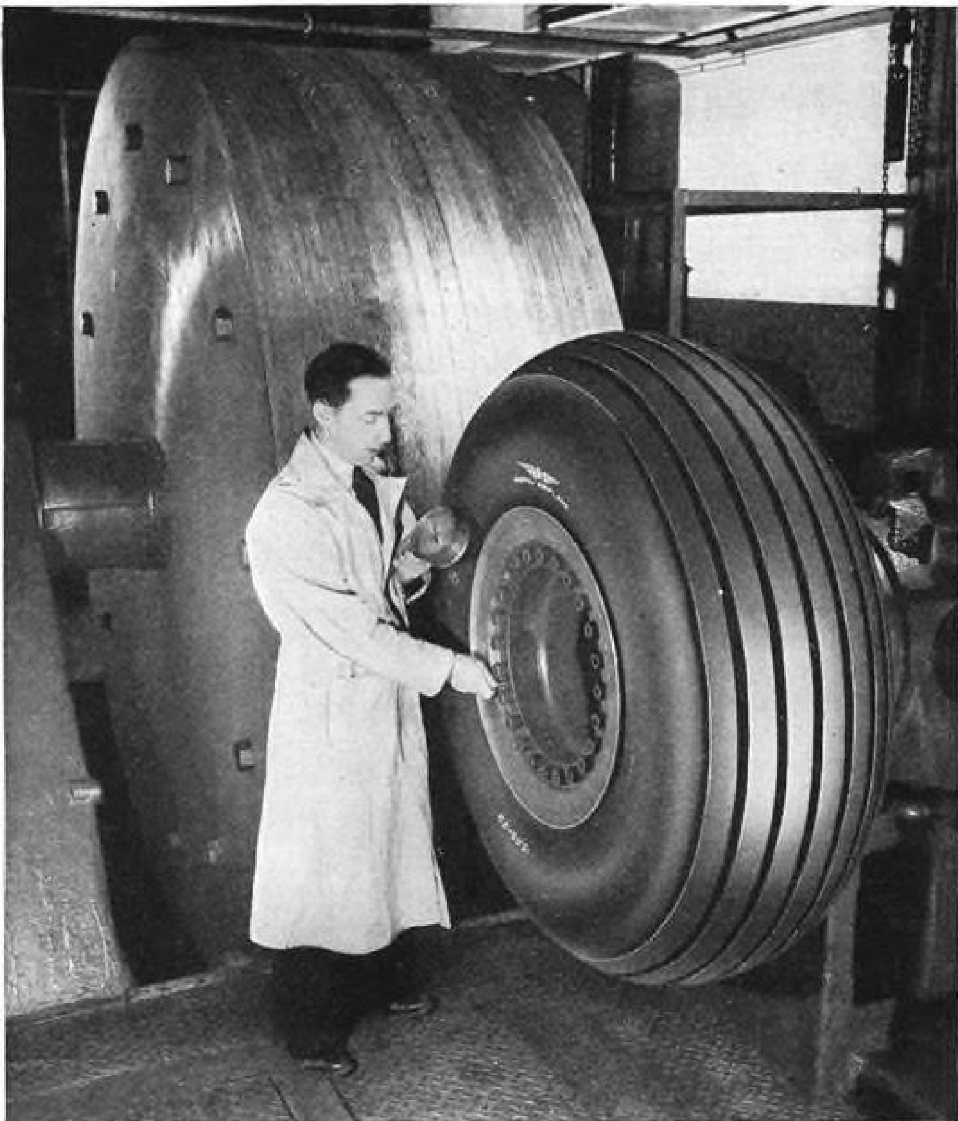
MONTHS OF THE TOUGHEST LANDING operations can be equalled in a few short hours on this giant dynamometer. It operates at up to 200 m.p.h.—duplicates loads and braking power exceeding any existing plane.
