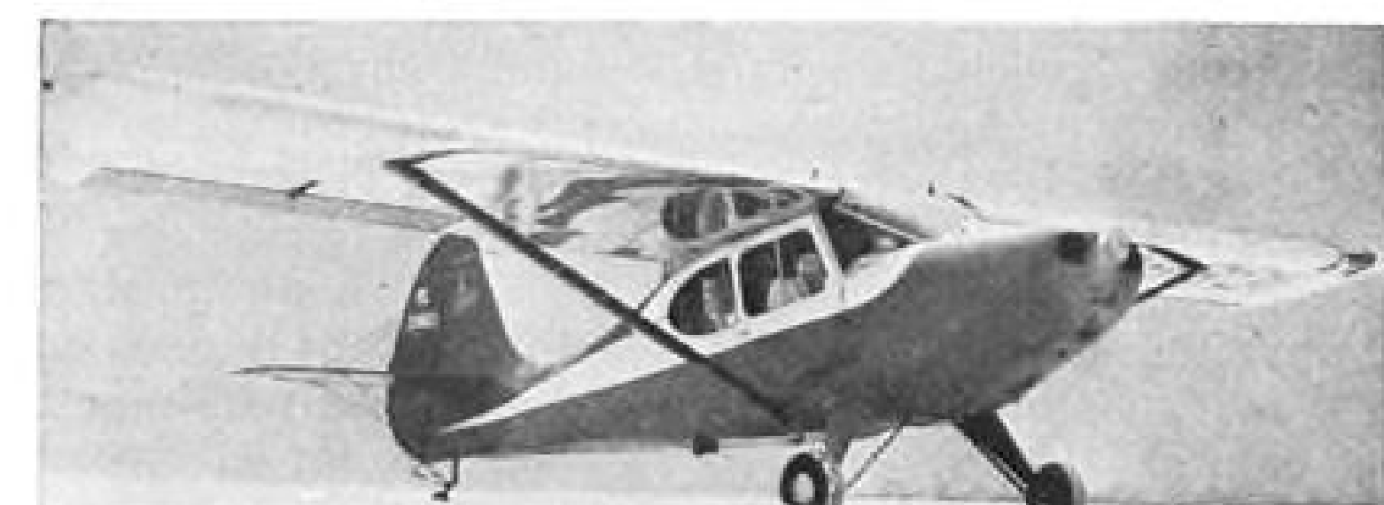
AERONCA SEDAN has a fuel capacity of 38 gal., its power-off stalling speed is 35 mph. With full load (four passengers) its sea level rate of climb is 600 fpm.
