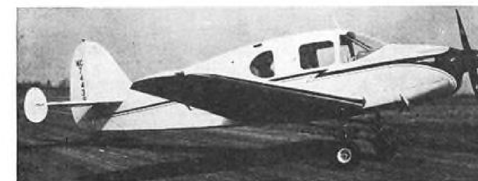
BELLANCA CRUISAIR SENIOR, four-place, climbs 800 fpm. with Sensenich propeller, 1130 fpm. with Aeromatic. Stalling speed 45 mph., fuel capacity 30 gal.
