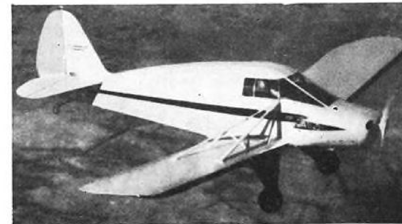
CALLAIR MODEL A-3, two-place, climbs 1,000 fpm. Stalling speed 45 mph., fuel capacity 30 gal. Propeller by Sensenich. Production in 1947 totaled 14.
