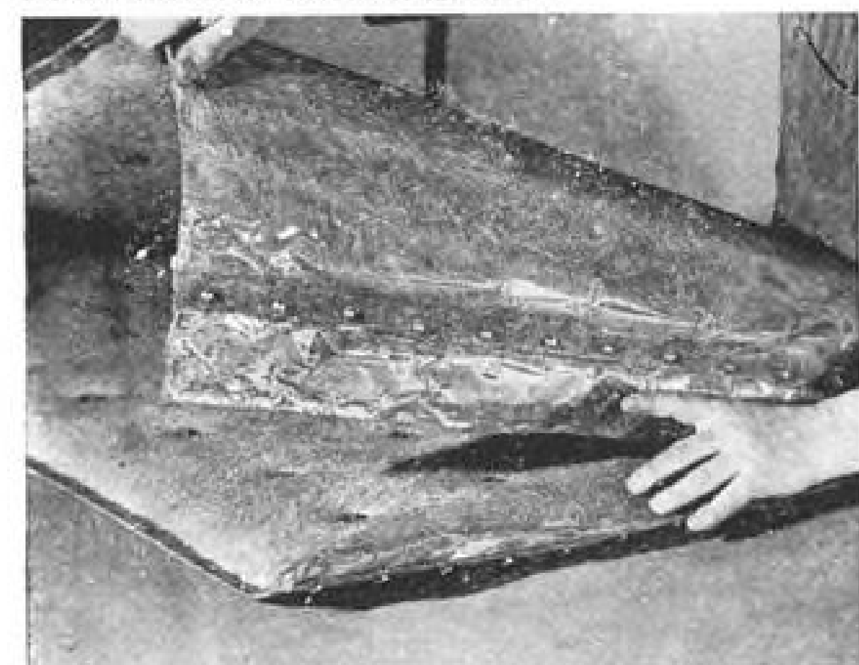
Close-up of J-M Thermoflex Insulation Blanket. Note flexibility which assures easy application.
