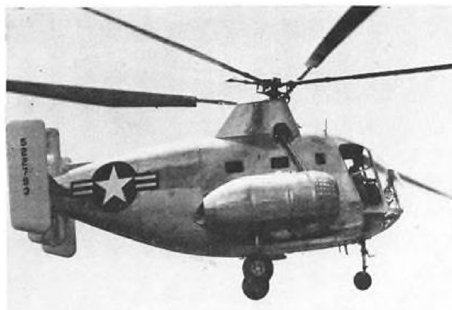
KELLETT XR-10 metal experimental model is designed for 10 plus 2 crew. Rotors are steel tube under plywood.
