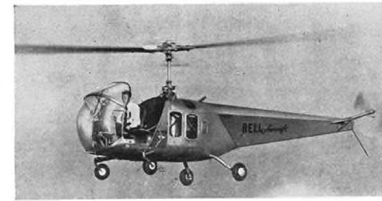
BELL 47D's steel tube construction is covered with metal and fabric. Laminated rotor is loaded at 2.21 lb./sq. ft.
