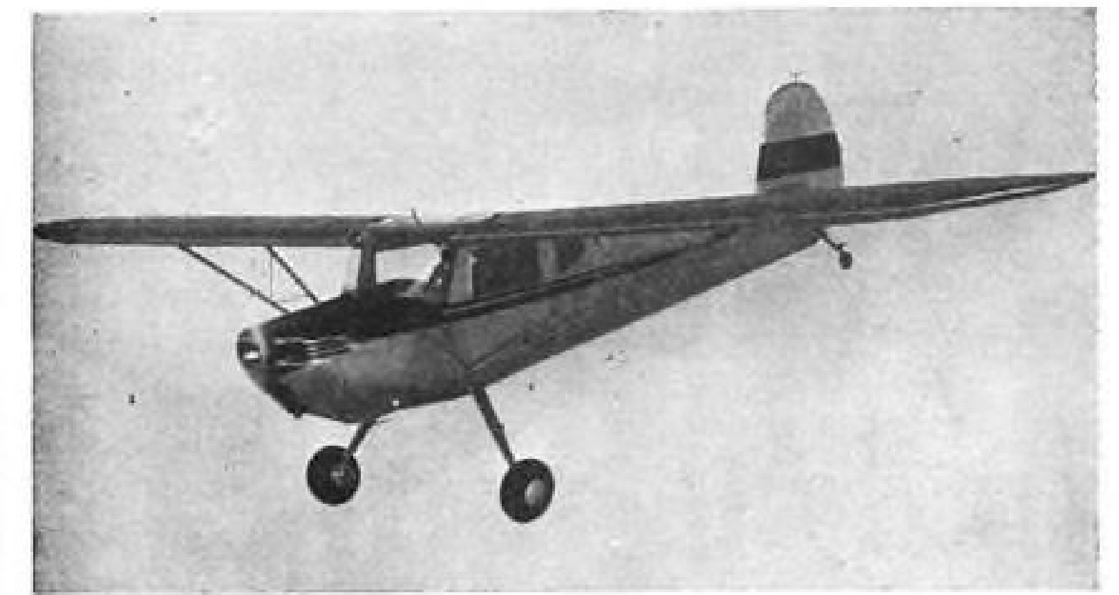
CESSNA MODEL 140, seats two. Climbs 690 fpm. Stalling speed is 41 mph. Fuel capacity is 25 gal. Sensenich propeller is used. (Ross-Pix)
