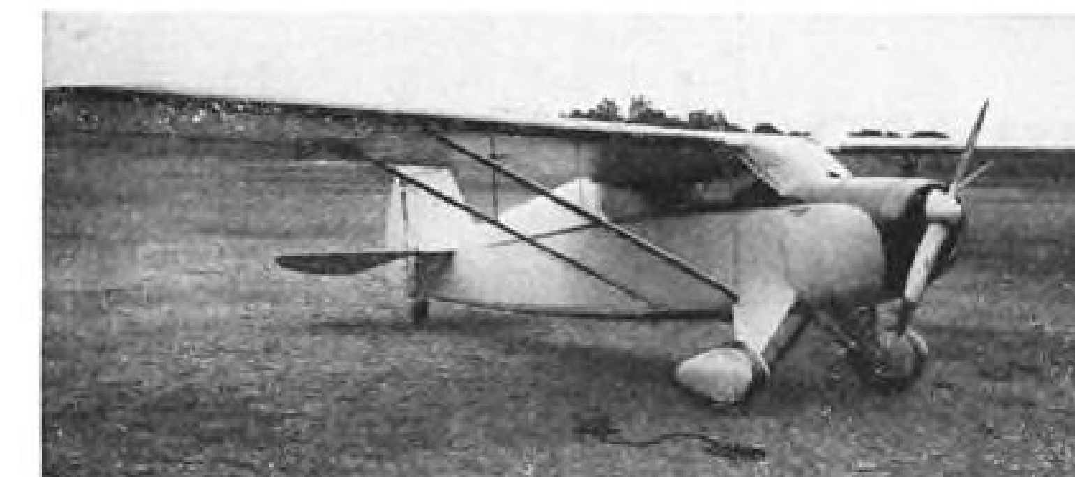
FUNK CUSTOMAIRE MODEL B85C seats two. Rate of climb is 800 fpm. Stalling speed is 37 mph. Fuel capacity is 20 gal. Lewis propellers are used. Landing gear features hydraulic shock struts and tail wheel assembly. Brakes are also hydraulic (toe operated).
