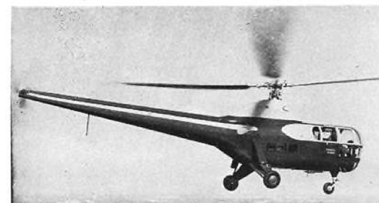
S-51 (ATC #2) four-place 'copter now in production has steel-tube covered with plywood rotors loaded at 2.76 lb.
