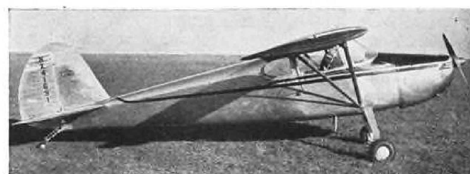
CESSNA MODEL 170 is four-place personal plane. Climbs 700 fpm. Stalling speed is 50 mph. Fuel capacity is 37.5 gal. Propeller is manufactured by Sensenich.
