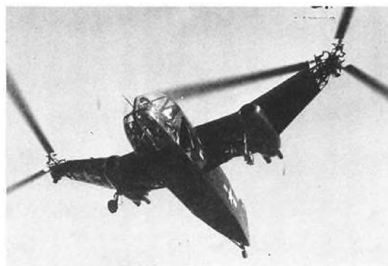
McDONNELL XHJH-1 showing engine and rotor mountings. Small wheeled landing gear is unusual.
