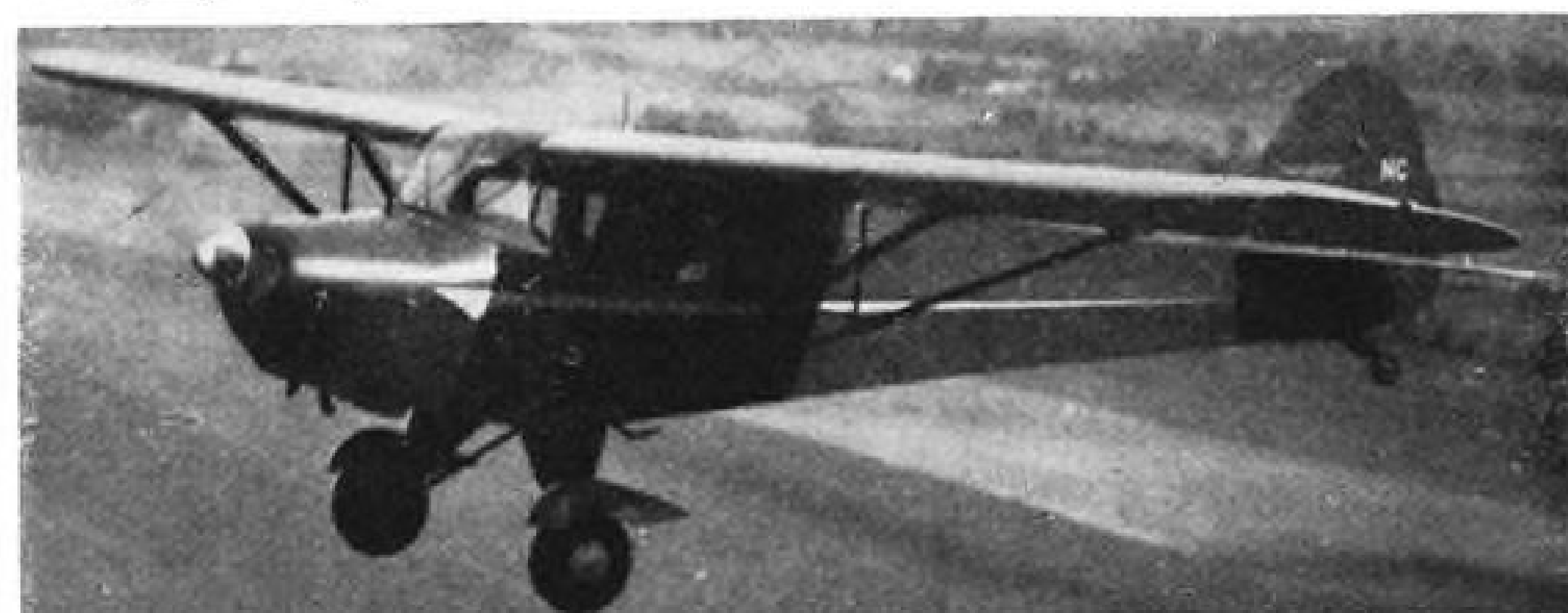
TAYLORCRAFT MODEL 47, two-place, climbs 550 fpm. Stalling speed is 38 mph., fuel capacity 18 gal. Propeller manufactured by Lewis.
