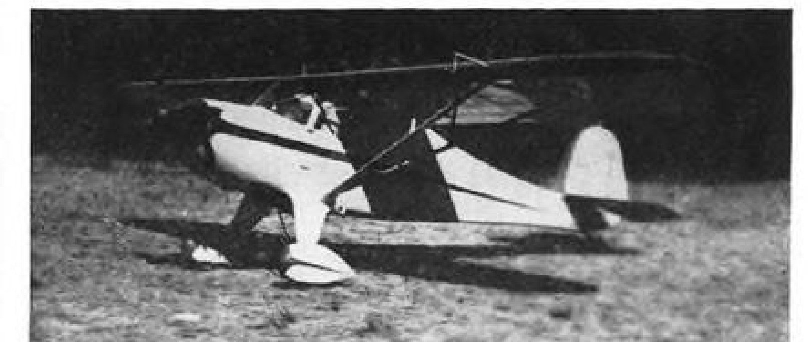
MONOCOUPÉ MODEL 90AF-115, two-place, climbs 1100 fpm. Stalling speed is 45 mph., and fuel capacity 28 gal. Equipped with Sensenich 2 position hydraulic propeller. The twin-engine Model H MONOCOACH has four-to-five seating capacity.
