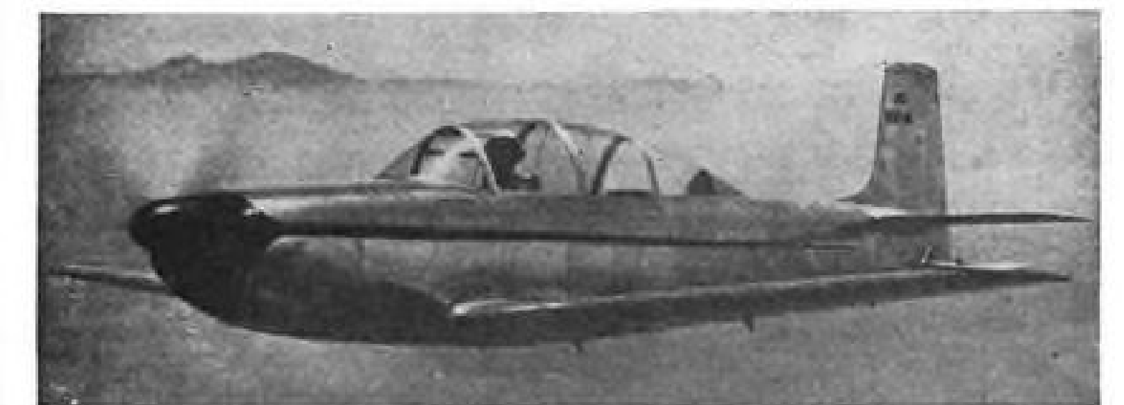
AERO-FLIGHT STREAK 85, two-place, climbs 950 fpm. Stalling speed is 52 mph. Has fuel capacity of 20 gal. Uses Sensenich propeller.
