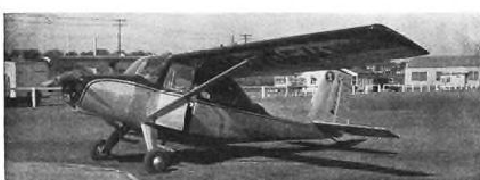
LUSCOMBE SILVAIRE SEDAN, the Dallas company's entry in the four-place field, climbs 900 fpm. Stalling speed is 58 mph., and fuel capacity is 42 gal.
