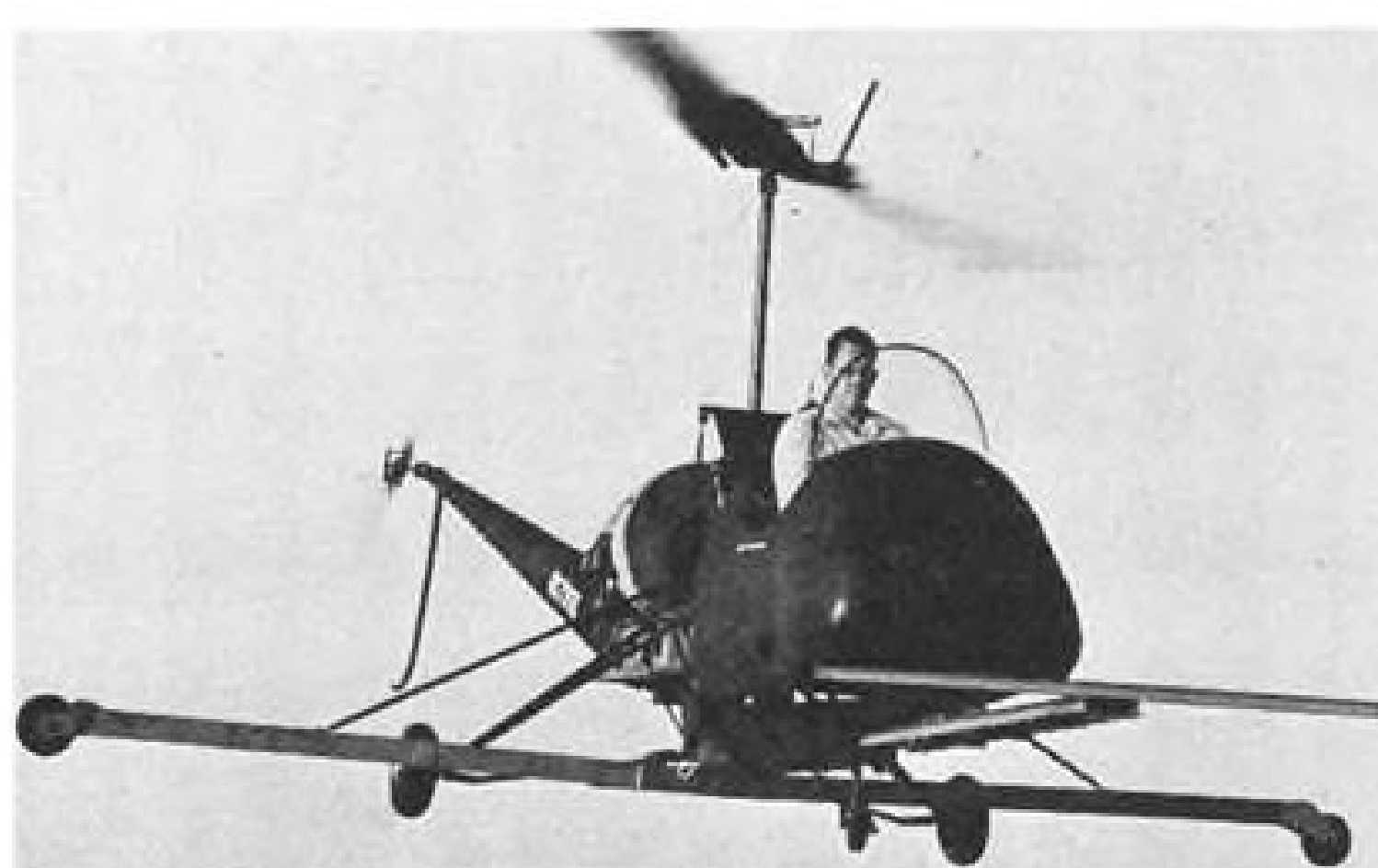
SEIBEL S-3 does not employ cyclic pitch, control is obtained by shifting center of gravity. Uses solid wood rotor.
