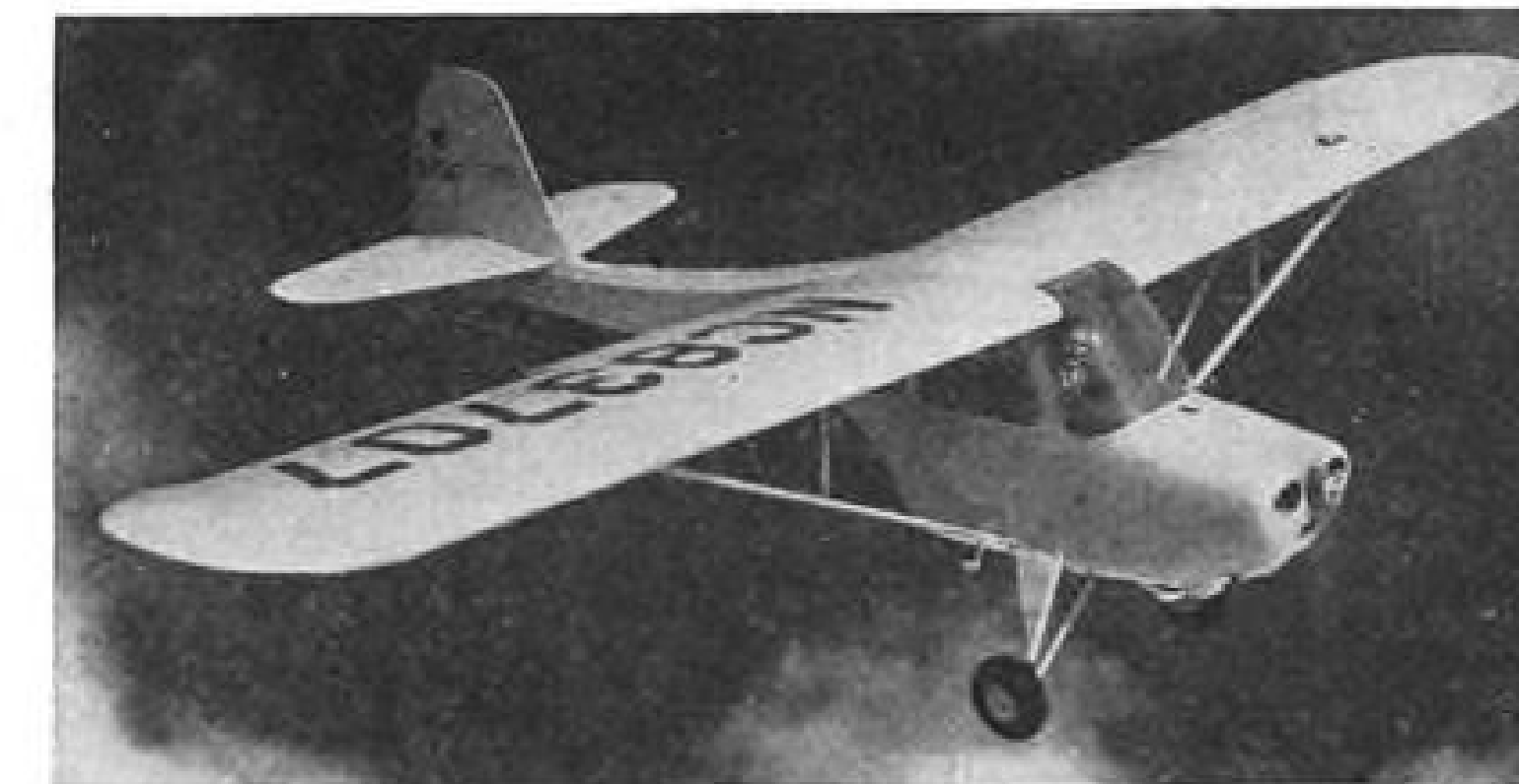
AERONCA CHAMPION MODEL 7AC, two-place, climbs 500 fpm. Stalling speed is 40 mph., and fuel capacity 13 gal. Sensenich propellers are used.
