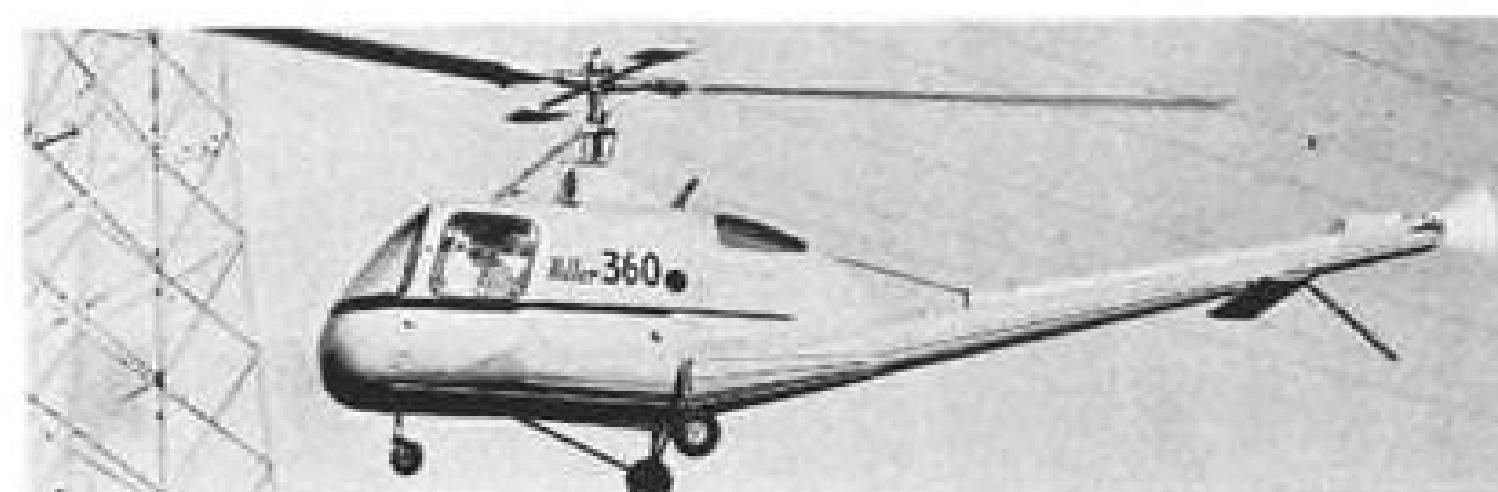
HILLER 360 features a teetering type rotor and emphasizes simpler design that is easy and cheap to reproduce.
