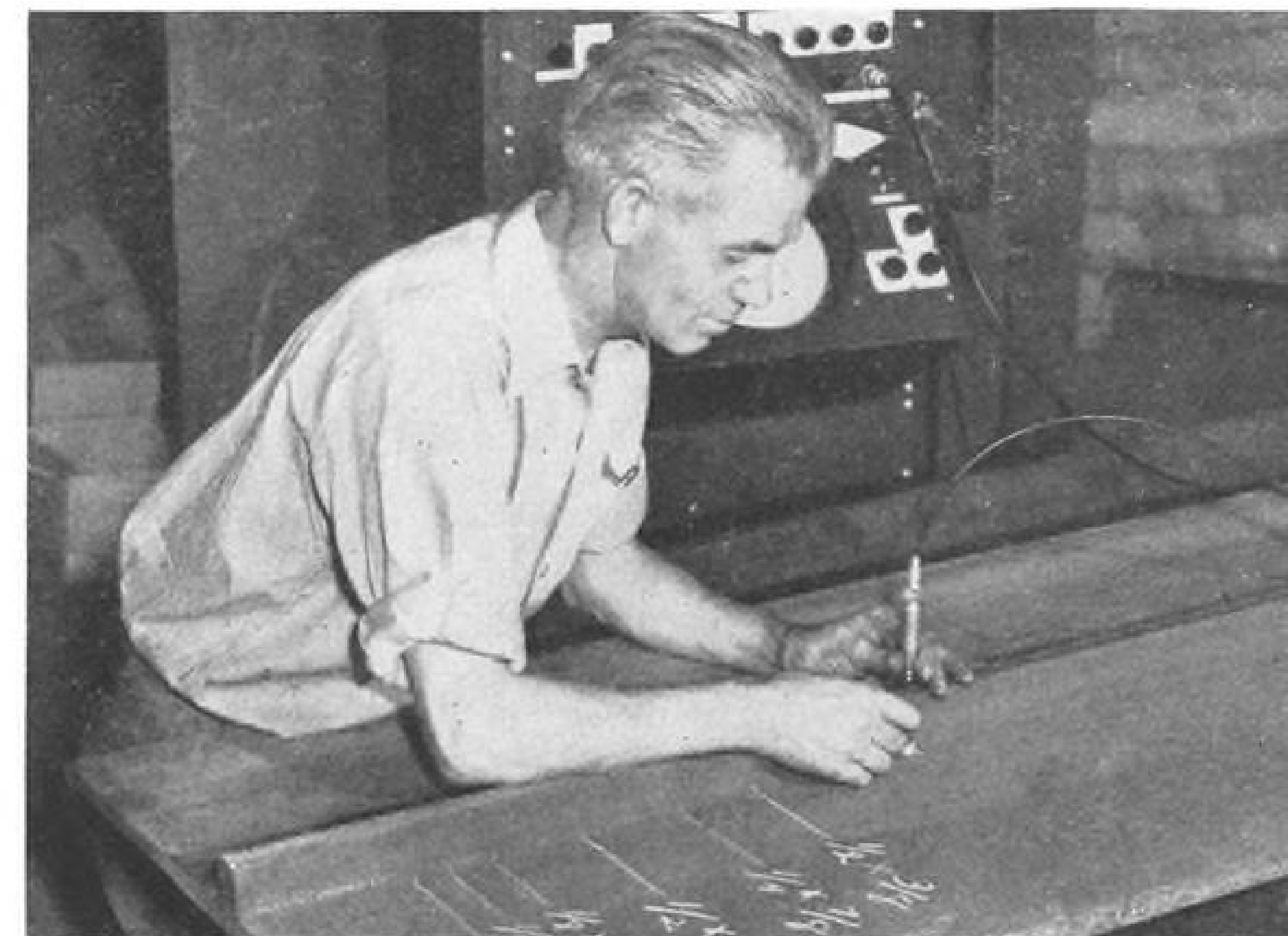
Operator moves Reflectoscope's searching unit along rib section of propeller material, and marks locations of flaws on adjacent plate surface.
