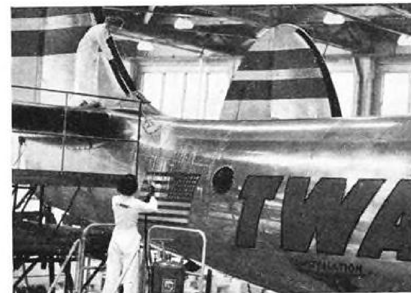
"Spray application of Turco Mulsirex and water rinse saves man-hours and materials; promotes safety by facilitating aircraft inspection and repair," says R. C. Loomis, Director TWA Maintenance & Overhaul.
