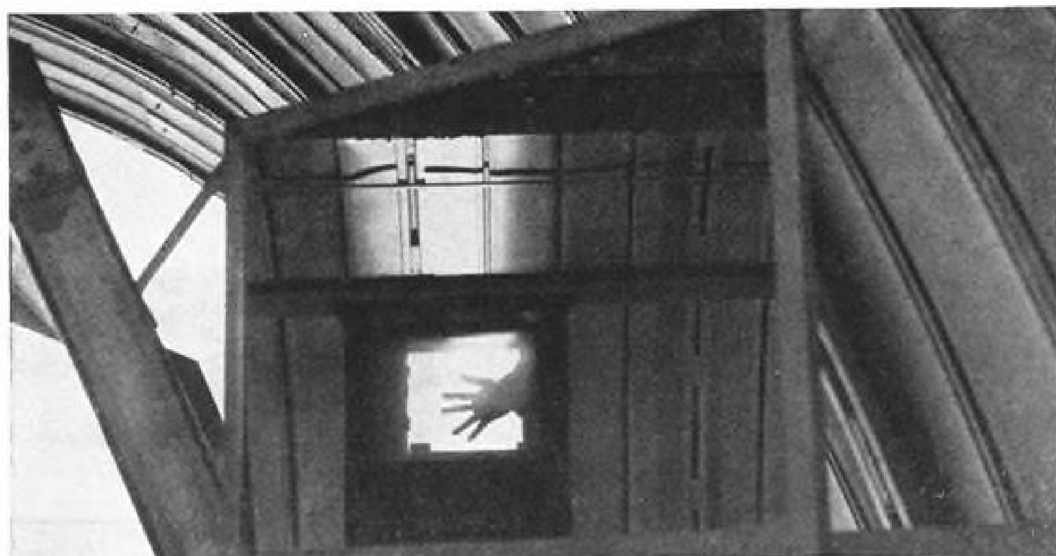
Here, hand image on mirror demonstrates how shadows of shock waves can be observed by aerodynamicist conducting ramjet study when jet stream strikes obstacle in its path.
