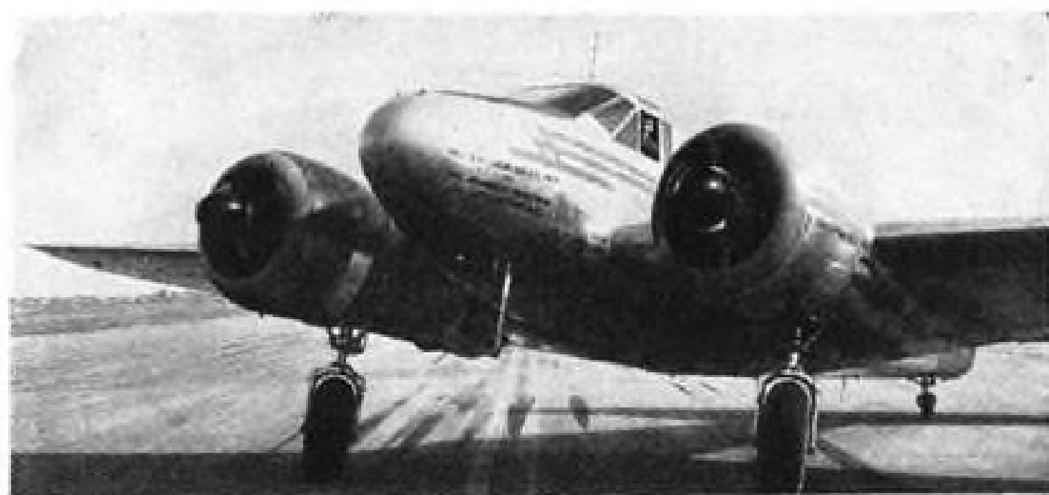
Beechcraft and DC-3 with castoring gear: it brings transports to close-in airports.
