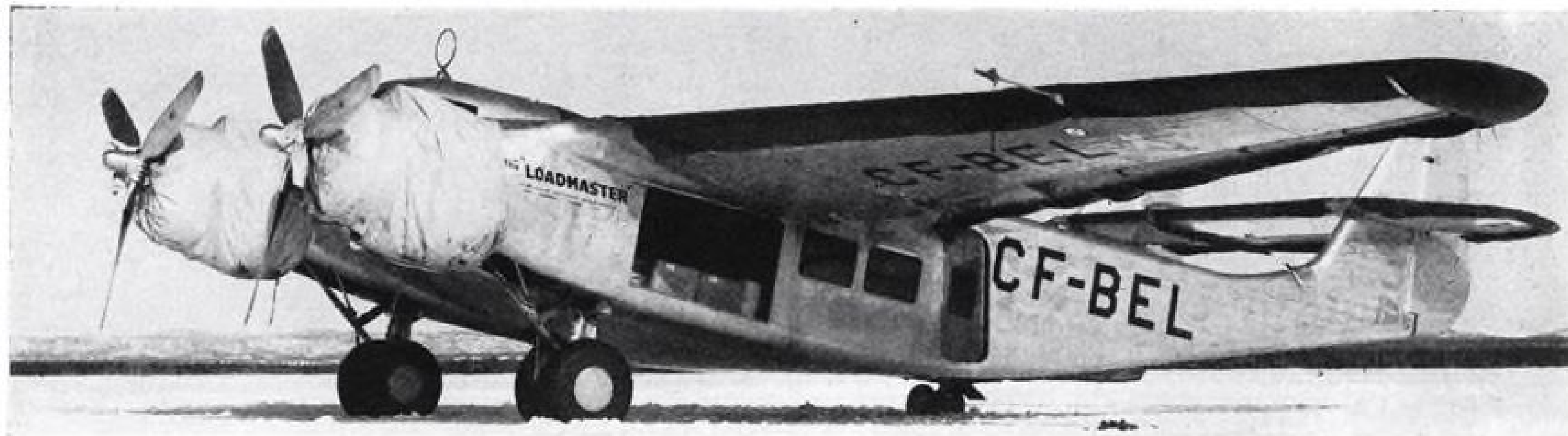
Wide side cargo access is feature of Cancargo's "flying wing" Loadmaster, designed for heavy freighting in hinterland.
