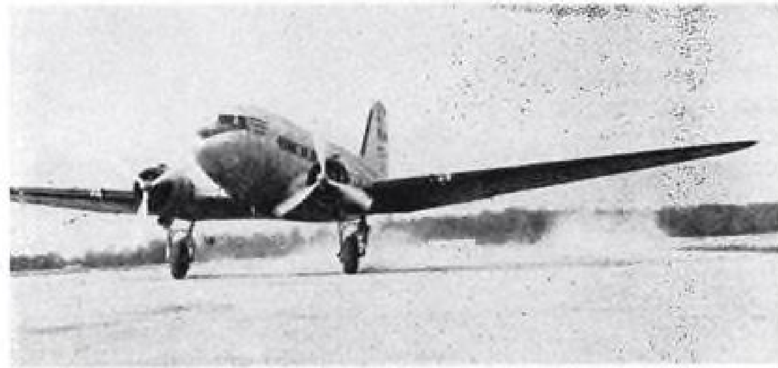
Beechcraft and DC-3 with castoring gear: it brings transports to close-in airports.
