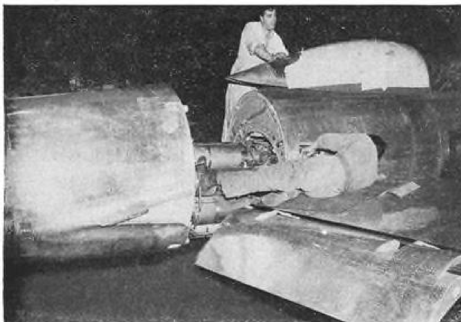
SEPARATION of fuselage exposes engine, also permits. . .
