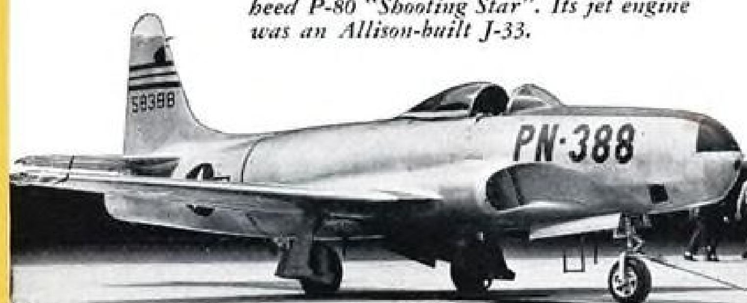
Col. Petit flew this U. S. Air Force Lockheed P-80 "Shooting Star". Its jet engine was an Allison-built J-33.
