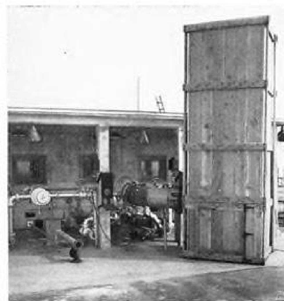
LESS EXPENSIVE method is used by AiResearch. This wooden frame sound control tower was built for less than $1000.
