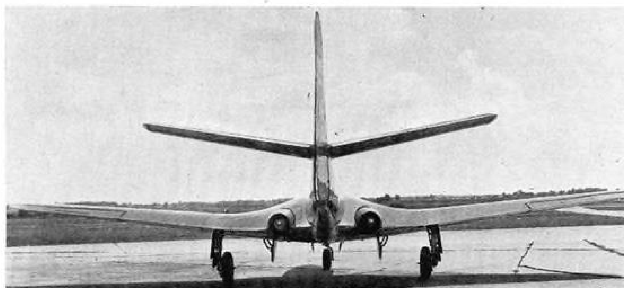
Rear view of Phantom shows close-inboard location of turbojets, affording stability with single-engine operation. Engines slant out to clear fuselage.
