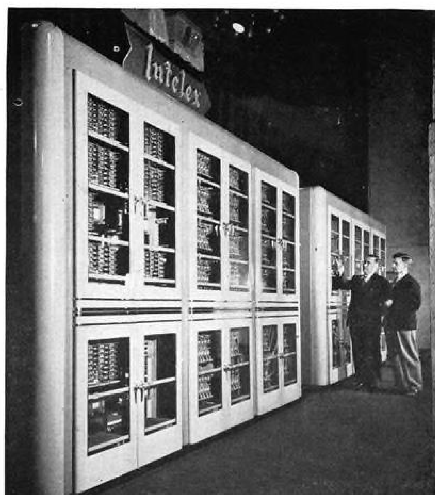
THE INTELEX, International Telephone & Telegraph Corp.'s electromechanical "brain," is a streamlined unit designed to handle requests for space in a matter of seconds. Bookings are recorded and reserved automatically.
