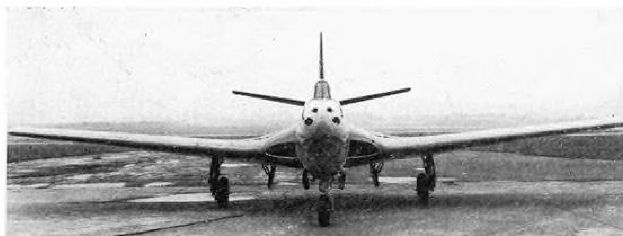
Phantom's head-on appearance emphasizes thickened wing roots with air inlets to turbojets. Design permits increased spar depth at root location.
