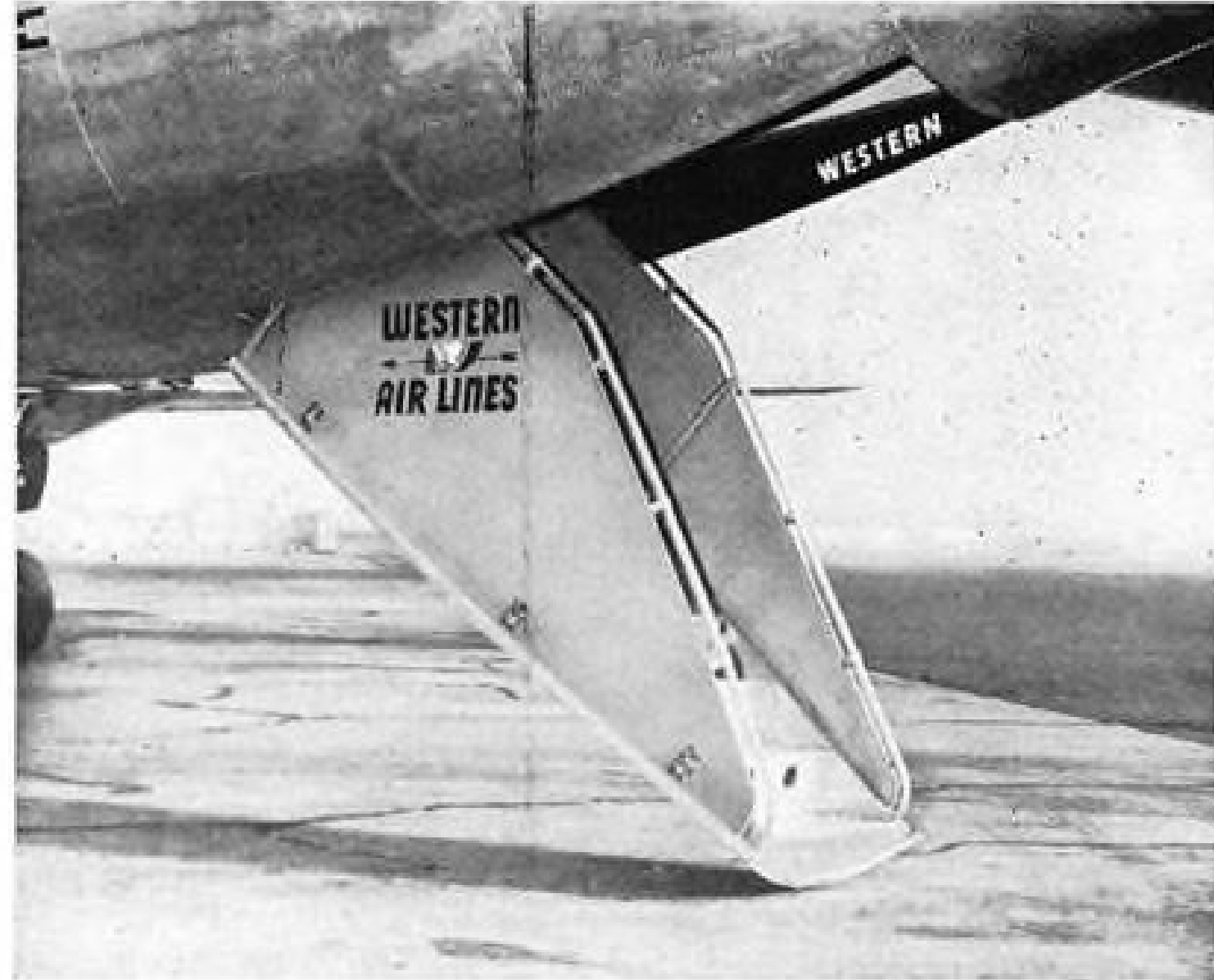
AFT integral stairway, featured in planes of Western Air Lines, is lowered directly under the tail section. Unlike the forward stairway, door and steps constitute a single unit.
