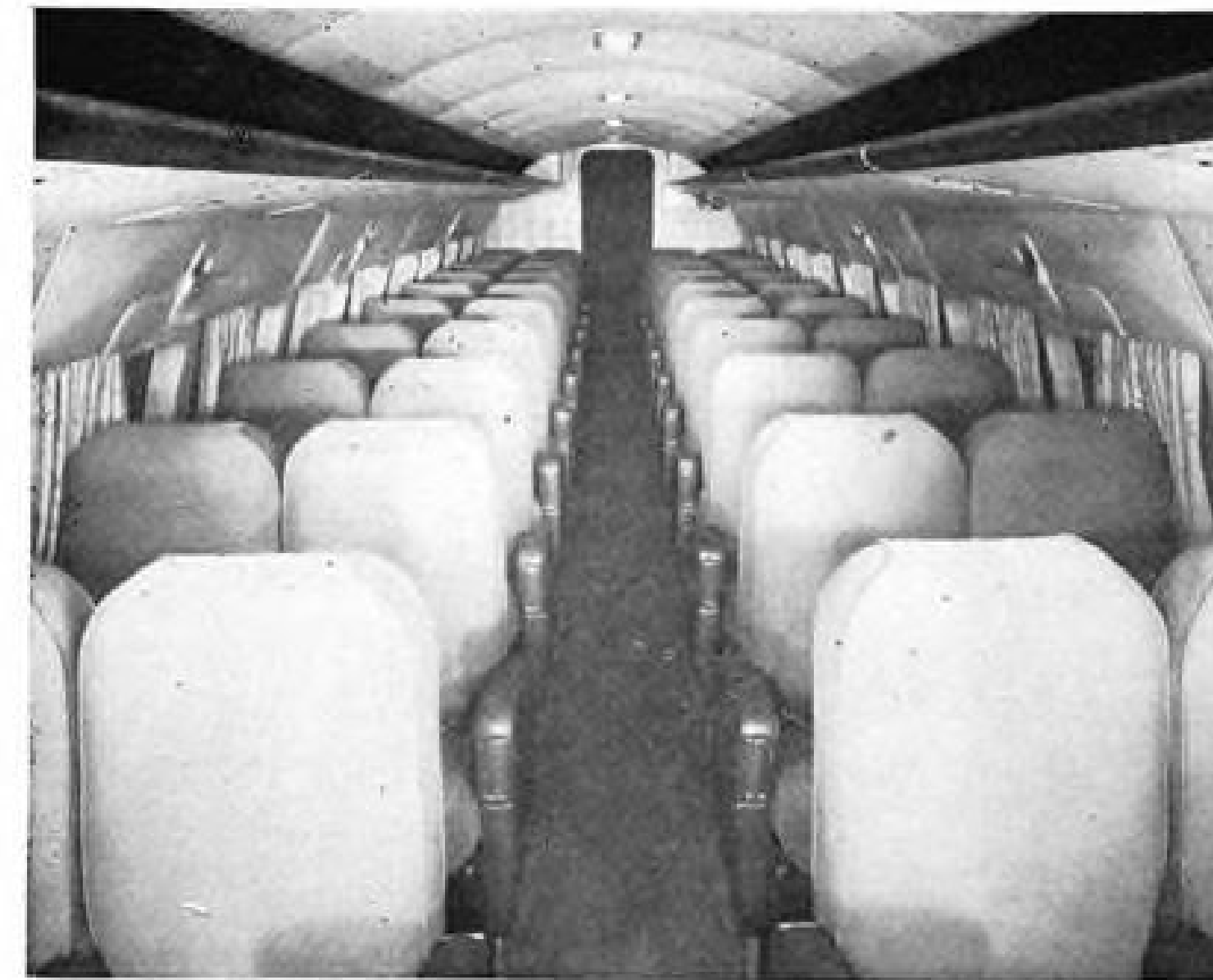
PASSENGER CABIN, looking aft from the first row of seats. The 40 seats are of special Convair design, filled with Fiberglas. Five emergency doors, two right, three left, open inward.
