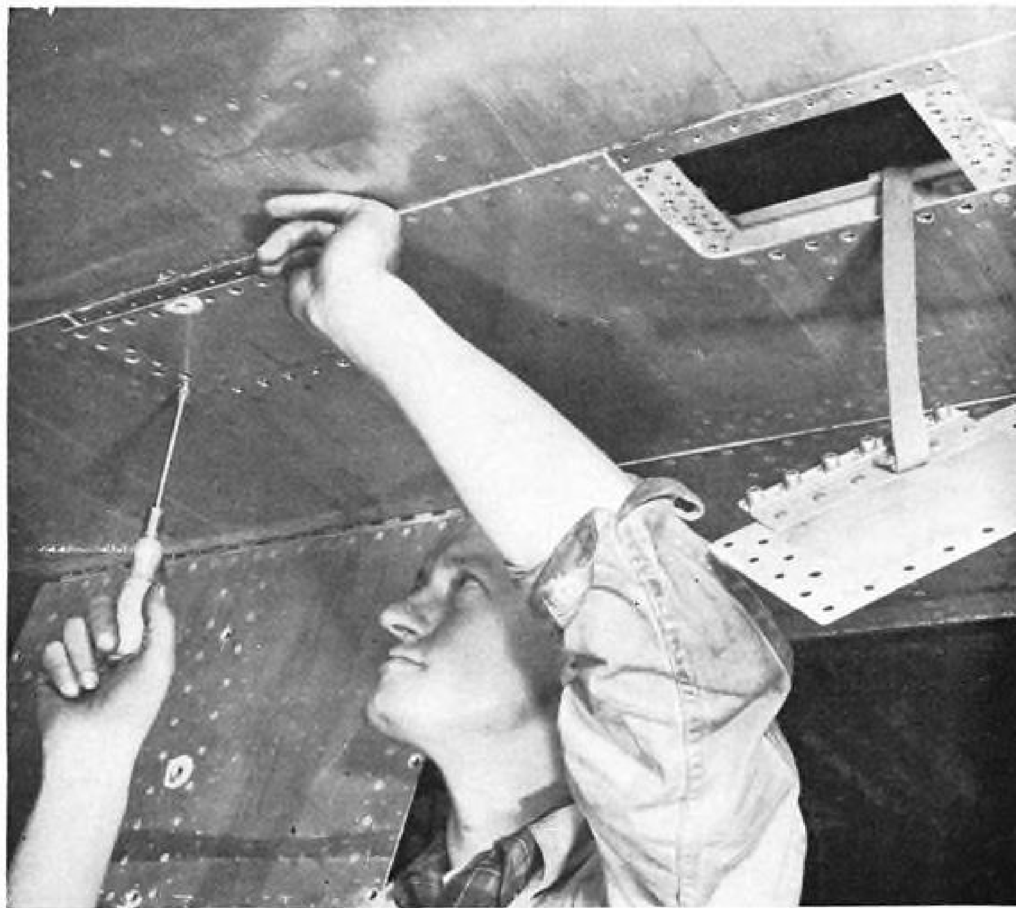
EASE OF ACCESS for servicing and inspection is afforded by some 300 plates and doors in Convair-Liner, similar to these
