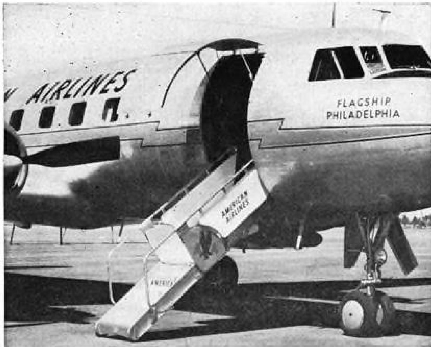
FORWARD integral stairway in American Airlines version of the Convair-Liner unfolds from within the plane as the door is opened. Door becomes a canopy, protecting passengers in bad weather.
