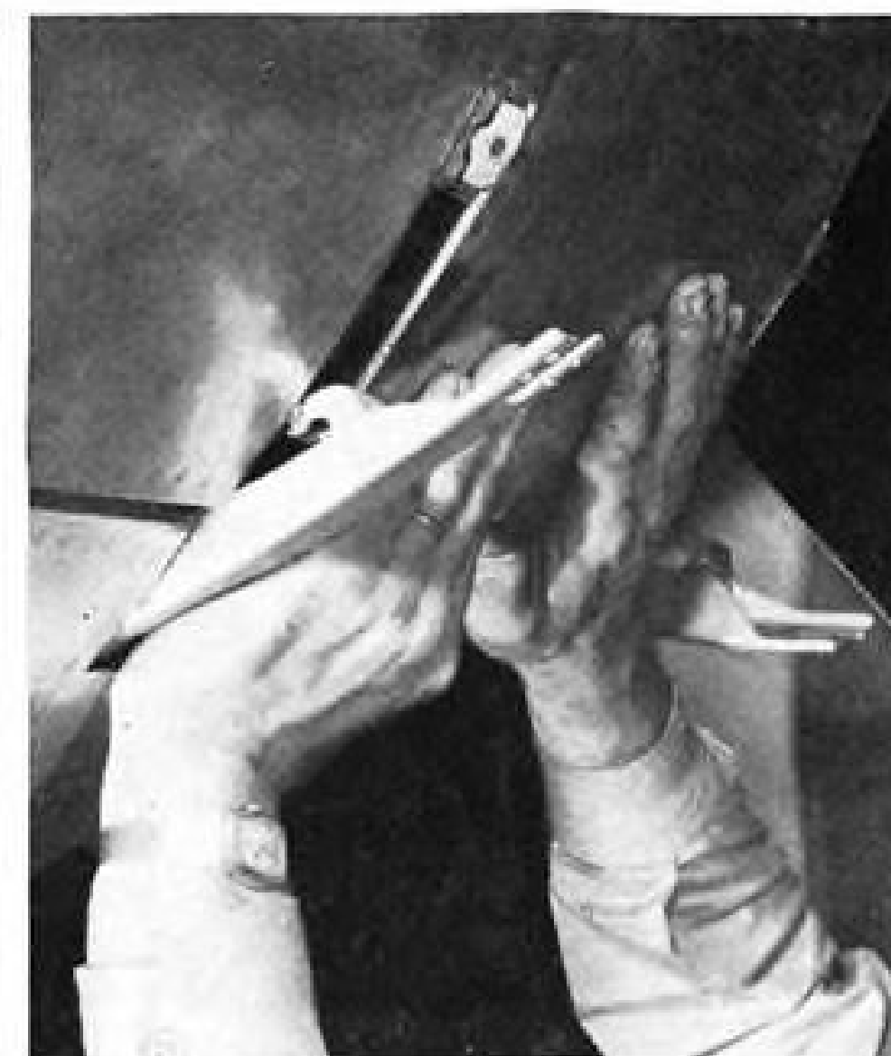
. . . over centering pin in other segment of cowl. Pin prevents shearing movement between sections. As latch closes . . .
