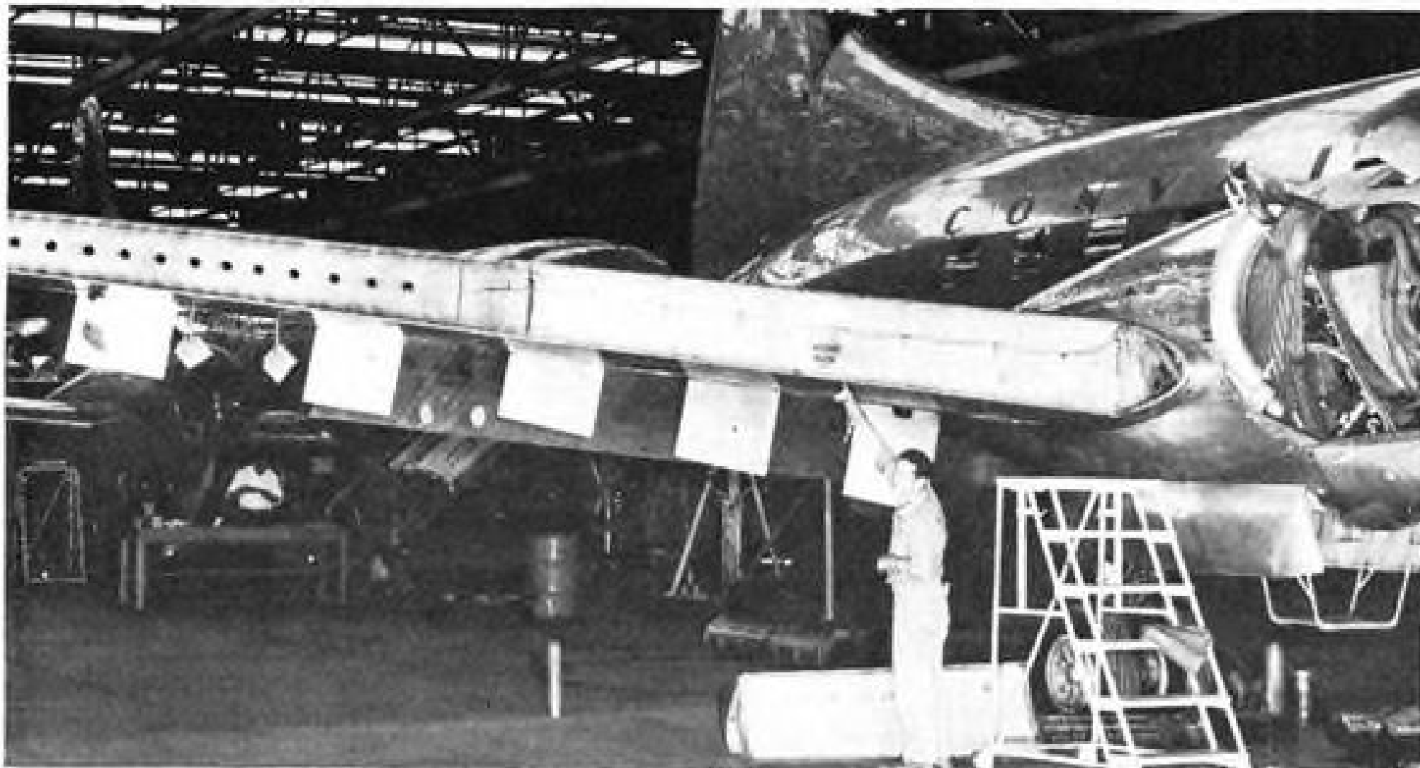
LEADING EDGE of wing outboard of nacelle is removable for inspection of wiring. Mechanic points to disconnect panel
