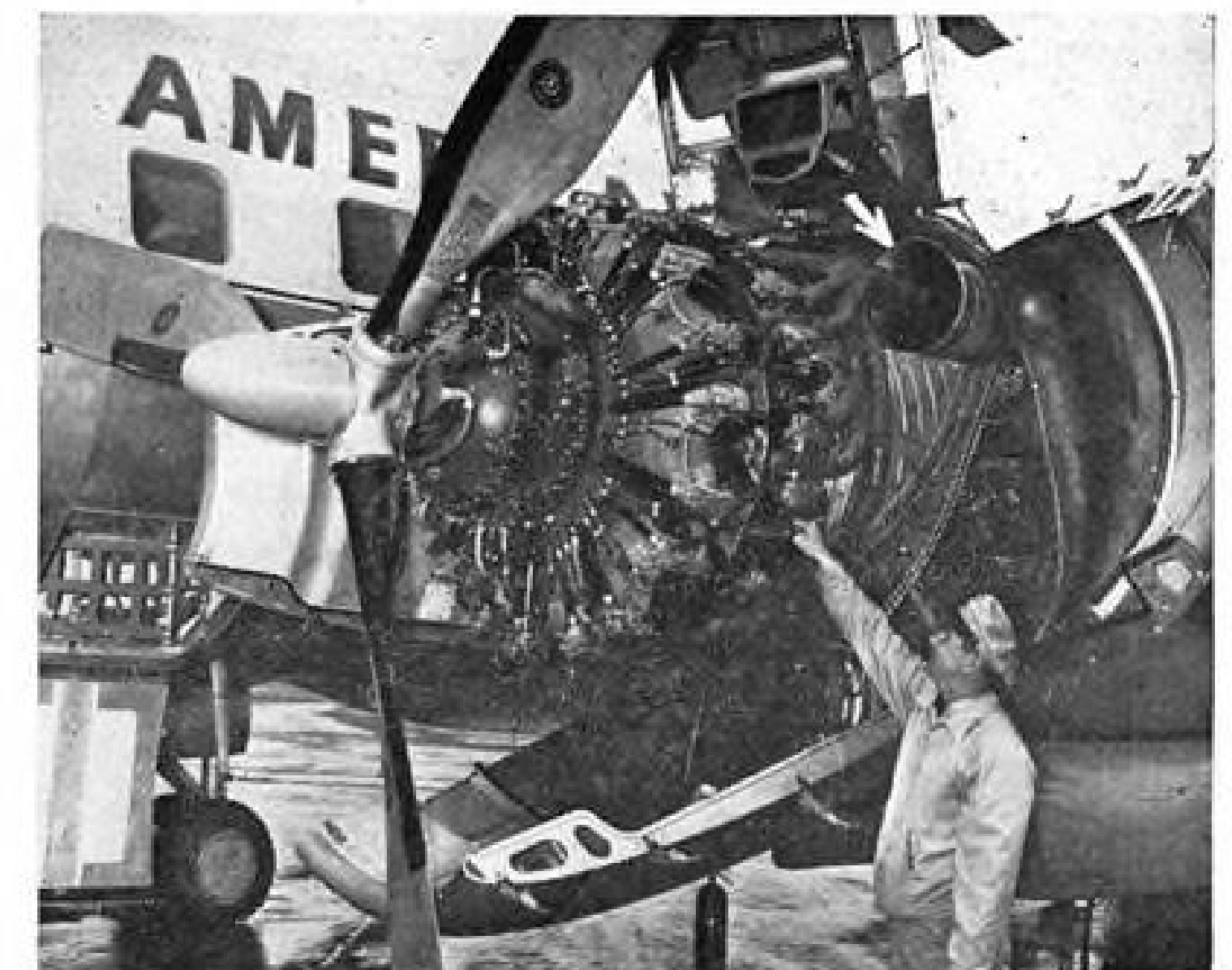
"ORANGE-PEEL" COWL, a Convair innovation, provides full access to engine. Arrow points to forward end of exhaust augmentation tube. Two tubes from each engine channel exhaust.
