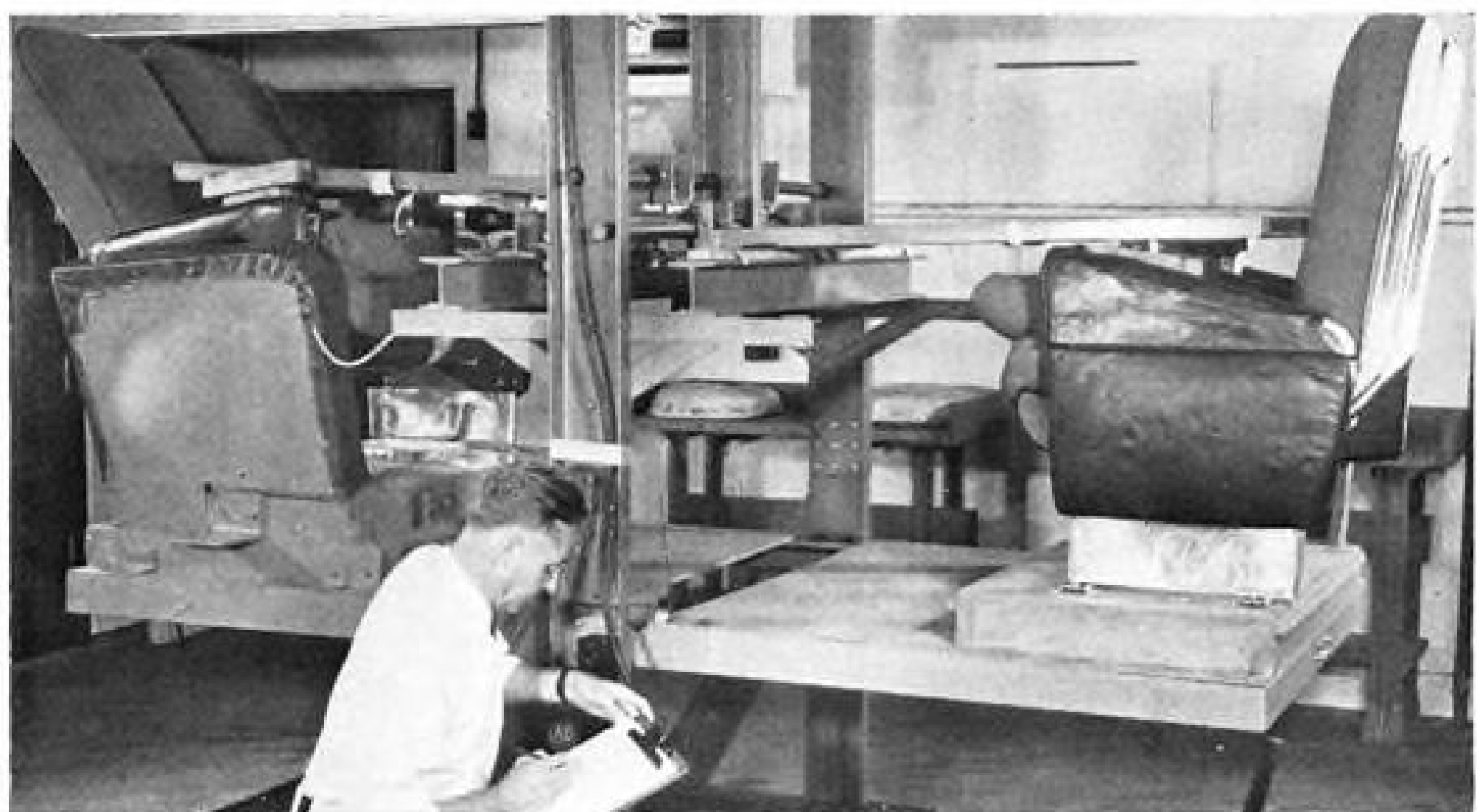
"DYNAMIC CYCLER" is a Convair device to test Fiberglas seat cushions. Seat raises up to contact the mold, and this
