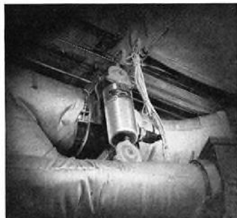
Close-up of one of the Barber-Colman units in the Convair-Liner—a cooling air control valve actuator.
