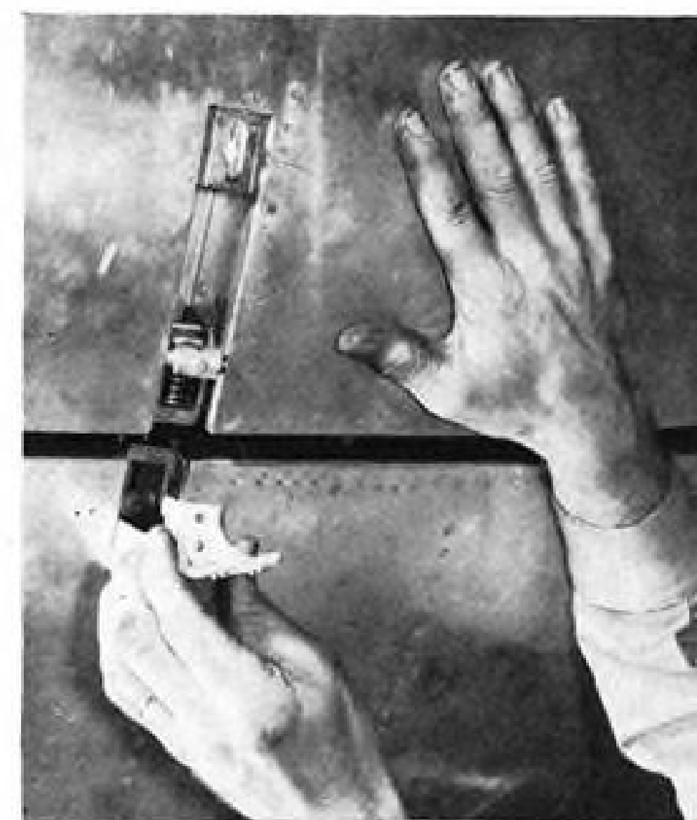
CLOSING COWL, mechanic brings together two segments, and pulls out latch from recess. Next step is to fit latch . . .
