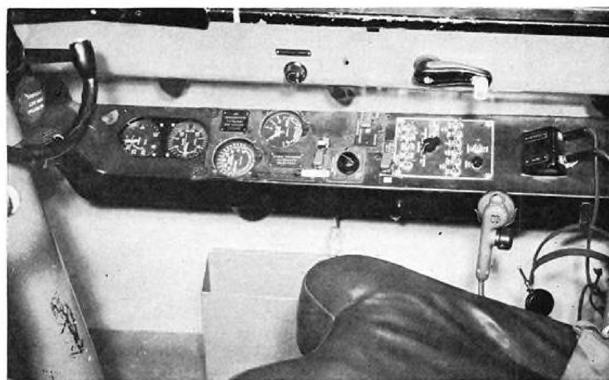
CABIN PRESSURE is selected by copilot through controls at dials seen third and fourth from left. Dials, left, give cabin
