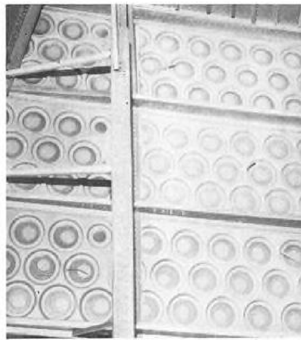
Trailing edge waffle construction.
