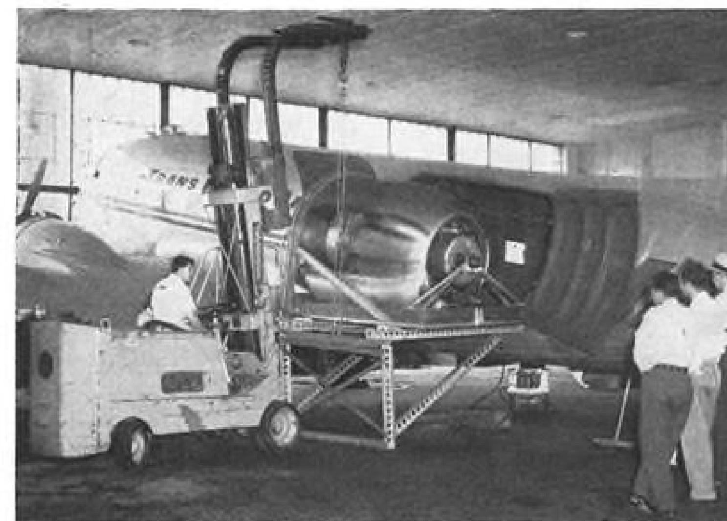
Tow motor hoists cradled power unit to loading ramp-platform and unit is moved automatically into the loading bay of the modified C-47.
