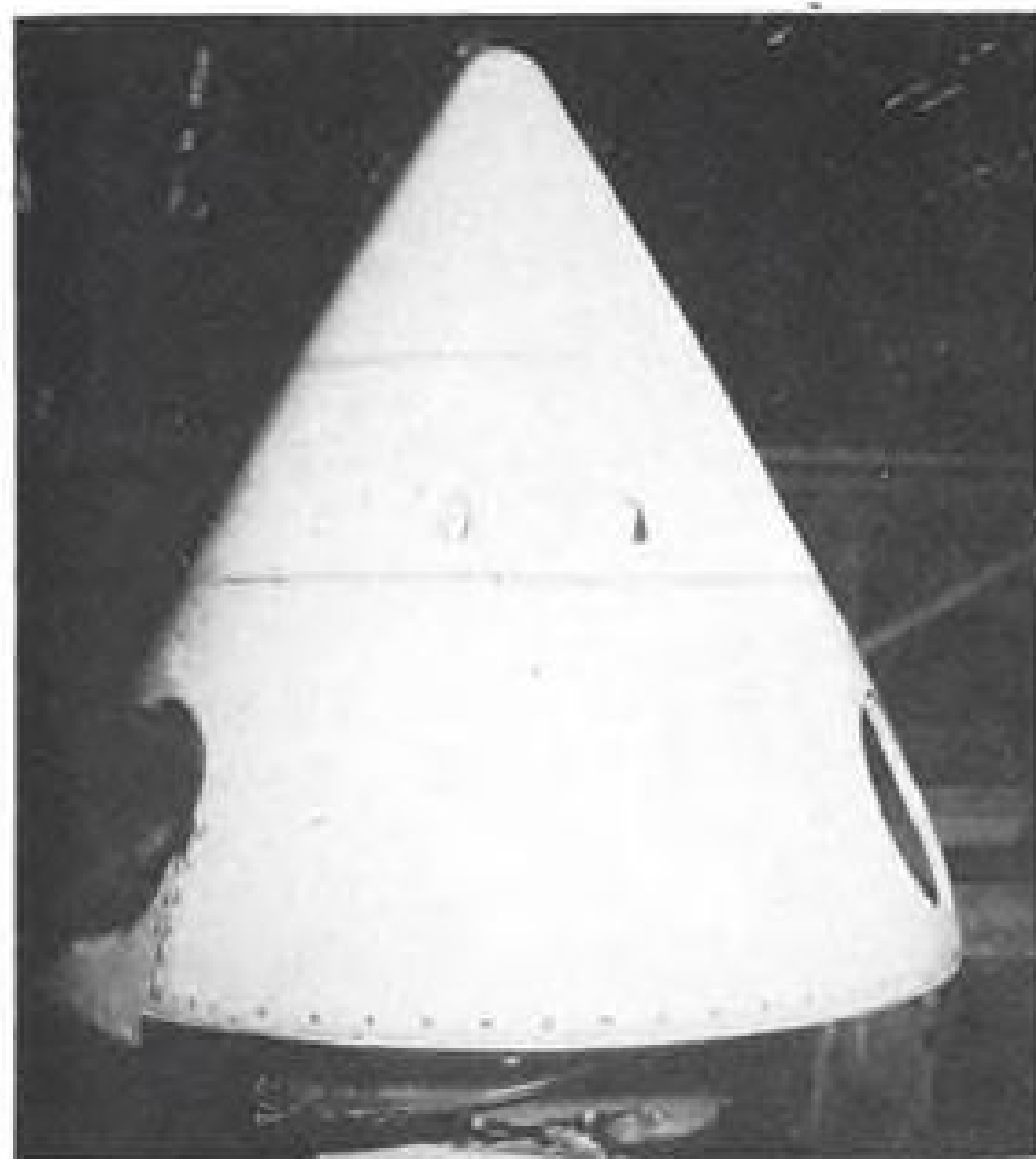
Magnesium propeller spinner.
