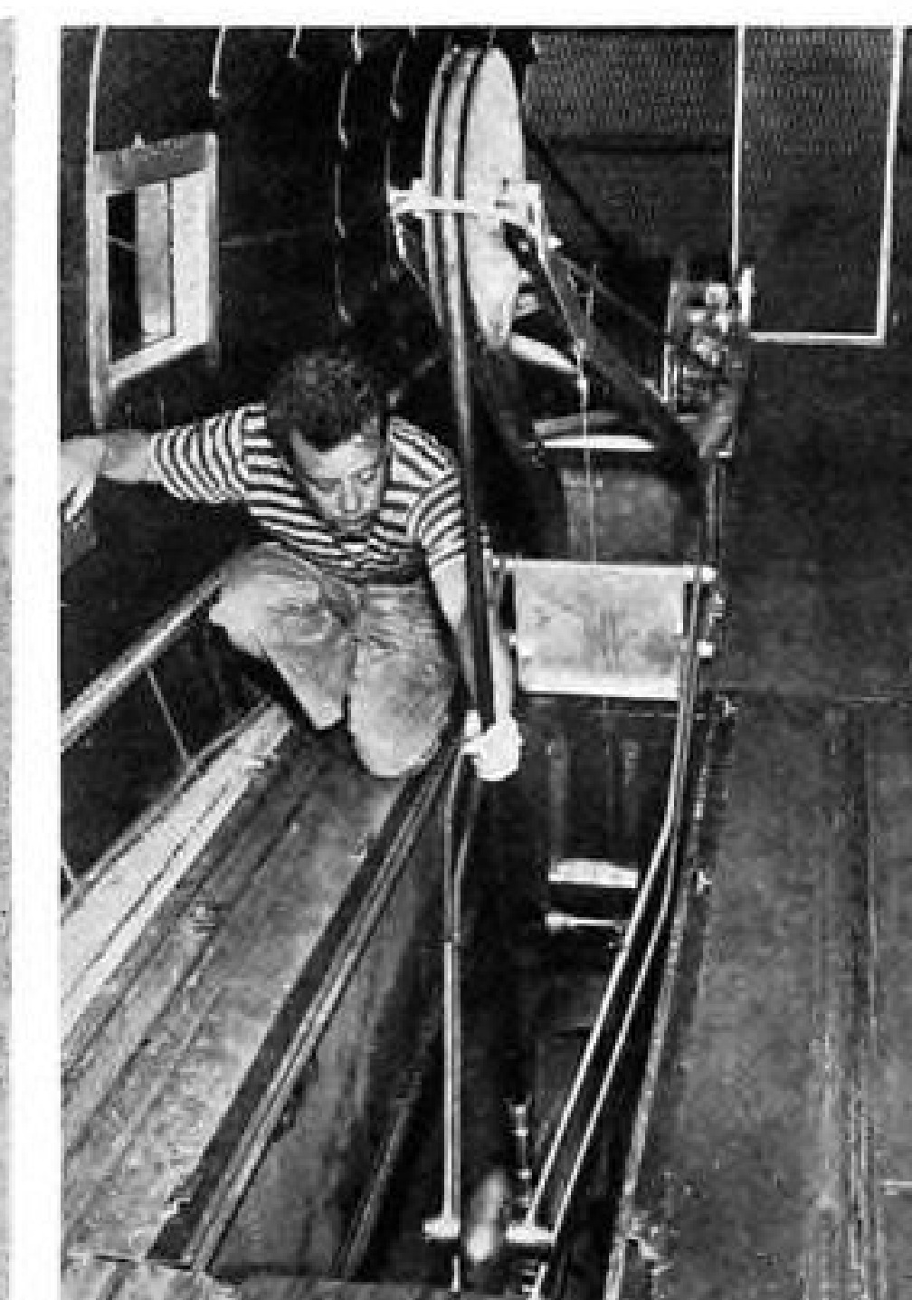
Trailing from Gulf Oil Corp.'s flying lab is magnetometer housed in nose of "bird" that is lowered via special hoist in the craft.
