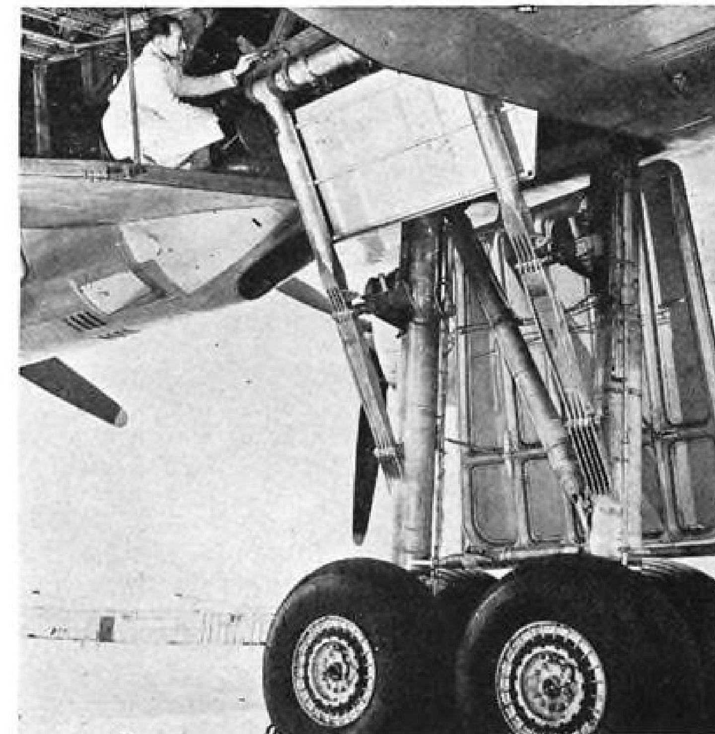
Craft's massive four-wheel, truck-type main gear required extensive research. Vanes on tire side impart prerotation.
