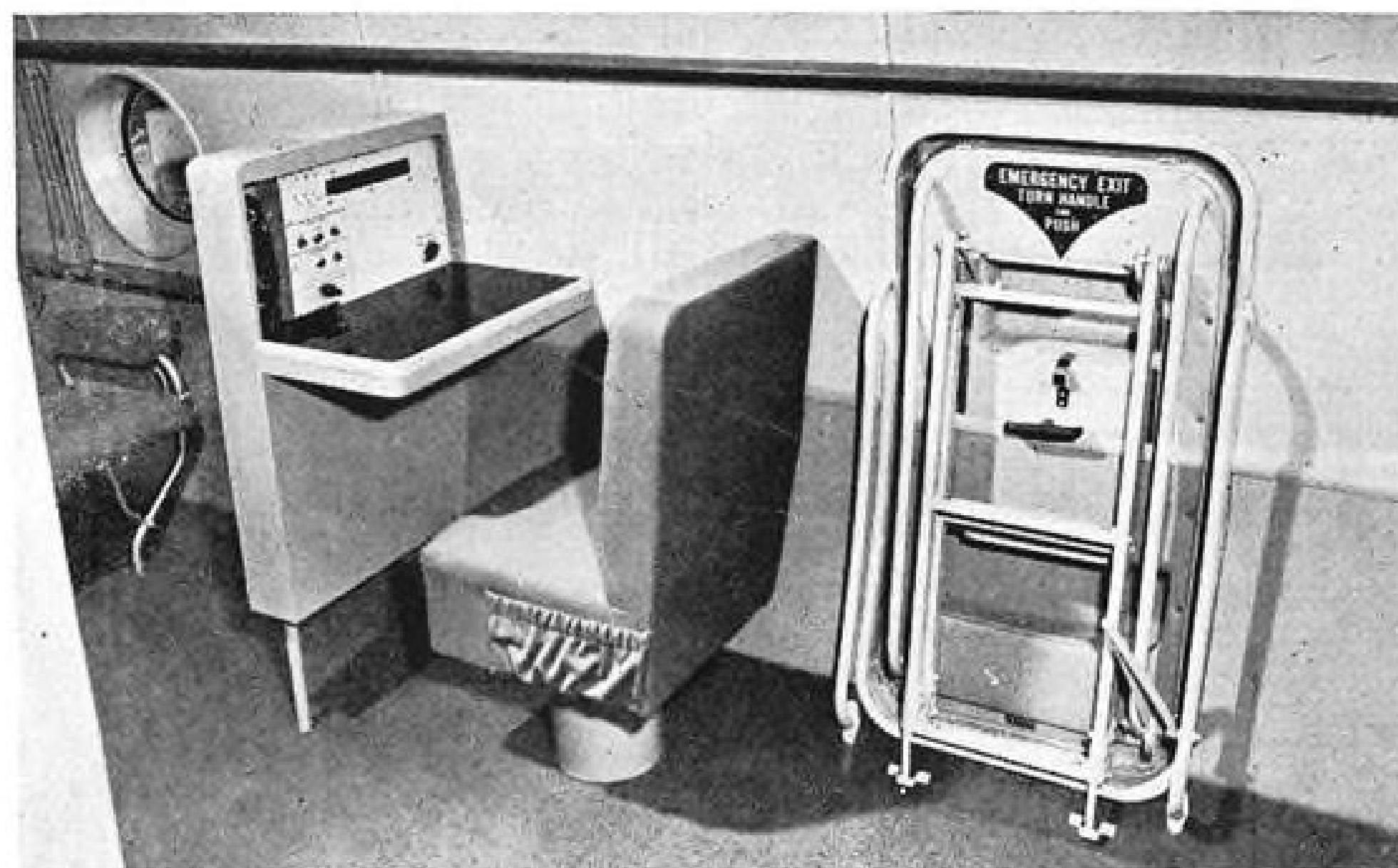
Flight steward's simple desk carries only light indicators, cabin air controls, and telephone.
