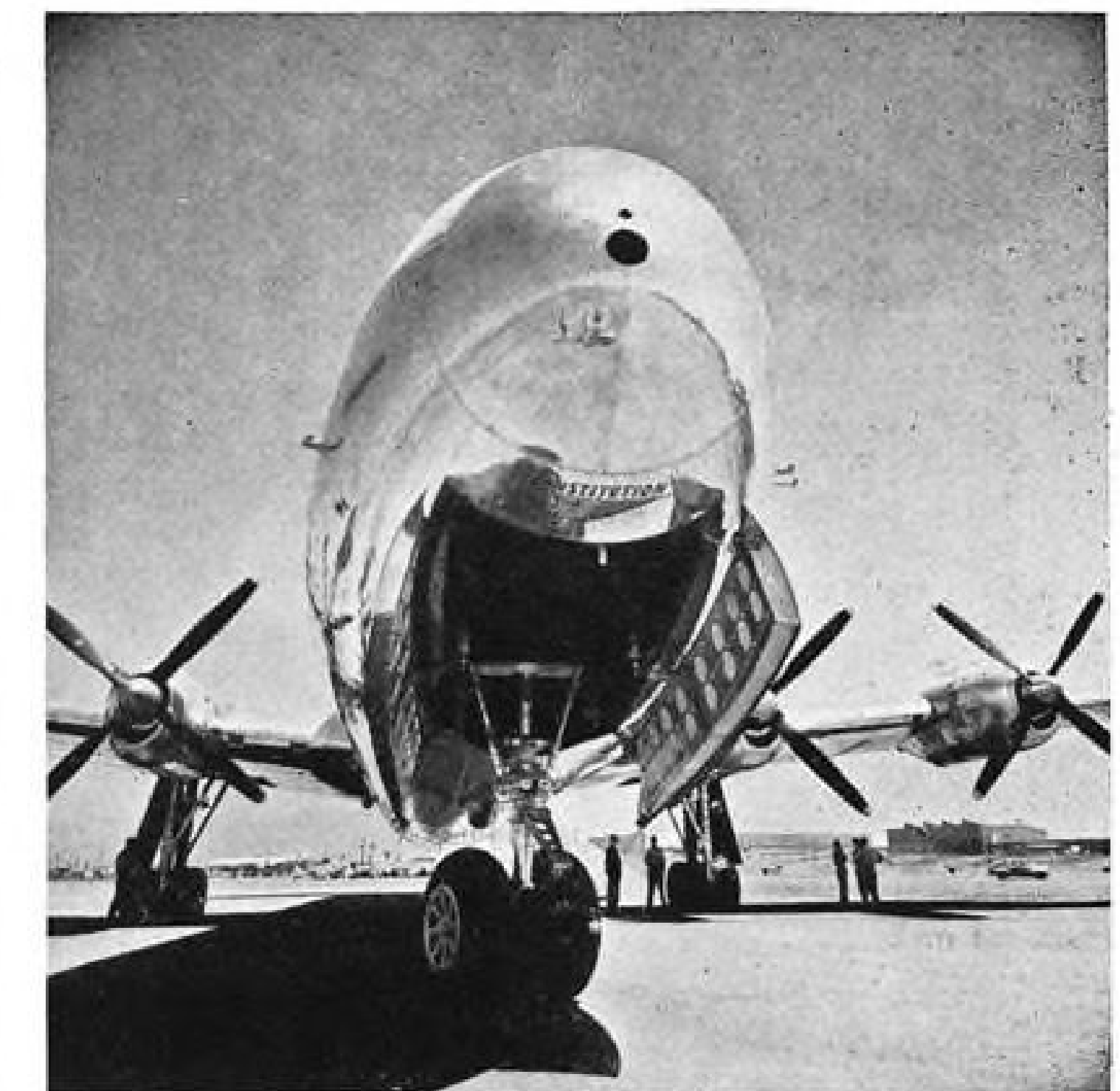
This spacious well, in addition to housing craft's dual nose wheel, is forward passenger entrance. Main entrance is aft of wing.
