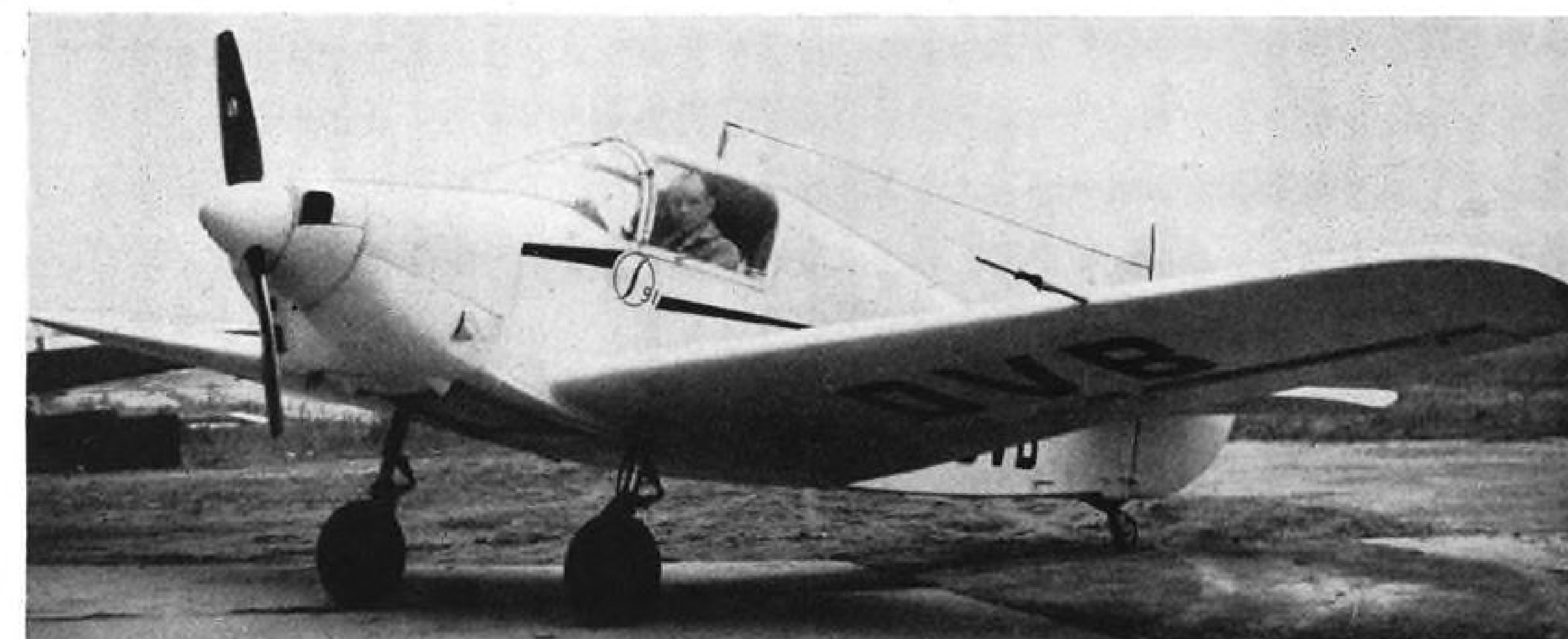
French S.I.P.A. sport plane is two-place, 85-hp., 125-mph. craft.
