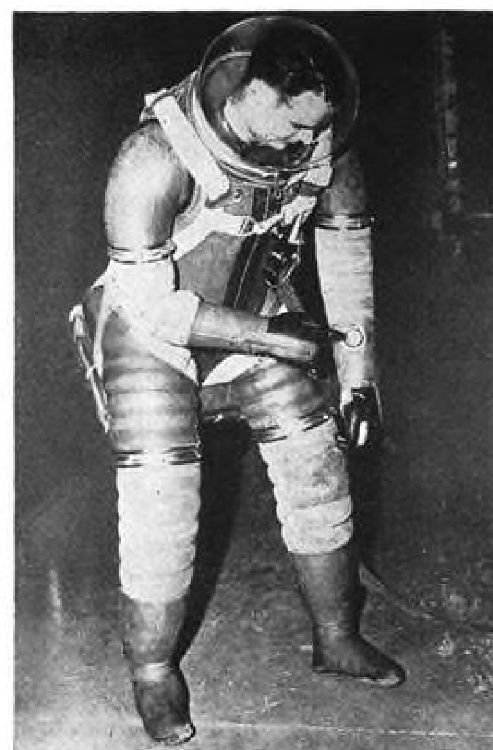
This pressurized, zipper-fastened strato-suit developed by B. F. Goodrich under military guidance has oxygen and communication provisions piped-in by means of a single conduit which can be disconnected quickly by the pilot in the event of emergency.
