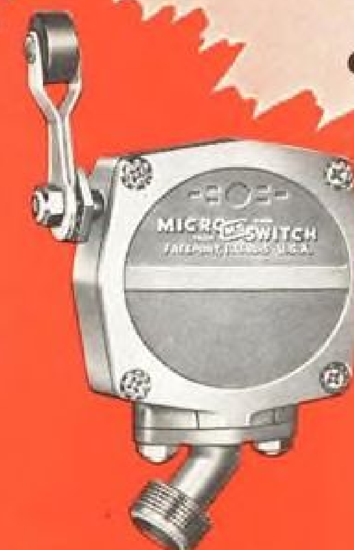
MICRO LMR aircraft switch has sturdy die cast aluminum housing. Mounting holes make possible four position mounting on either face. Rotary lever arm actuator is adjustable through 360 degrees. Total travel of roller arm is 90° in either direction. AN number 3233.
