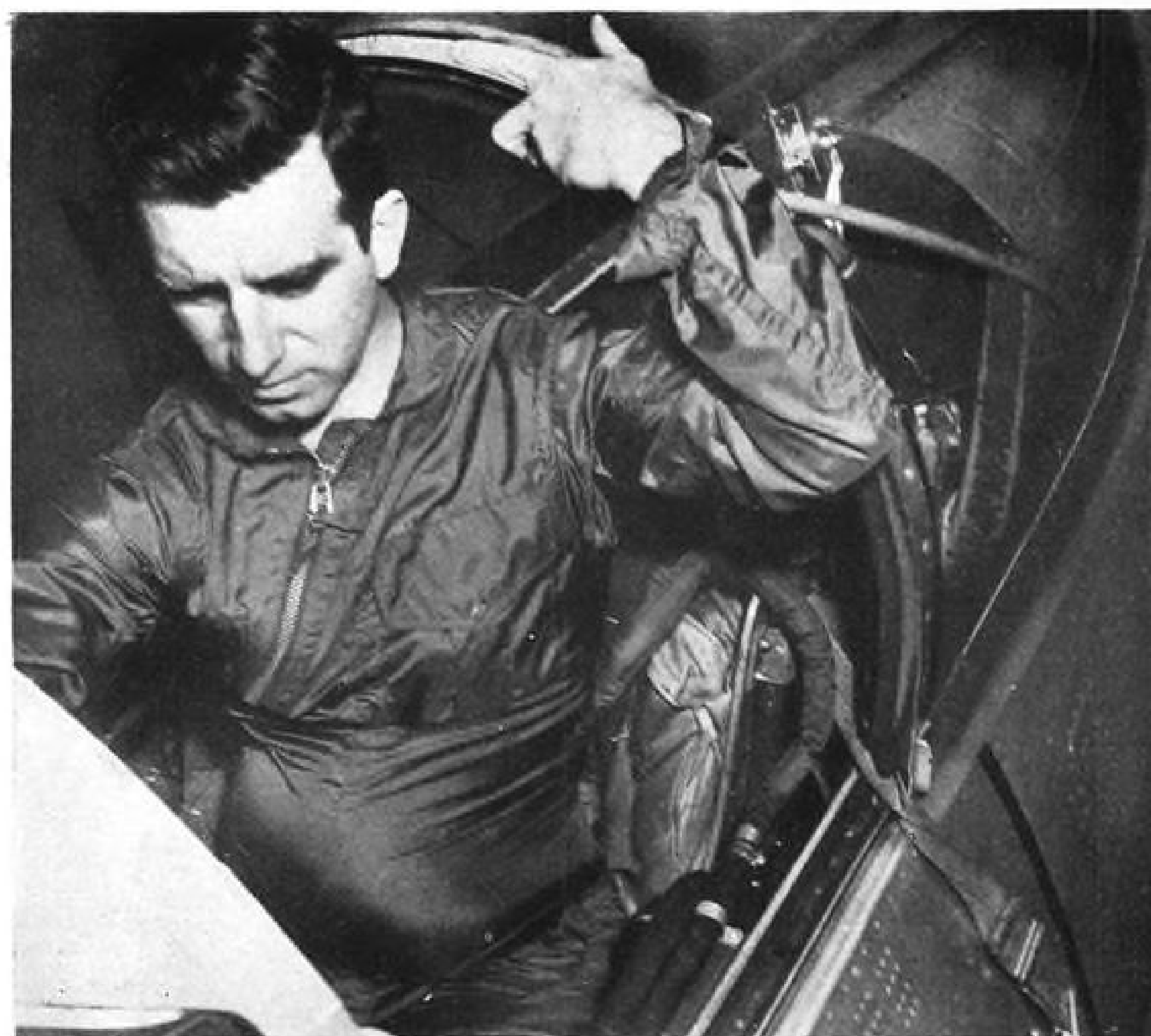
This anti-blackout suit has inflated bladder over abdomen to keep blood from leaving head.
