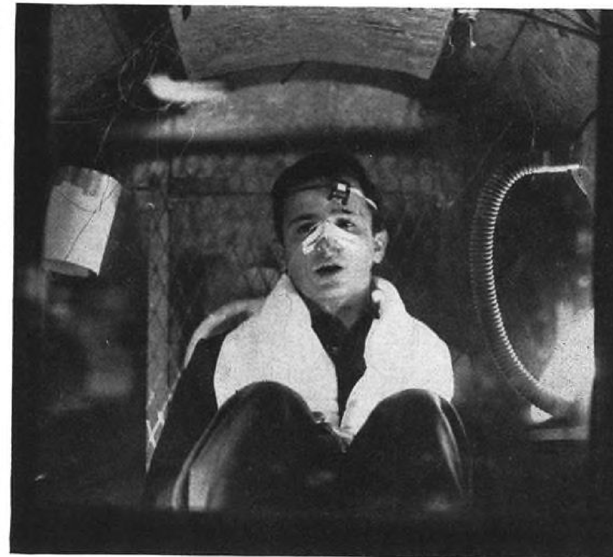
In "hot-box" test, subject's reaction is observed and recorded as 200 F. is exceeded.
