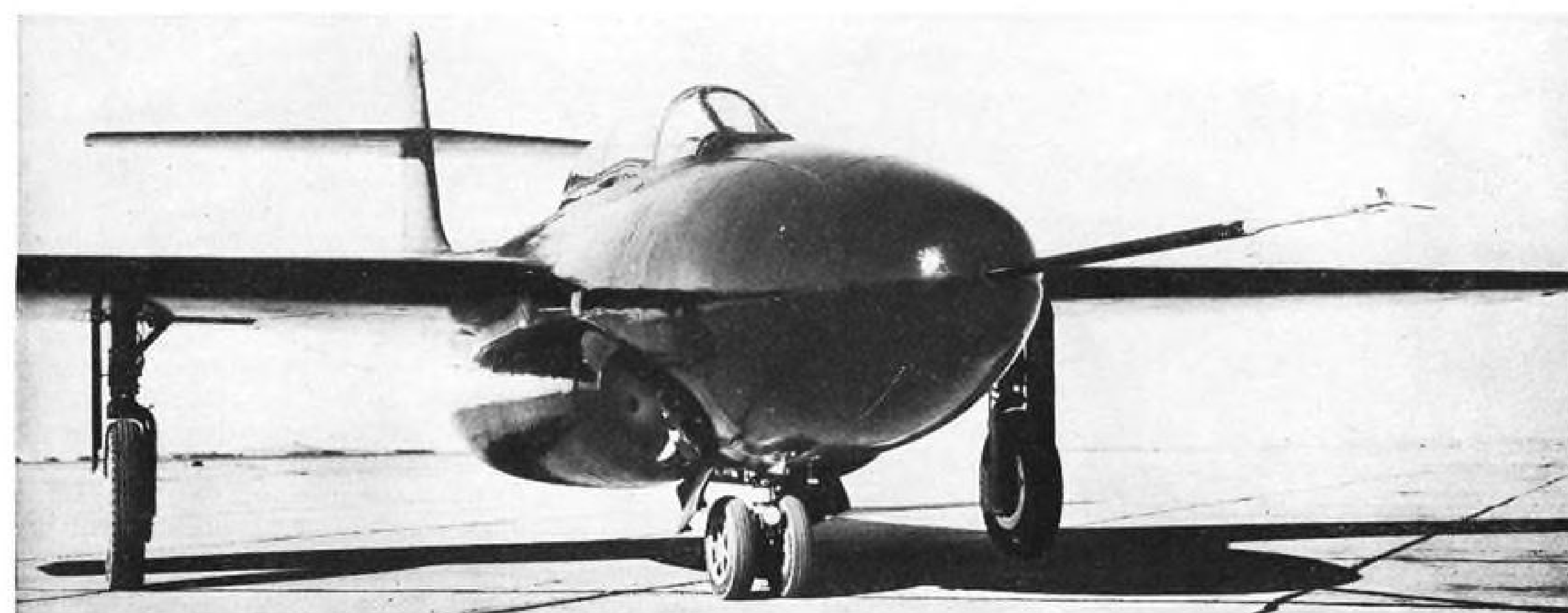
NORTHROP'S XF-89. Great weight (30,000 lb.) calls for large main wheels and double nose wheels.
