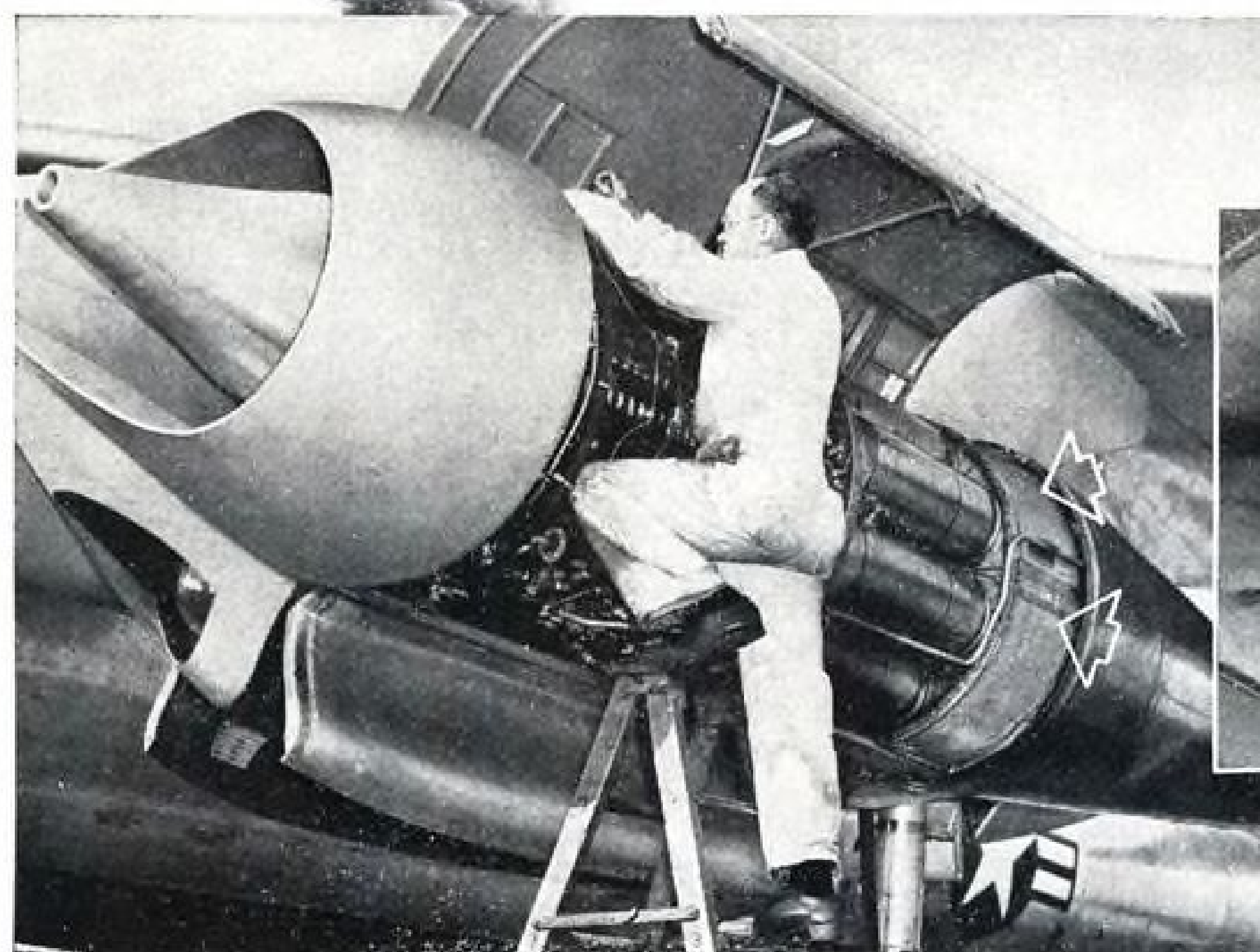
ABOVE: Arrows indicate Thermoflex Blanket around turbine casing of the Boeing XB-47.
