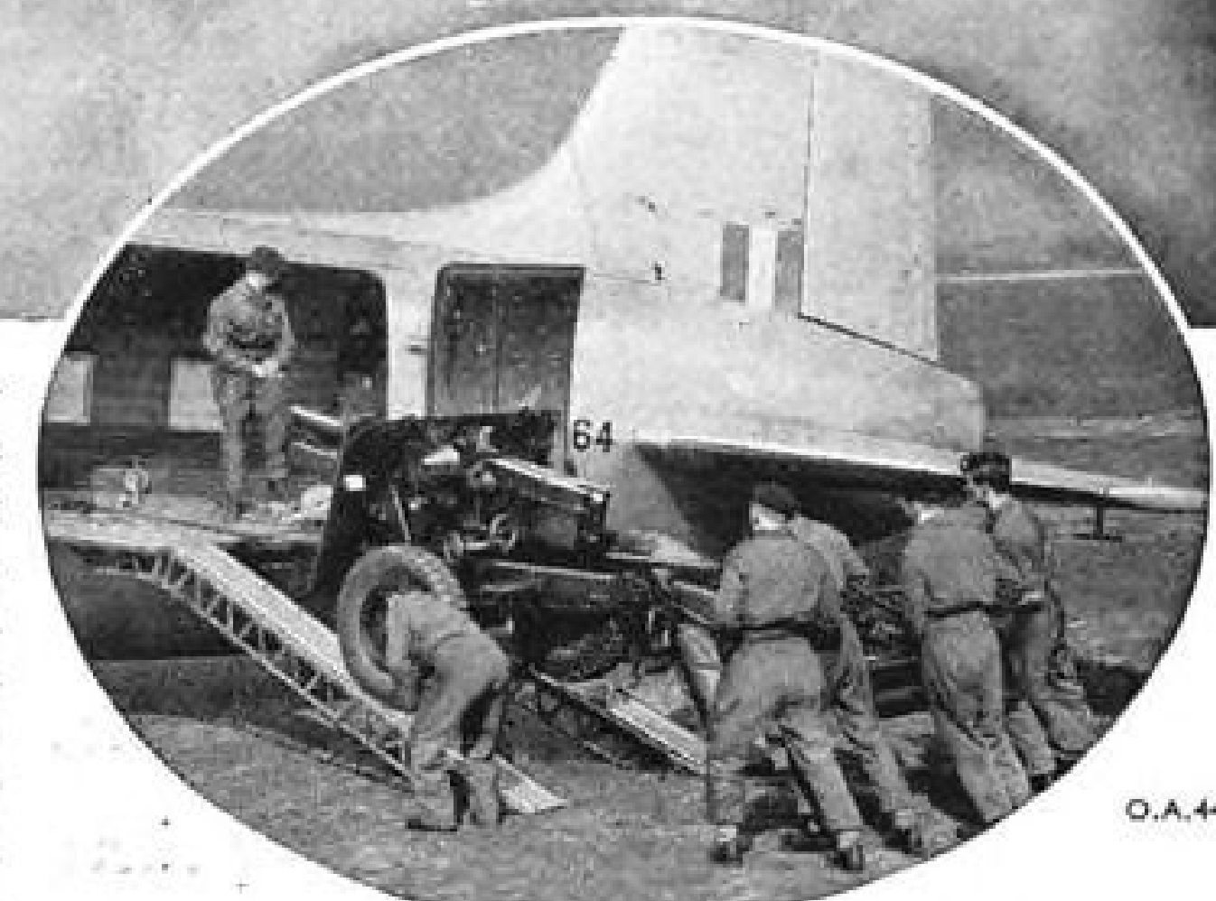
MILITARY DOORS. Specially wide doors are arranged to allow speedy, unrestricted loading and unloading of Jeeps, guns and other equipment. An inset door is provided for the dropping of paratroops or supplies.
