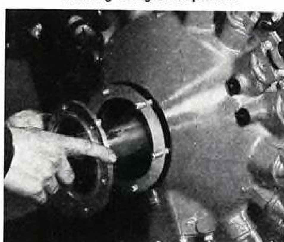
To simplify exact loading of outer race of propeller shaft thrust bearing
