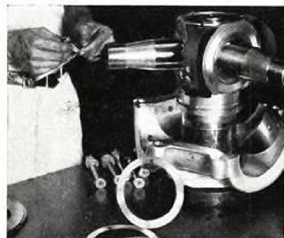
To regulate fit between spider and barrel in prop assembly
