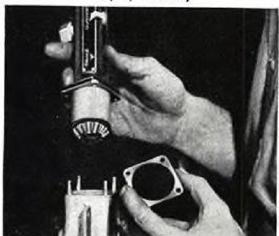
For adjustment of gear meshing in landing gear control machinery
