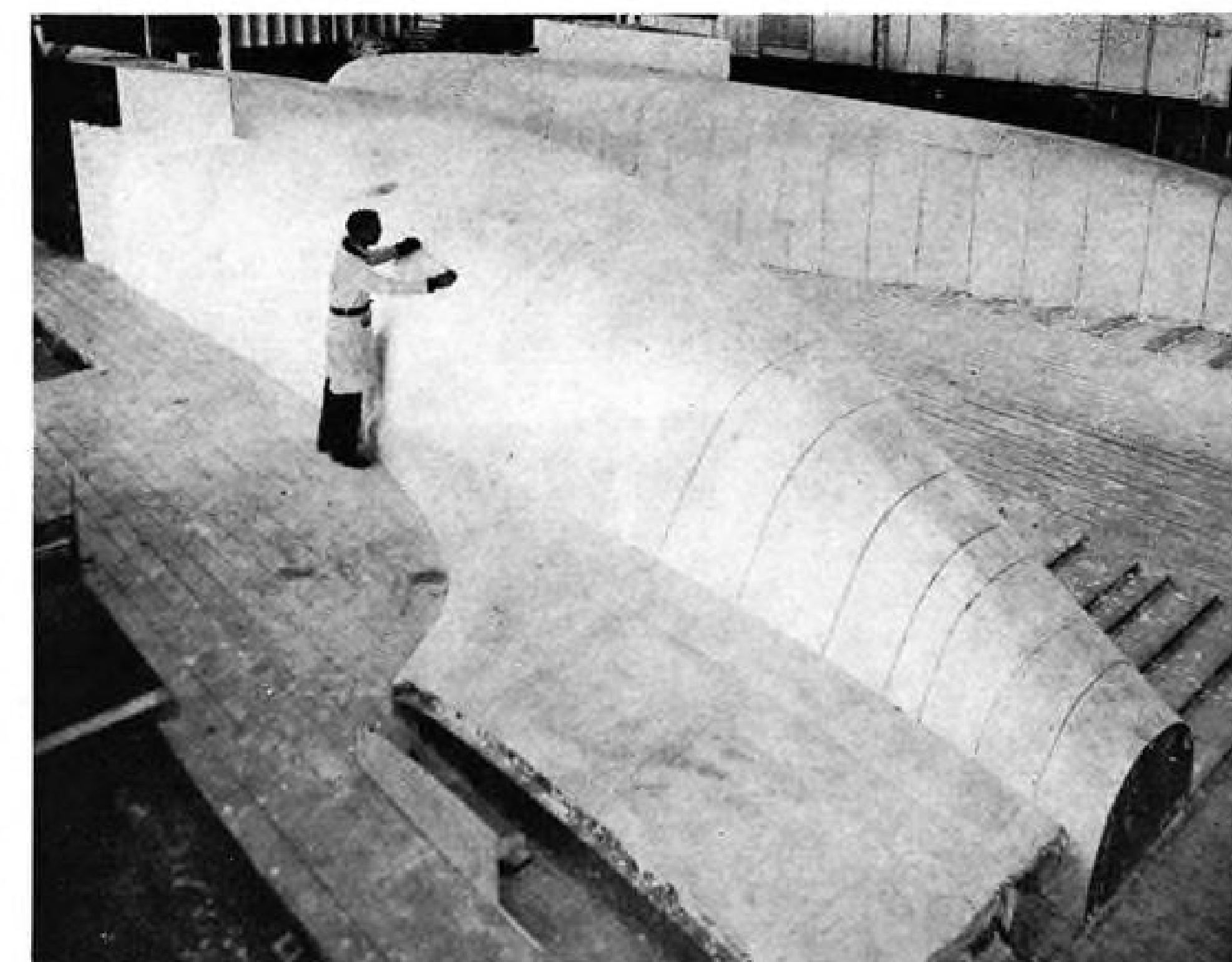
Raider's fuselage in plaster. Mockup facilitates fabrication of dies, jigs and tools.
