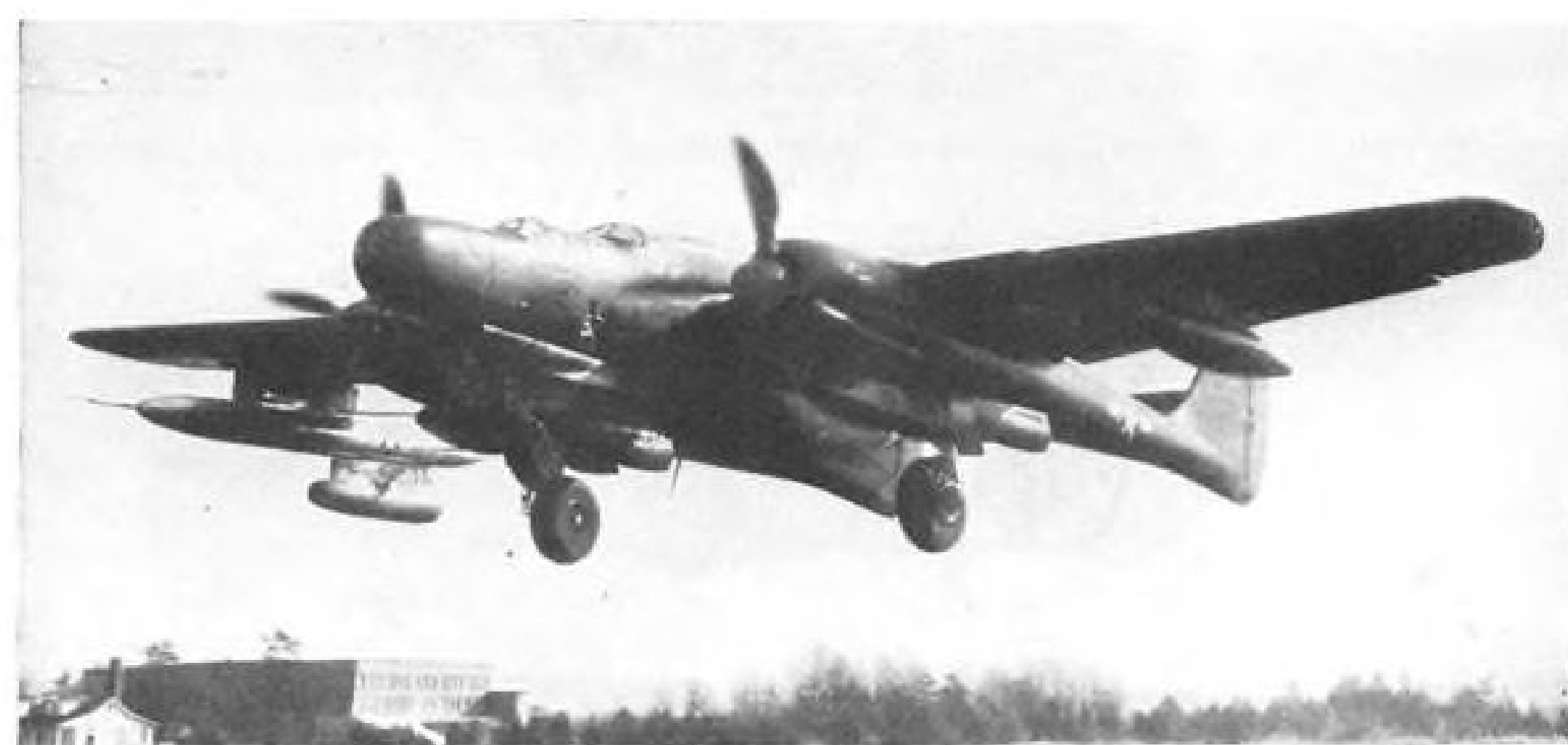
Gorgon IV is borne aloft under right wing of modified Northrop Black Widow . . .
