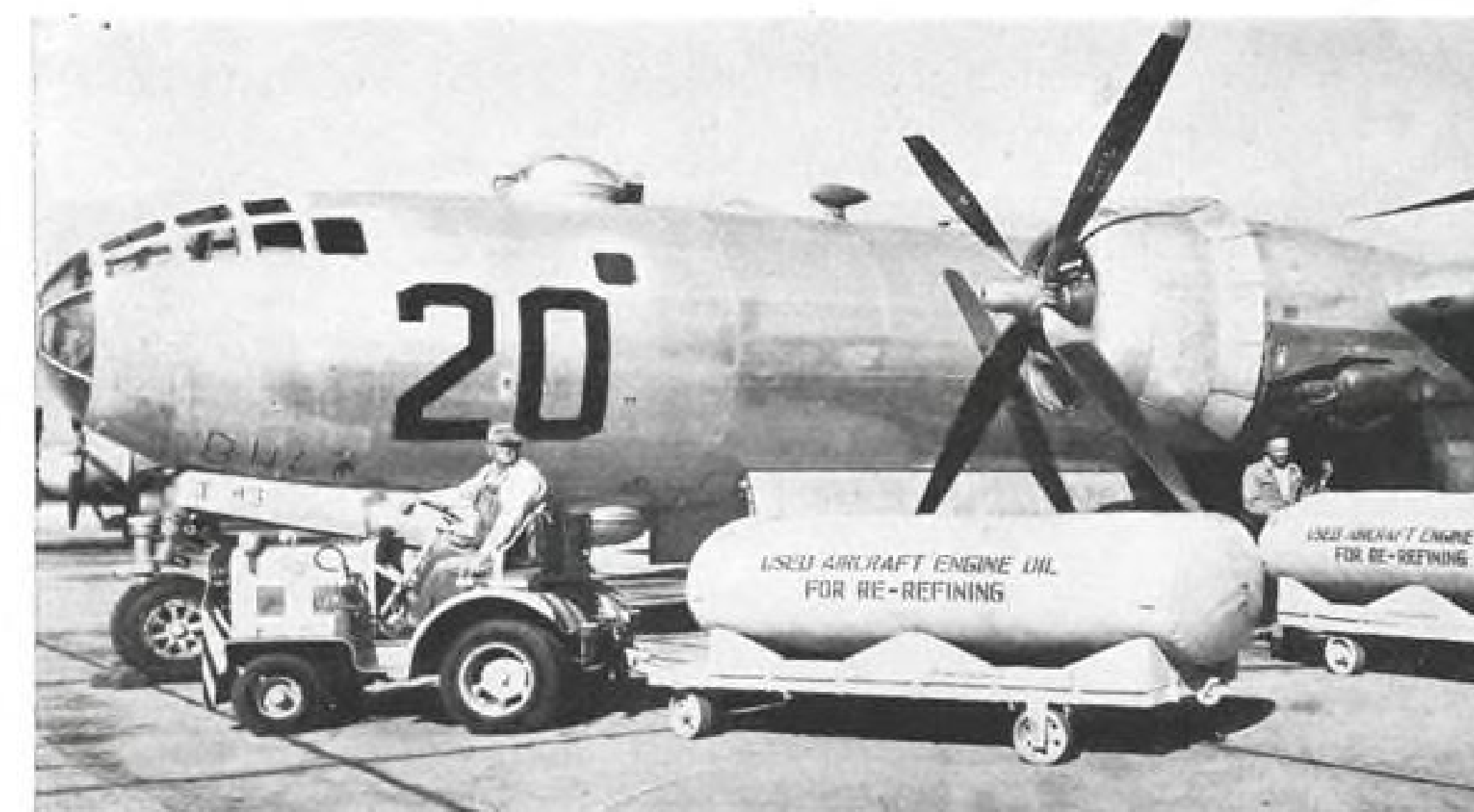
Oil reclamation program is aided by maintenance tugs which tow tanks of accumulated used lube to facilitate drainage from craft on the line. Tanks were B-29 units.
