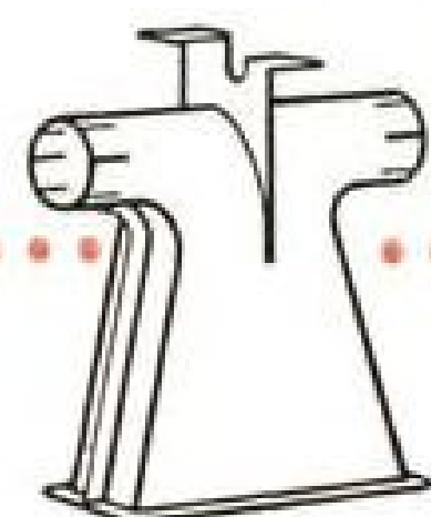
AIR DISPENSER ASSEMBLY Welded: 100 parts in 20 hours. Brazed: 100 parts in 2 hours.
