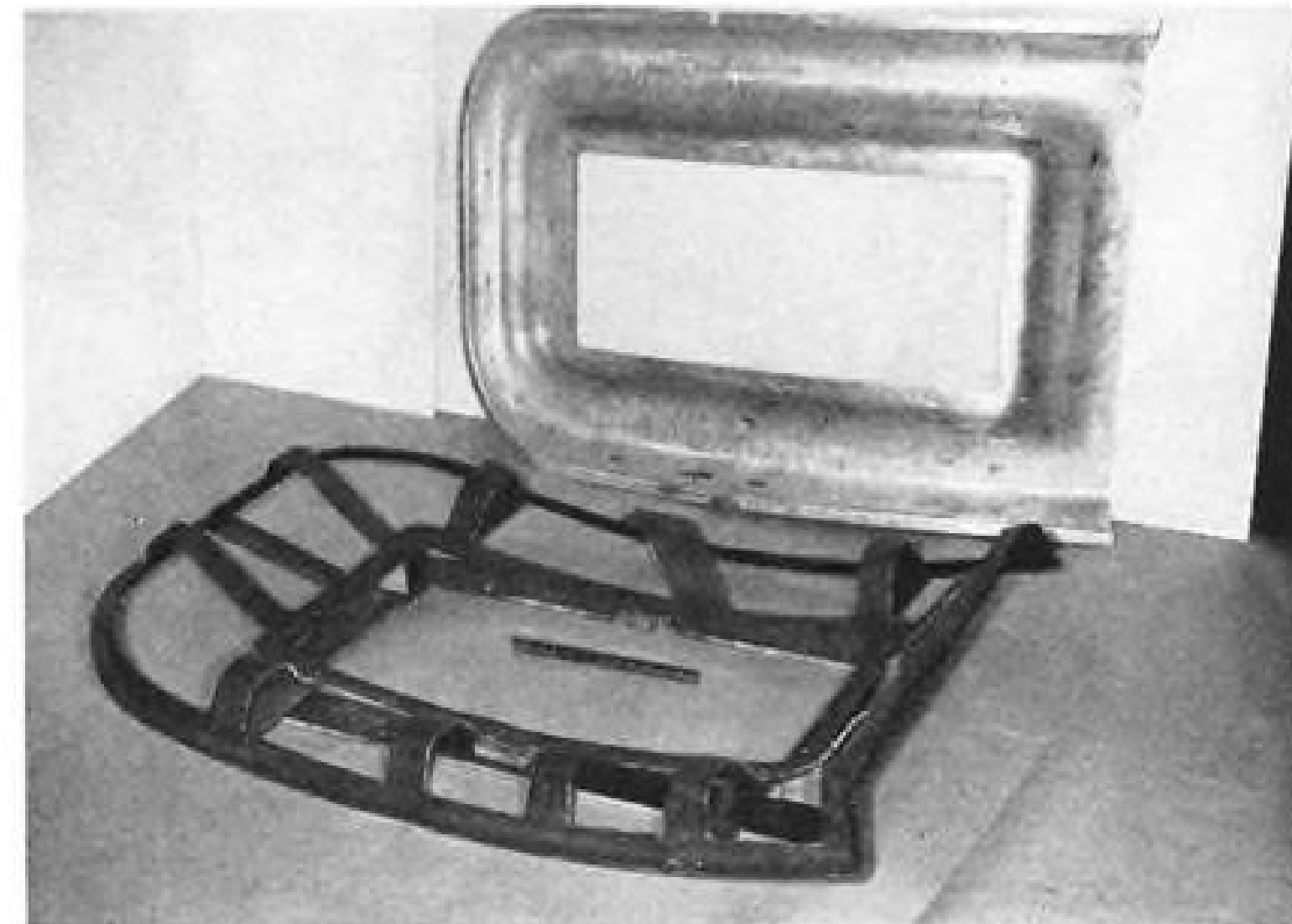
sible with steel counterpart. Right: More than 50 man-hours were saved in fabrication of this routing fixture used in manufacture of large part for F-84 Thunderjet.
