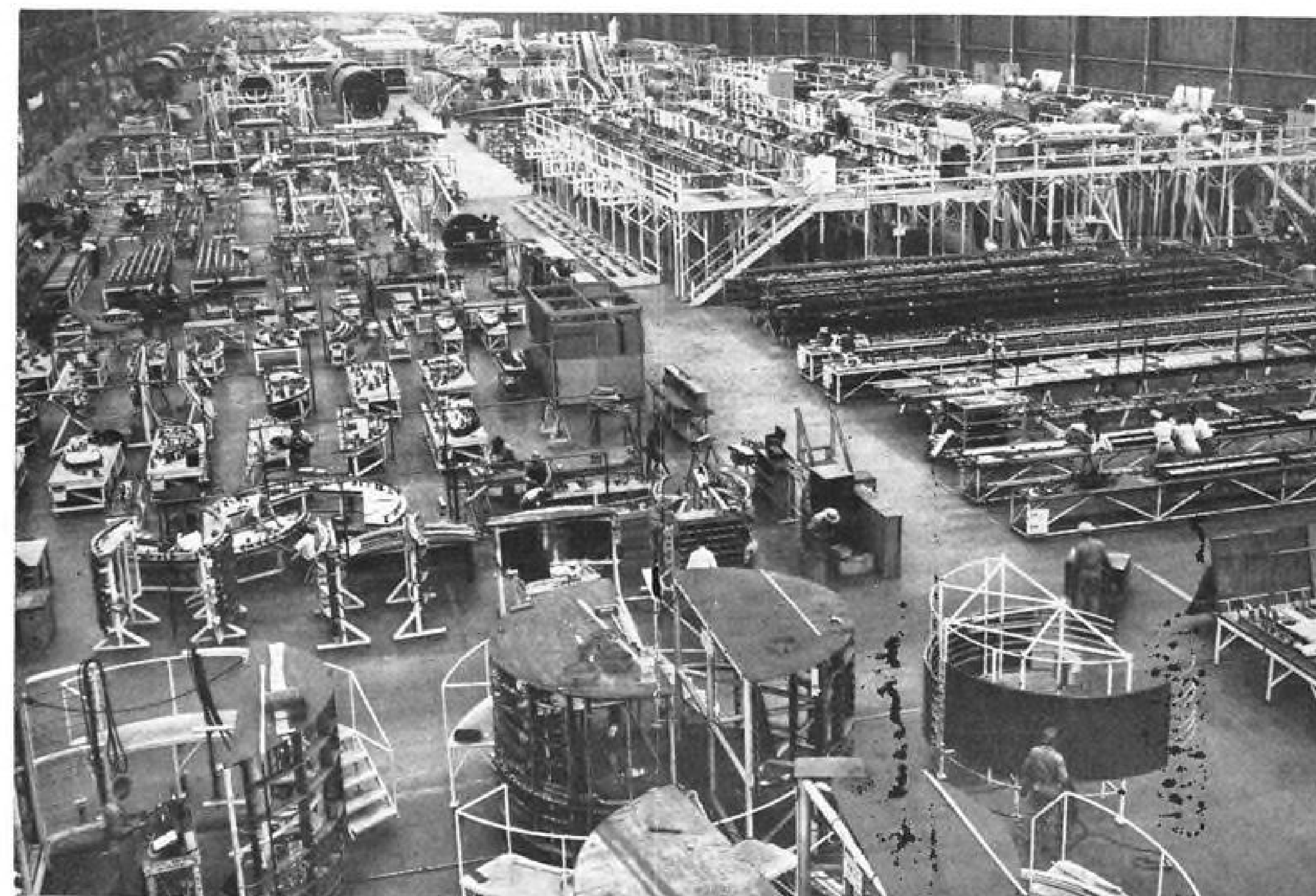
Tremendous stretch of plant's 200-ft. width is strikingly revealed in view from site of bomb bay fabrication. At upper right are seen major assembly fixtures for bomb bay truss structure. Area in foreground and at left is for subassembly.
