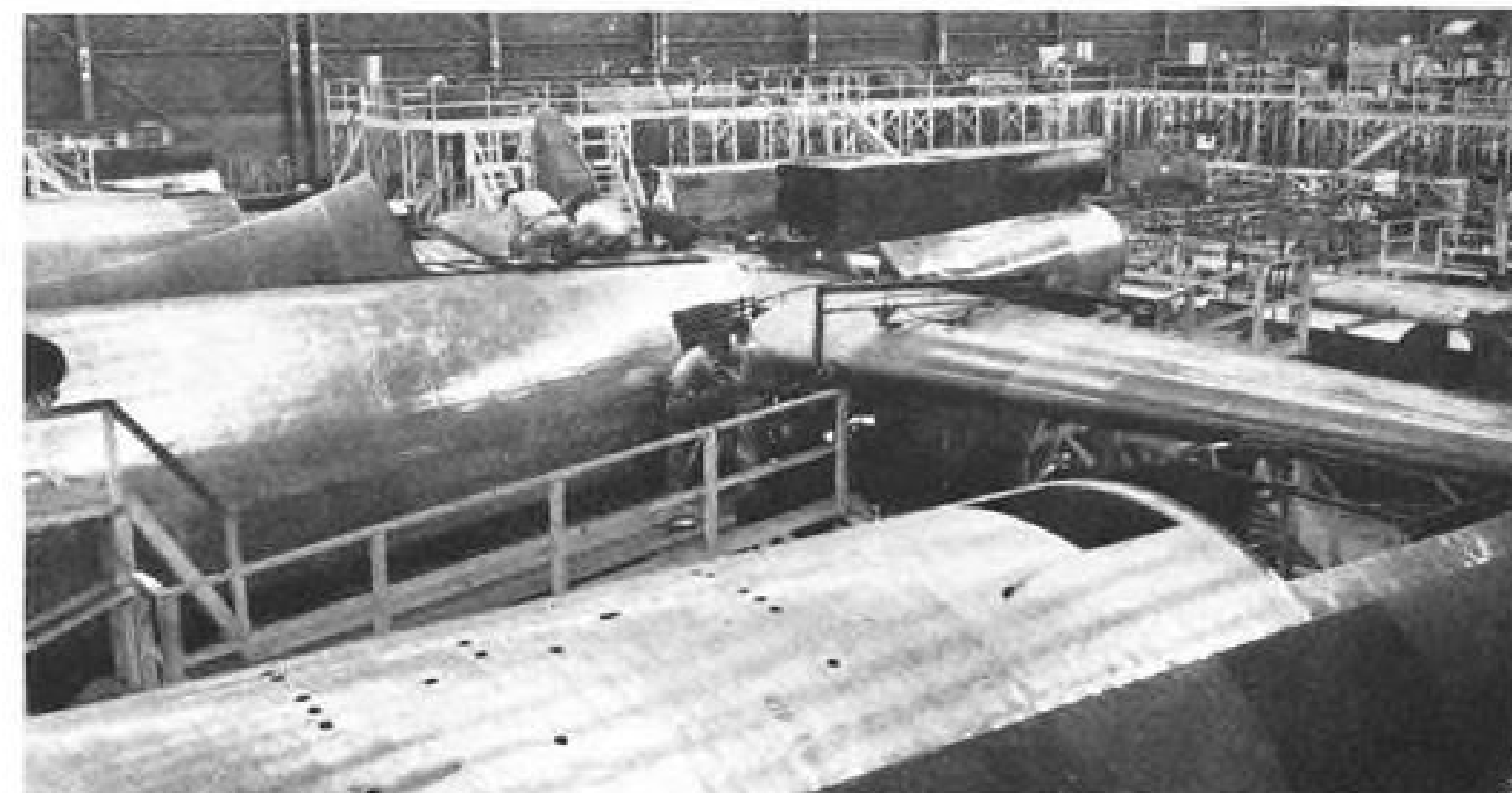
Mating horizontal stabilizer with tailcone and tail section. At this station (left, out of picture), aft bomb bay section is mated simultaneously to tail.
