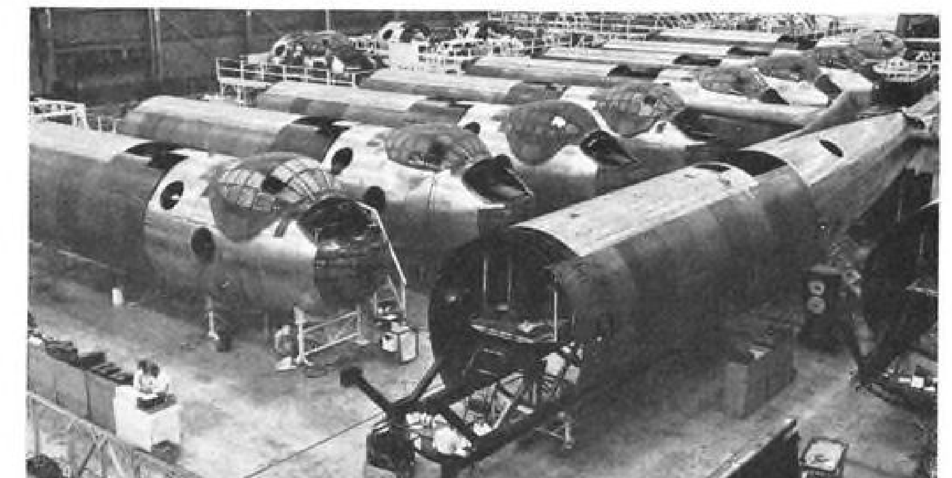
Nose-forward bomb bay primary line. In background, pilot enclosure is being installed. In foreground is aft bomb bay mated to tail. (Continued on page 37)
