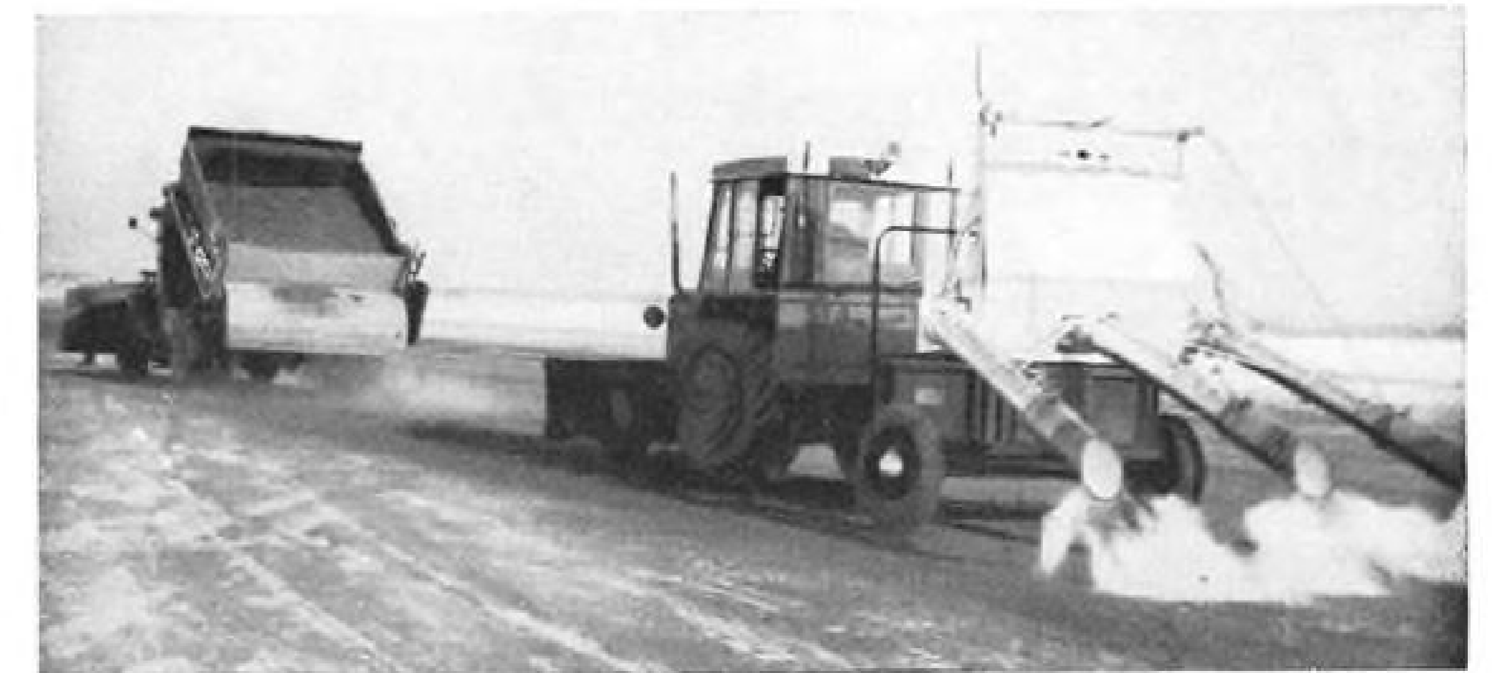
A sander followed by a three-jet weed burner conquered thick runway ice in recent tests at Minneapolis. The 2100-degree flame from the weed burner's nozzles fused the sand into the ice, providing good traction for plane landings and takeoffs.
