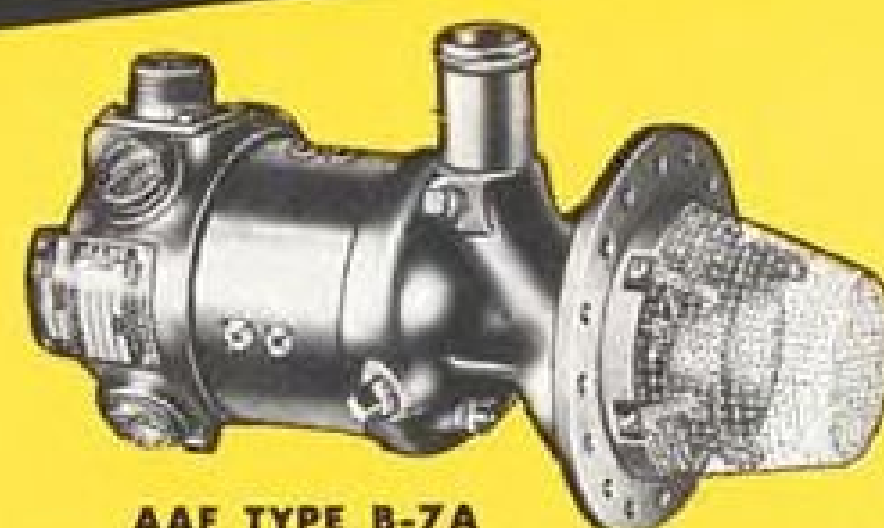
AAF TYPE B-7A "External" mounted—for reciprocating engine aircraft; capacity 19 psi at 500 gph (high speed)—10 psi at 500 gph (low speed).
