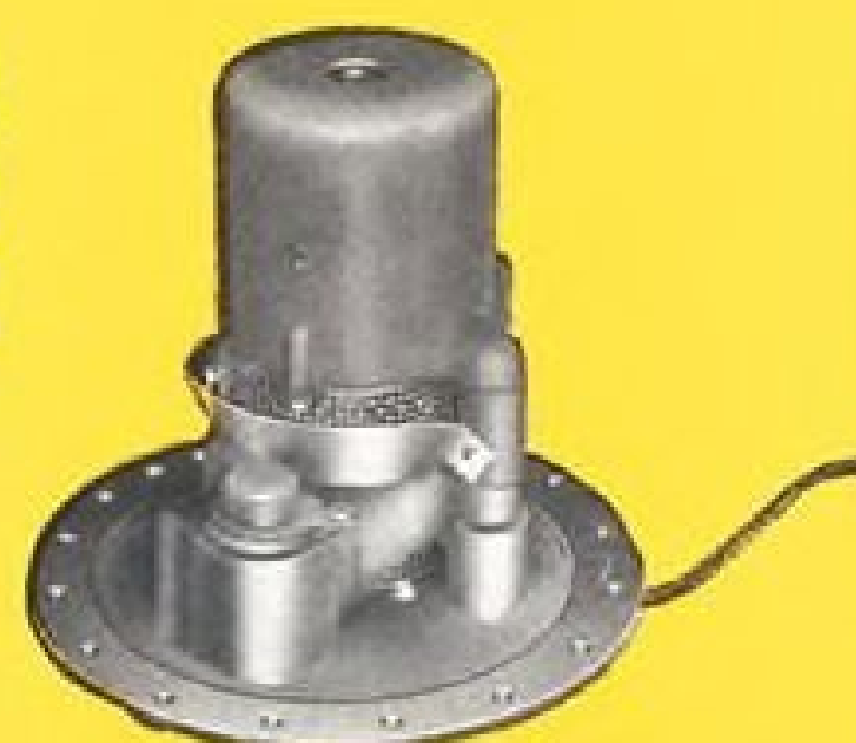
AAF TYPE B-22 "Submerged"—newly developed for military aircraft; uses 400 cycle 3-phase single speed 208 volt A.C. motor; rating 16 psi at 1000 gph.
