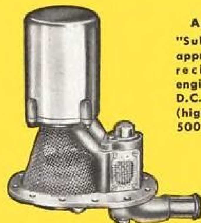
AAF TYPE B-7A "External" mounted—for reciprocating engine aircraft; capacity 19 psi at 500 gph (high speed)—10 psi at 500 gph (low speed).
