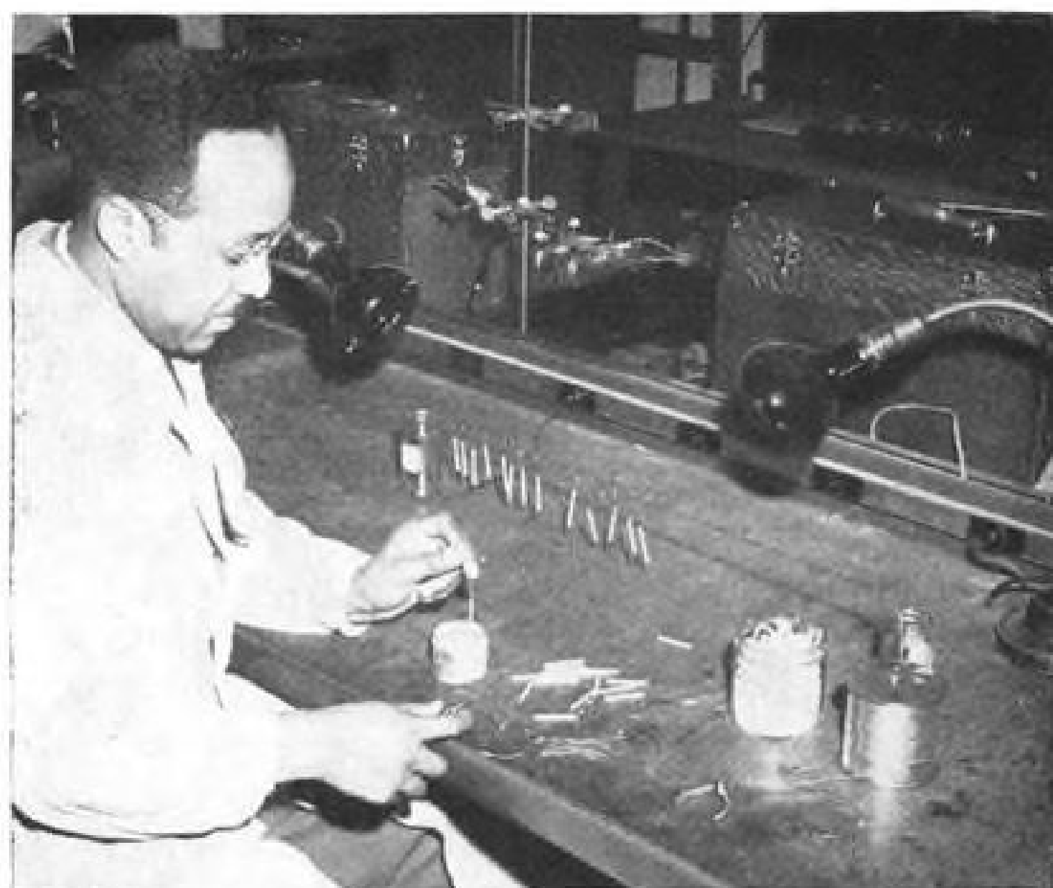
Special tubular capacitors, left, for use at high operating temperatures found in miniature assemblies are made by coating high-K titanate ceramic tubing with silver-
