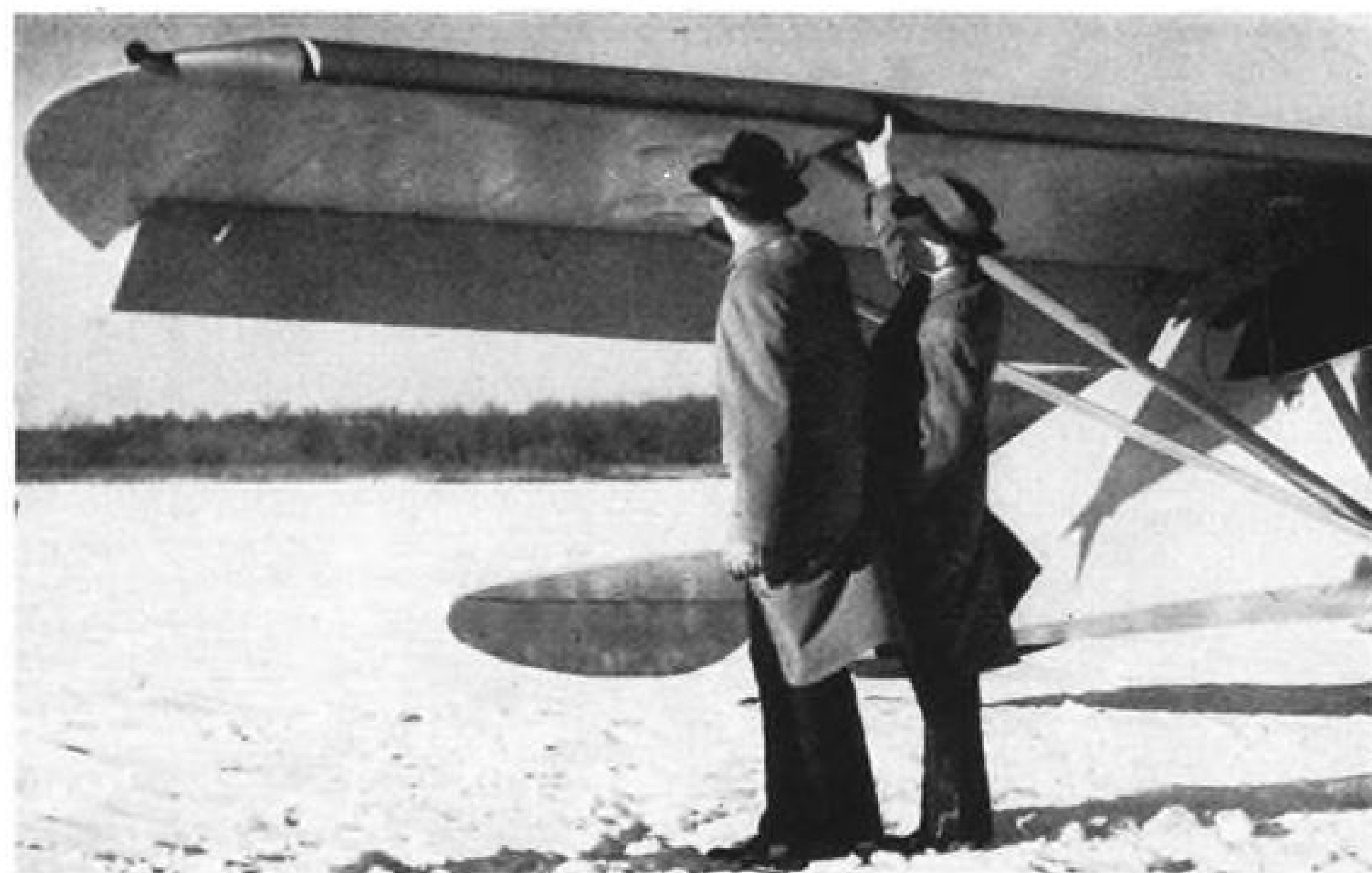
LEADING EDGE SLATS, aerodynamically actuated, contribute to plane's high-lift.
