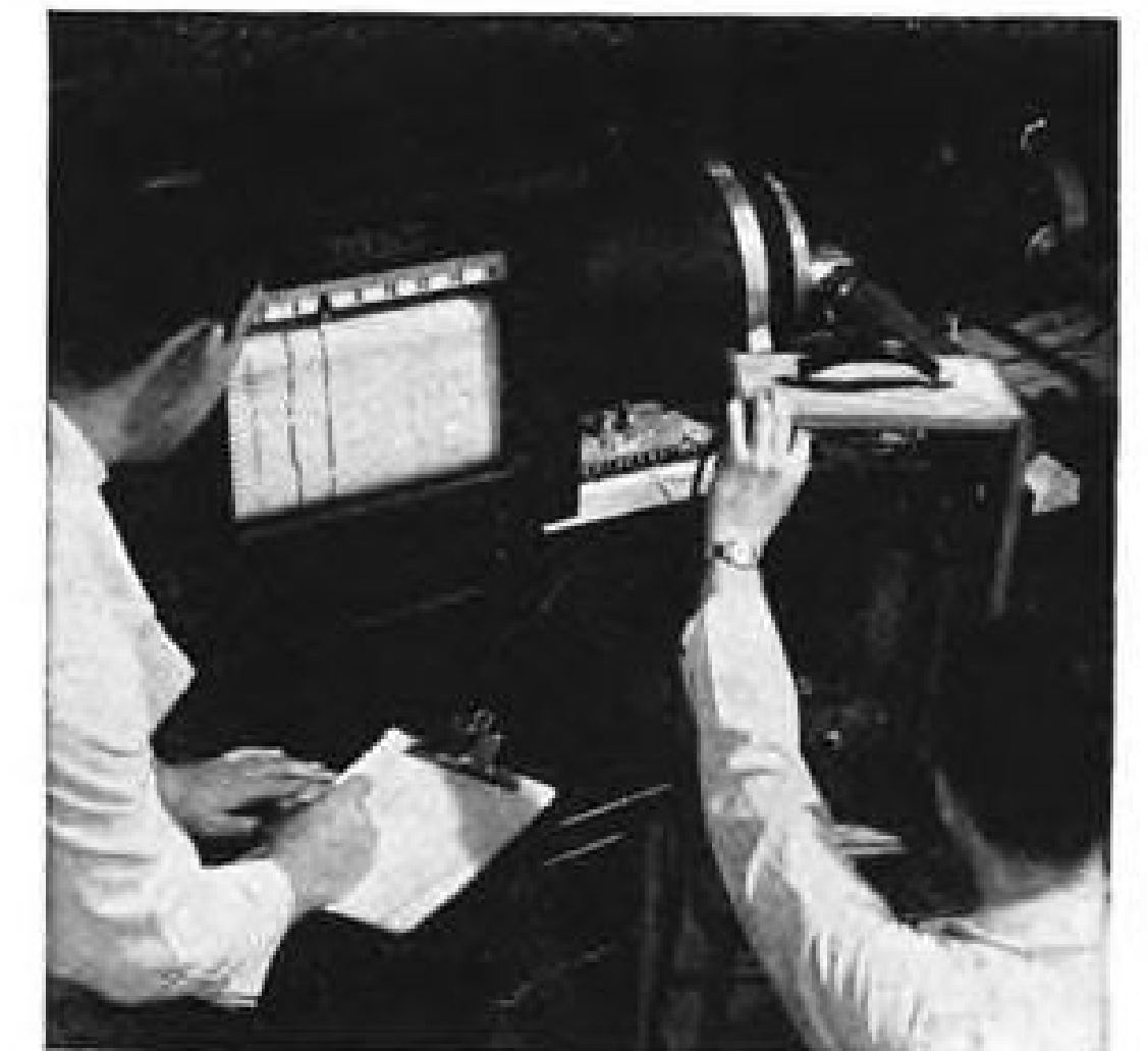
Temperatures taken continuously. Improved combustion efficiencies, lighter weight, longer life for Janitrol heaters result from such precise performance tests as this.
