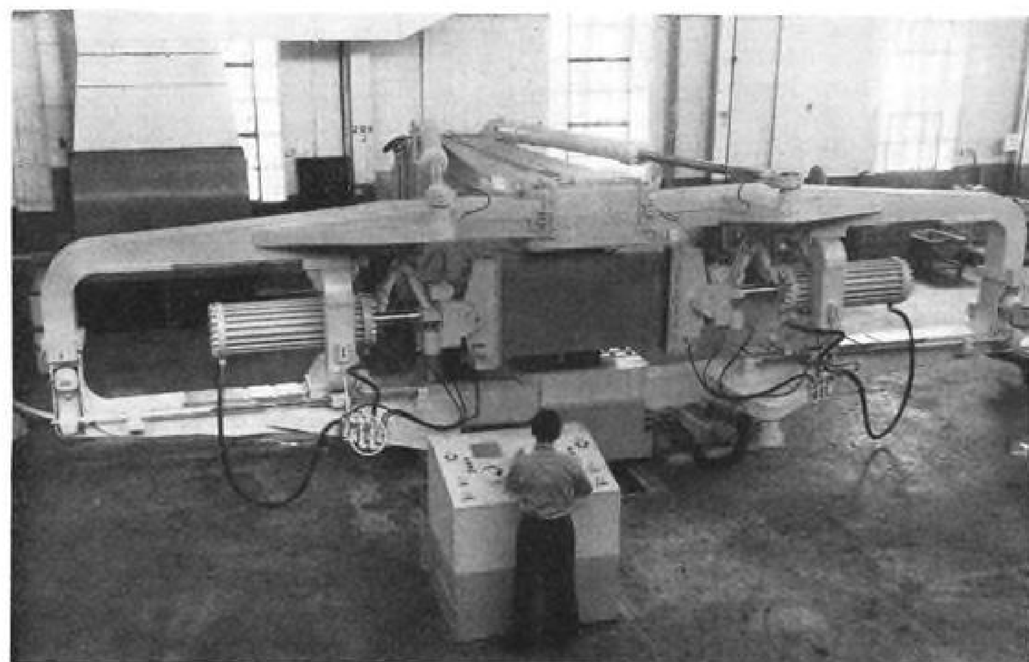
ALUMINUM SHEET is held in jaws of stretch press, pulled beyond normal limit and . . .
