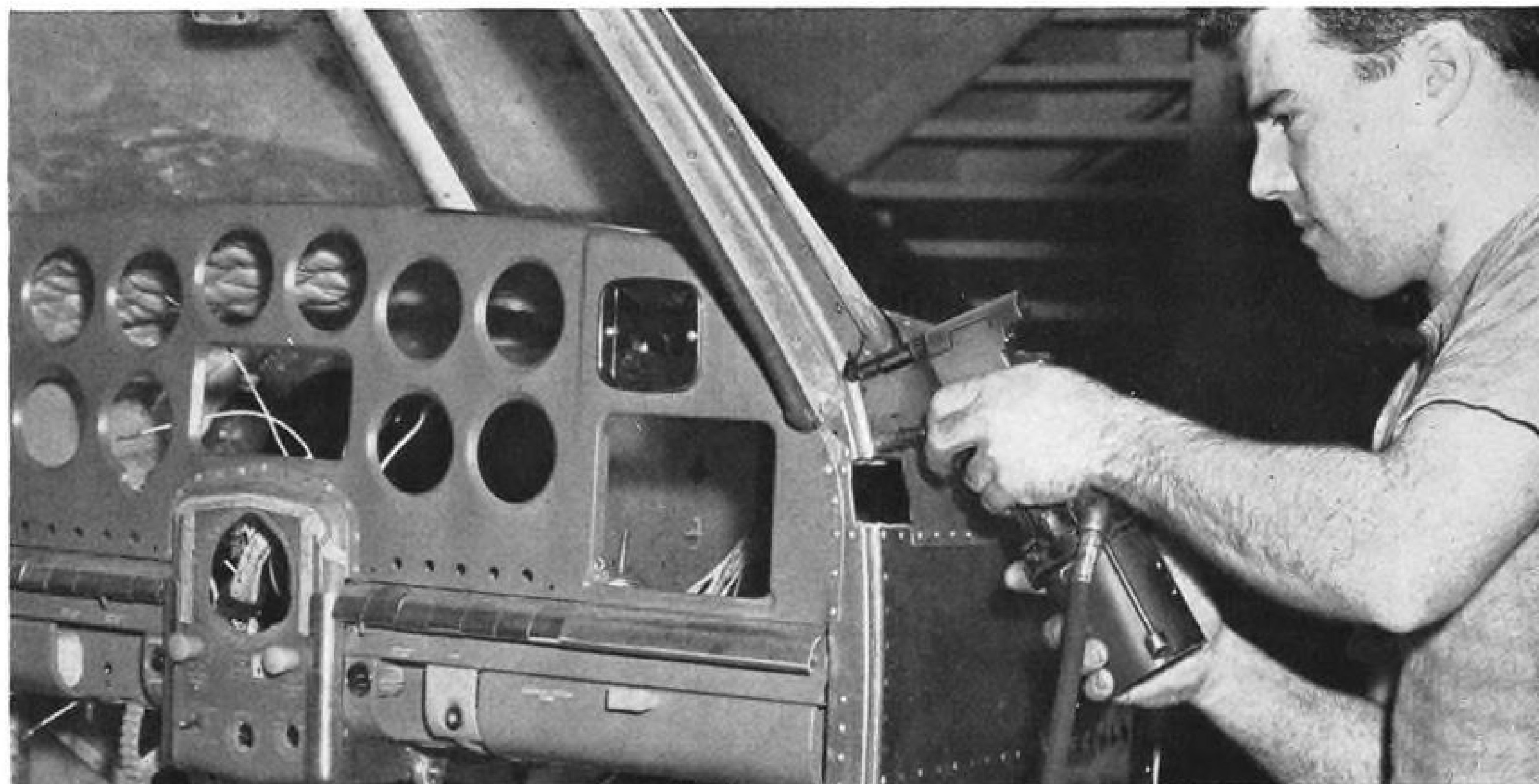
One man, working from one side of the job, replaces the two-man bucking team where Cherry Rivets and Tools speed assembly work.
