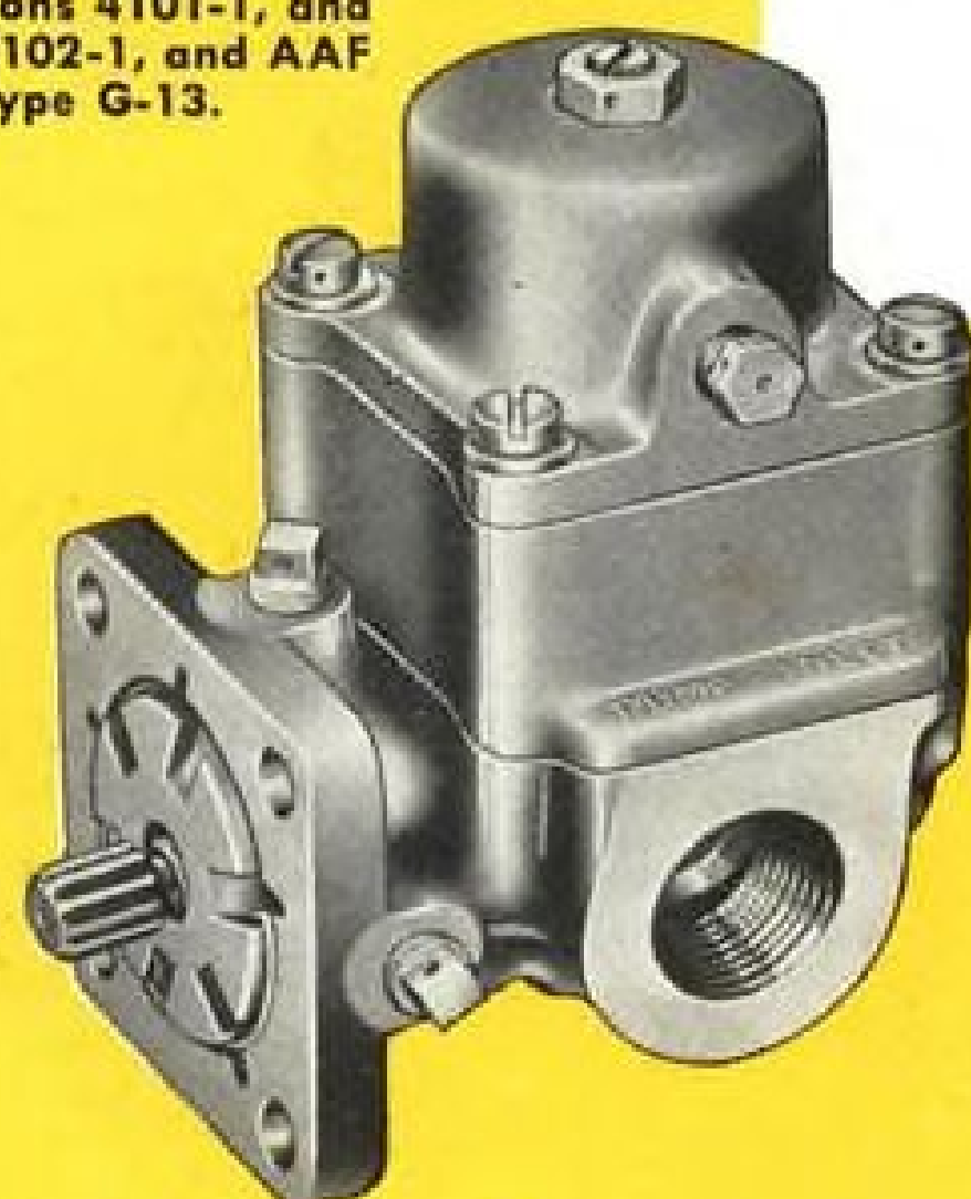
Engine-driven fuel pump for light aircraft and helicopters. Rating—85 gph at 2500 rpm.
