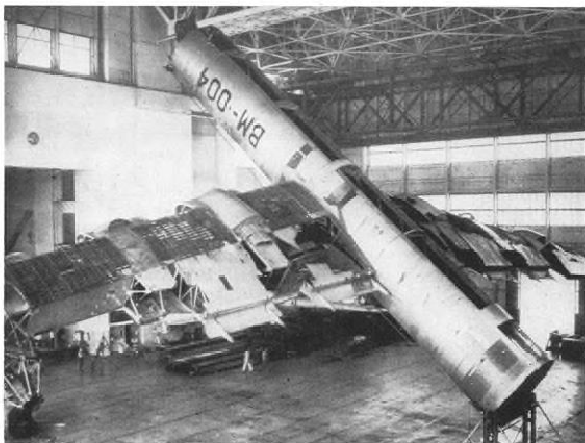
B-36 ON RACK: While Washington prepares to look into procurement of B-36, Wright Field is completing static tests on first production model of the bomber.
