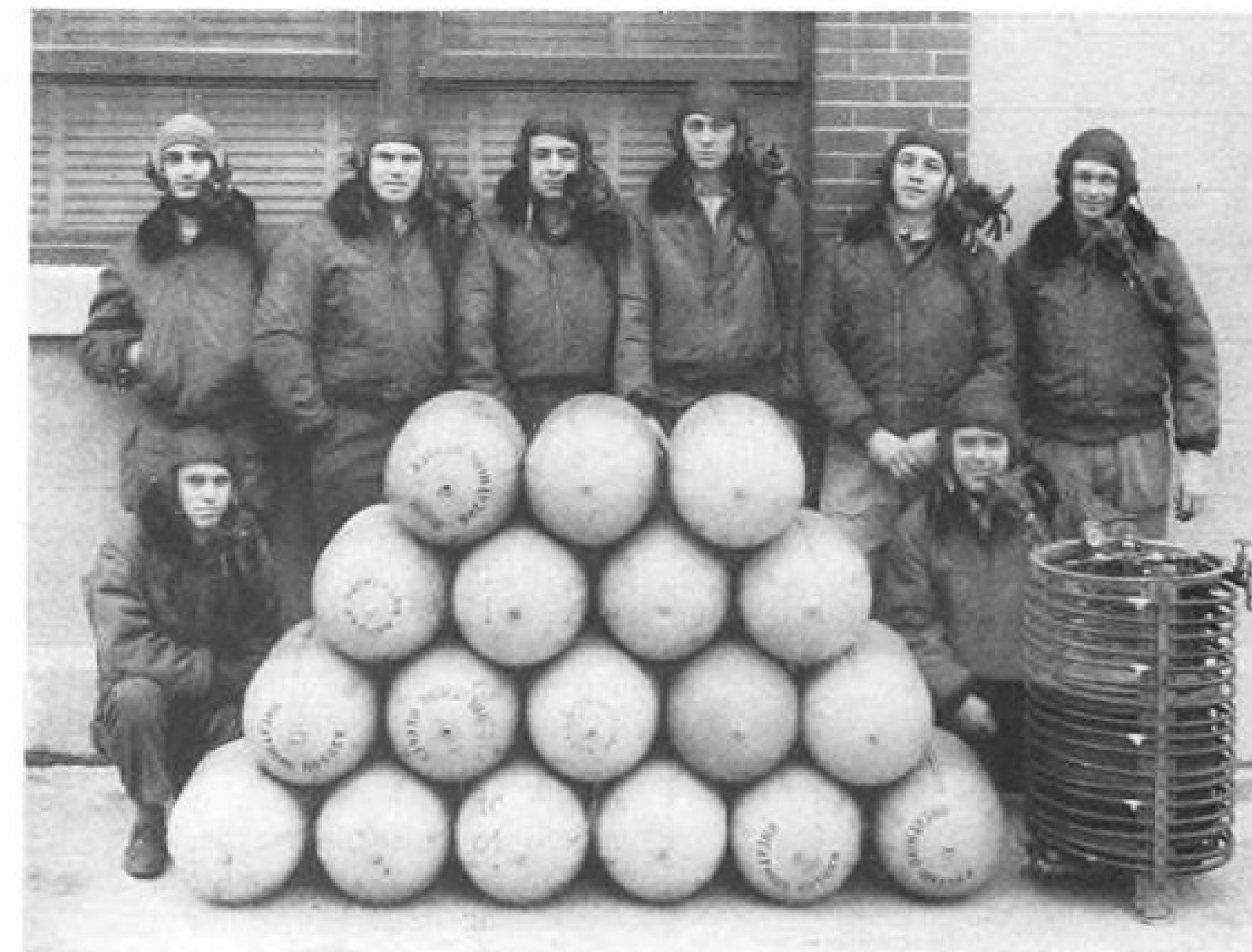
OLD vs. NEW: Left photo shows large pile of gaseous oxygen supply tanks formerly required for B-17 crew in contrast to compact Bendix version of liquid oxygen converter seen alongside. Original converter developed by National Bureau of Standards is shown at right.
