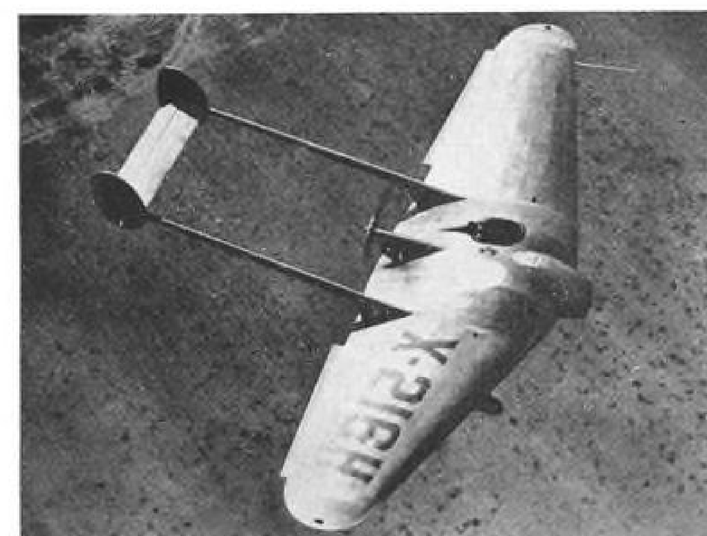
20 YEARS AGO: First Flying Wing ever built by Jack Northrop is shown here on its maiden flight, in 1929. It had a wing span of 30 feet, six inches. Successfully flown many times, it provided valuable research information and was a big step on the way to today's huge Northrop Flying Wing.
