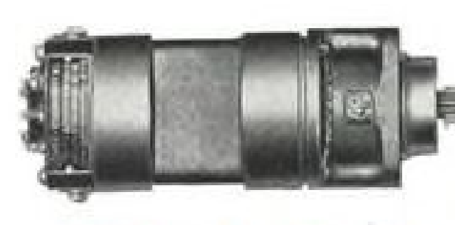
PILOT SEAT ACTUATOR MOTOR AND CLUTCH
