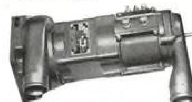
EXPLOSION-PROOF MOTOR EQUIPPED WITH AIR DUCTS
