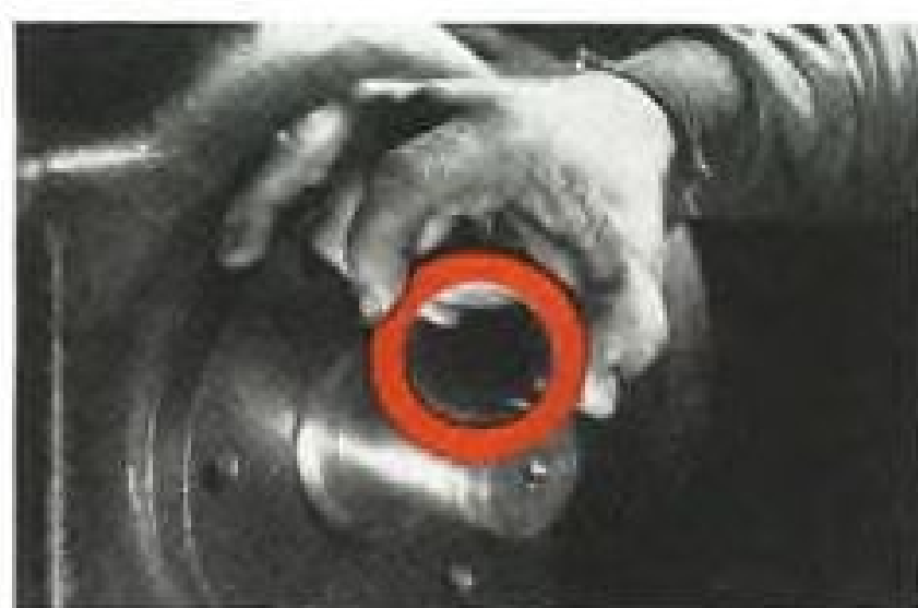
FOR THRUST BEARING adjustment of pump. Peelable shim is valuable for takeup of wear after service, reducing "down time" for maintenance.
