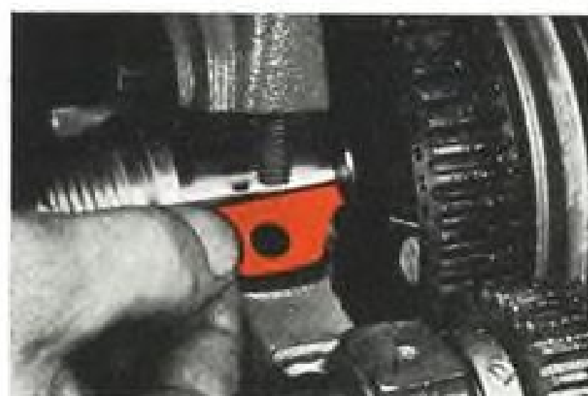
FOR SPLIT BEARING of lathe headstock spindle. Even after peeling, shim is always uniform in gauge, with a hard, clean and smooth surface.
