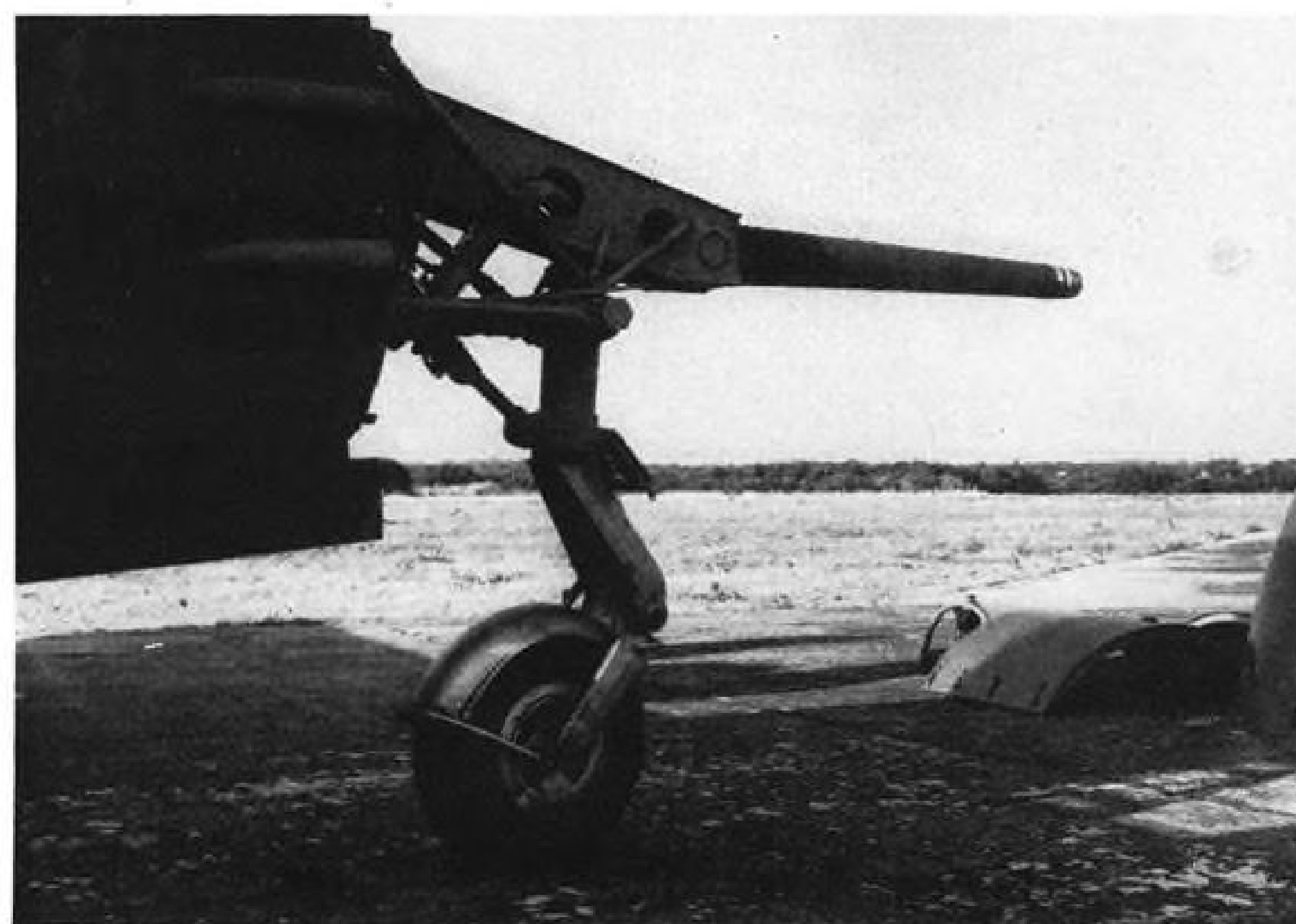
REFUELING PROBE on Meteor, nose cowling removed, showing hose connection to tanks.
