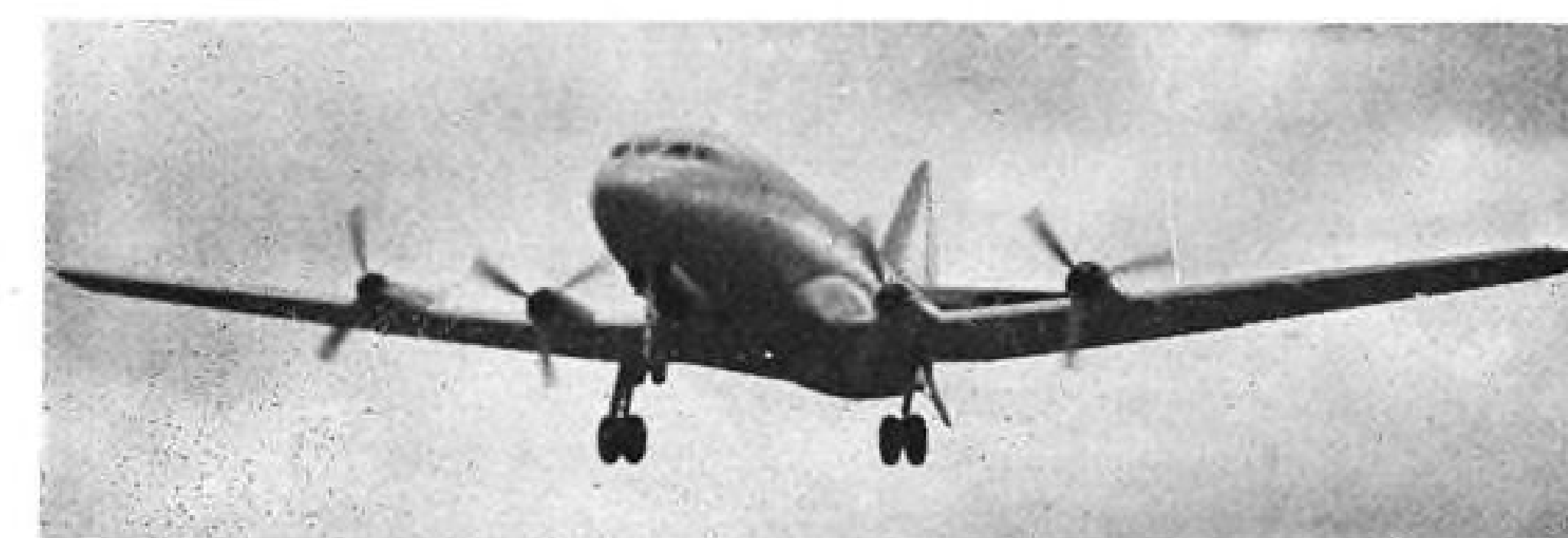
ARMSTRONG WHITWORTH 31-passenger Apollo with four Mambas. Gross weight of the pressurized craft is 39,500 lb. and it is designed to cruise at 305 mph. at 20,000 ft. Total freight capacity is given as 430 cu. ft.
