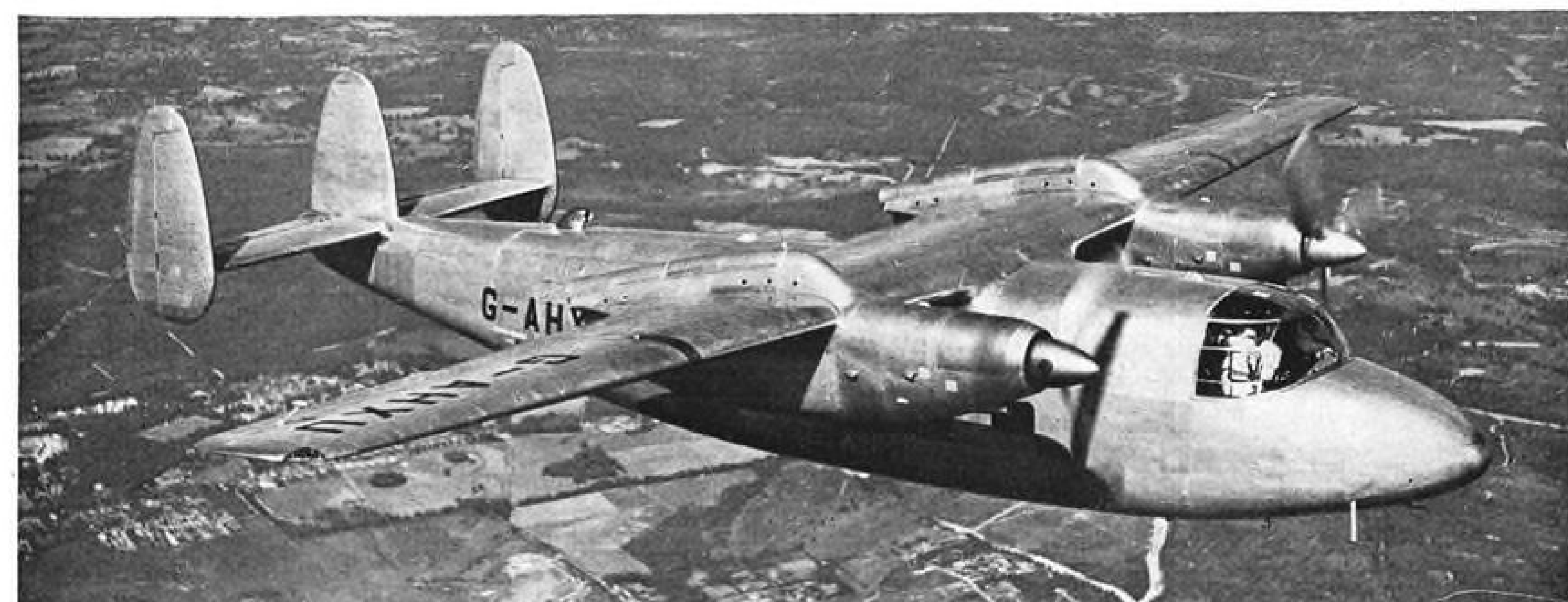
MAMBA-MARATHON'S unattractive jet-pipe fairings are displayed above otherwise very clean engine nacelles. Installation apparently was dictated by wings being too thin to enclose the pipes. Third British turboprop liner to fly, 22-seat Mamba-Marathon is smaller than . . .
