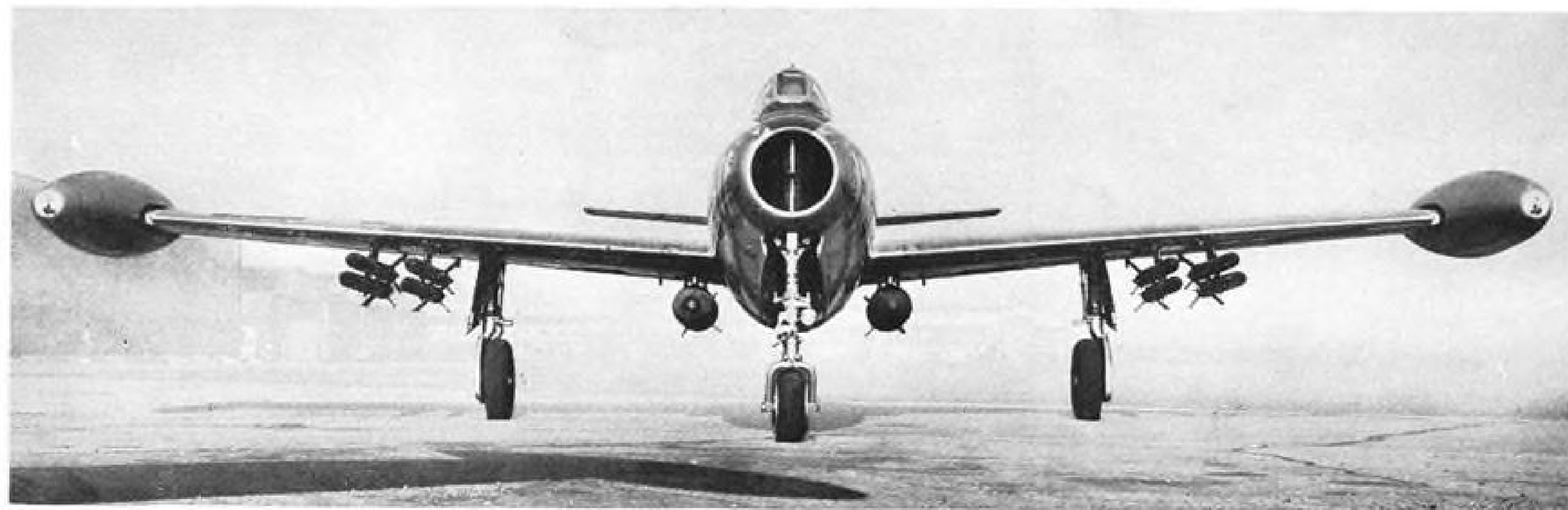
Pylons carrying bombs 11 in. below wings remedied trim difficulty. Rockets have been fired at airplane speeds up to 550 mph.
