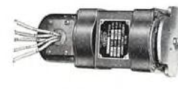
DRIVE MOTOR FOR RADAR SCANNER 400 watts output continuous. 12,000 R. P. M. reversible. 600 watts peak load. Weight, 4-1/2 lbs.
