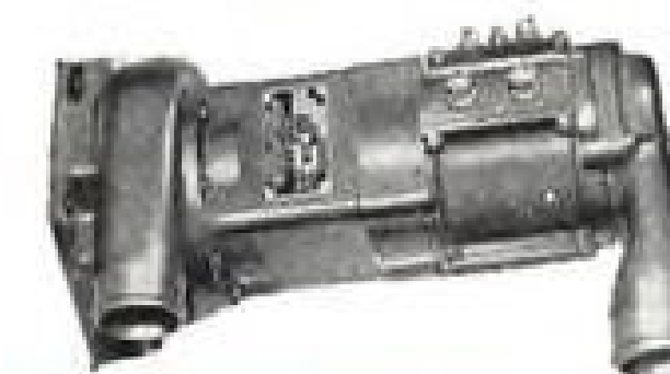
EXPLOSION-PROOF MOTOR EQUIPPED WITH AIR DUCTS Intake and exhaust ducts for external air cooling. Continuous rating of 4 H.P. with a ram of 12-inch head of water pressure; 2-1/2 H.P. when drawing its own air for cooling. Intermittent peak output, 7 H.P. 27 volts, 9000 R.P.M. Weight, 19-1/4 lbs.
