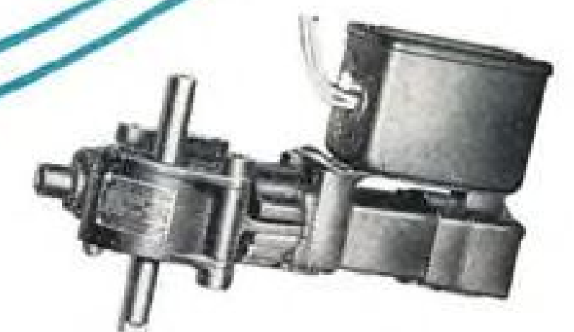
CANOPY ACTUATOR FOR JET FIGHTER Rotary type, with manual overdrive and radio noise filter. 81 R.P.M. on the double end output shaft. 150 inch-lbs. torque. Weight, 6-1/4 lbs.
