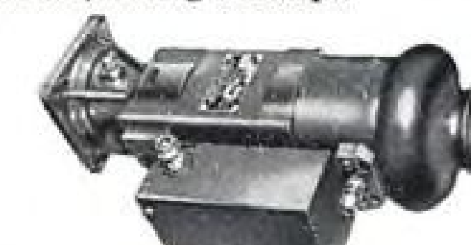
HYDRAULIC PUMP DRIVE MOTOR Open through ventilated for continuous duty. 3-3/4 H. P. continuous. Equipped with radio noise filter and integral gear reduction... Weight, 23-3/4 lbs.
