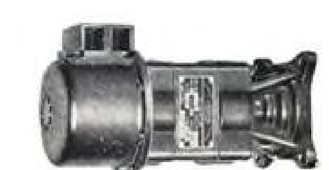
AILERON BOOSTER MOTOR Open through ventilated for continuous duty operation. Integral gear reduction. Weight, 12 lbs. 2 H. P. continuous rating.
