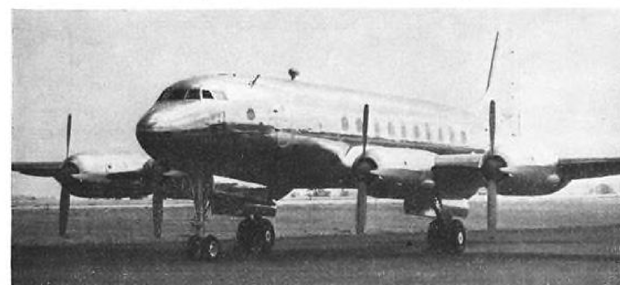
. . . FOUR THESEUS engines which total 9800 hp. for takeoff.
