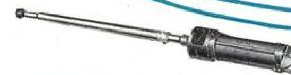
STABILIZER ACTUATOR, Linear Type Motor inline with screw. Magnetic clutch. Radio noise suppressors. Travel limit switches. Weight, 14 lbs. Normal load, 2500 lbs. Rate of travel, half-inch per second.
