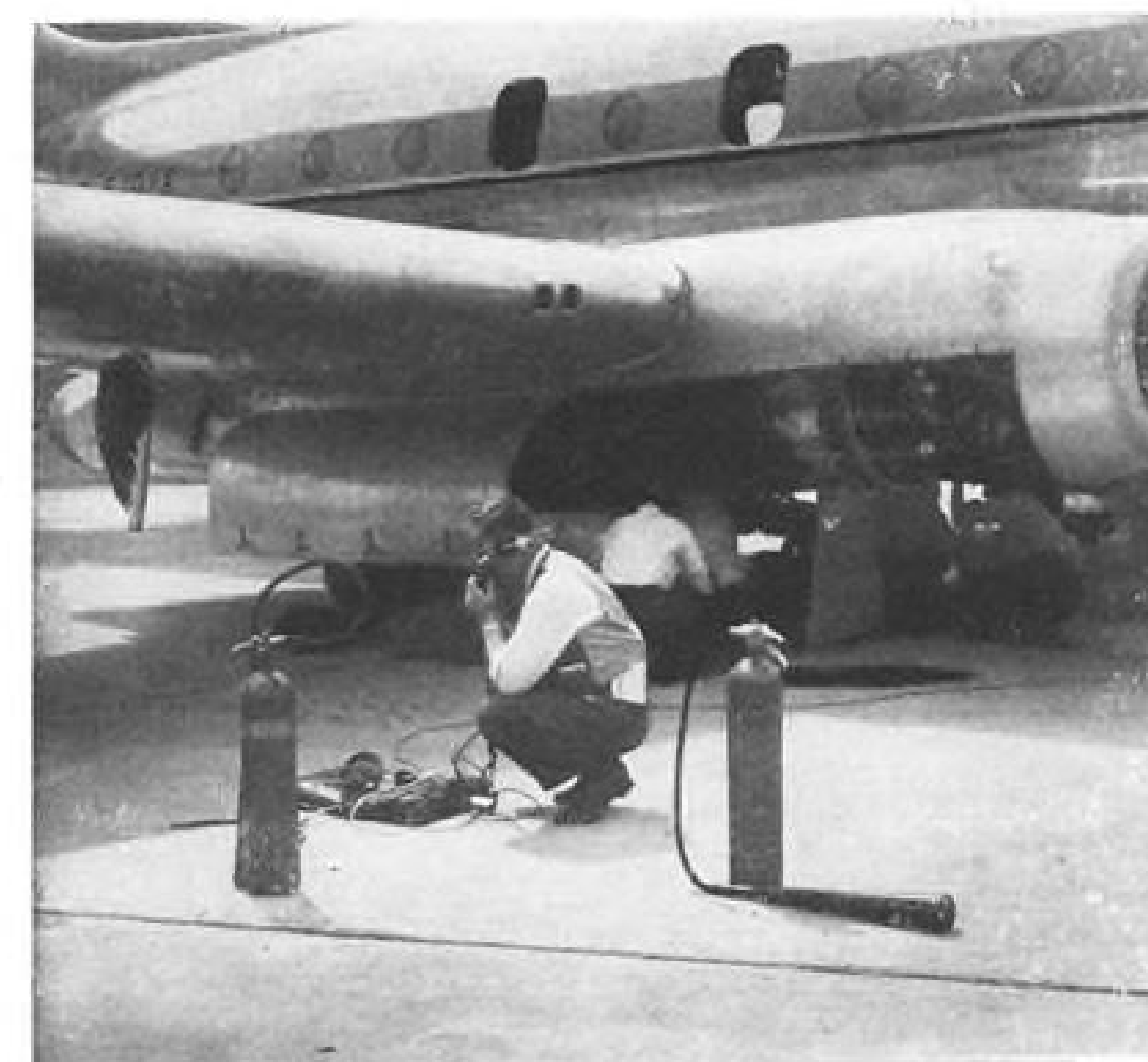
LOW NACELLE, large panels make maintenance easy, and . . .
