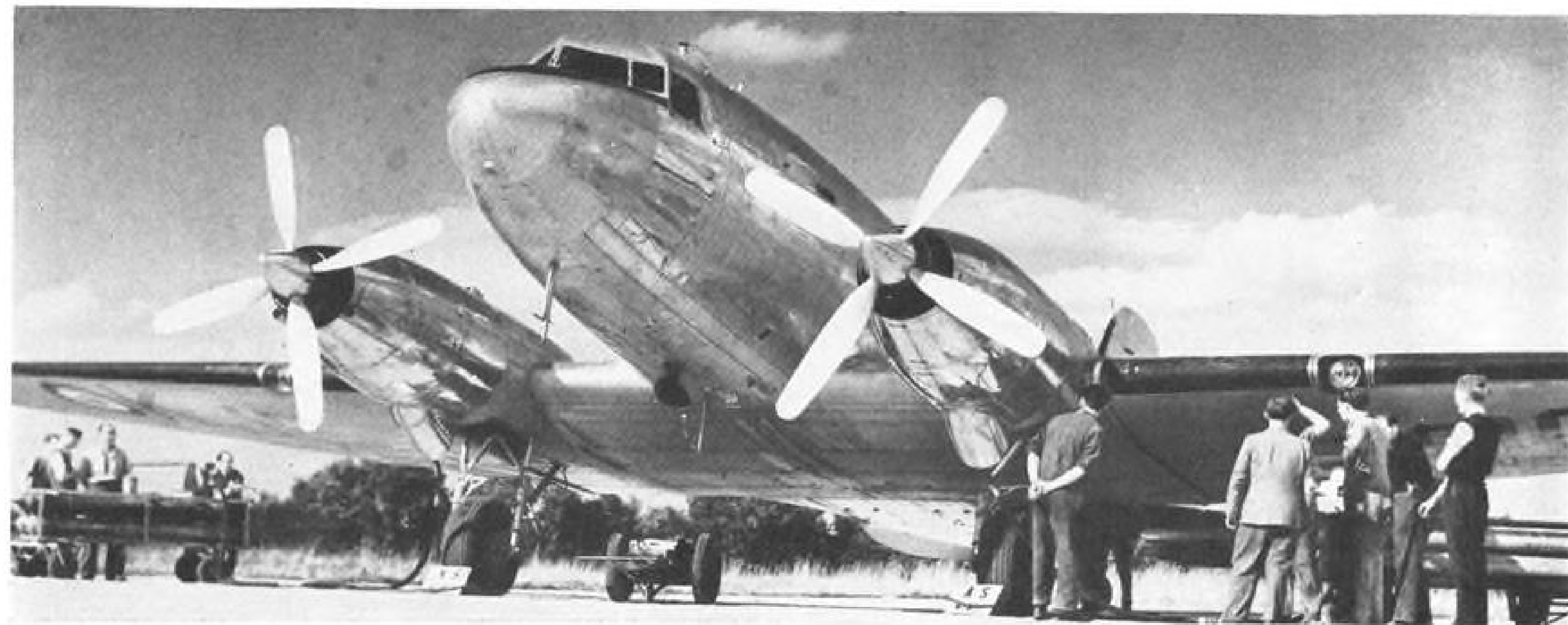
MAMBA-POWERED DC-3 conversion of Armstrong Siddeley retains the basic Douglas airframe, but offers great advantages in . . .
