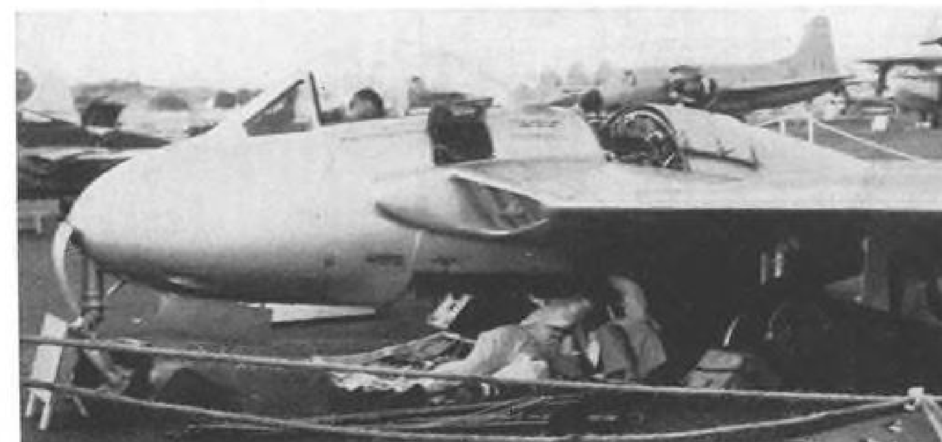
VENOM: Mechanics have easy access to innards of new DH fighter's engine, instruments and armament. Thin airfoil is fitted.
