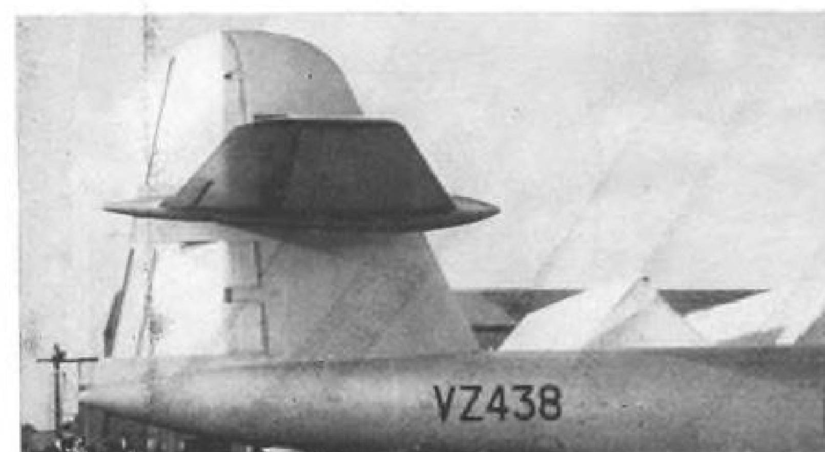
METEOR: New tail on Mk. VII fighter to raise critical Mach number on this Gloster.
