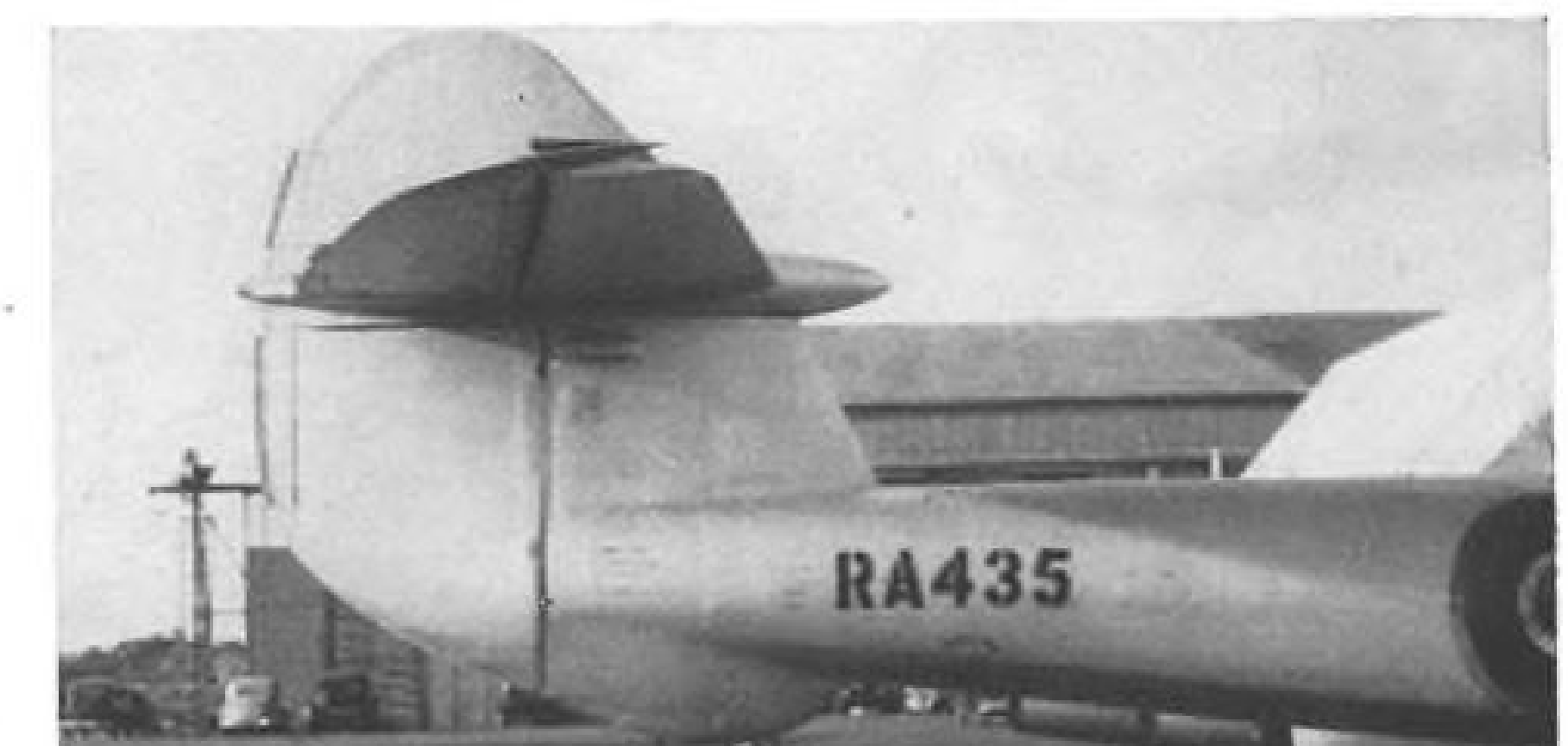
Normal tail on Mk. IV Meteor clearly points up extent of modification made on Mk. VIII shown in photo at left.
