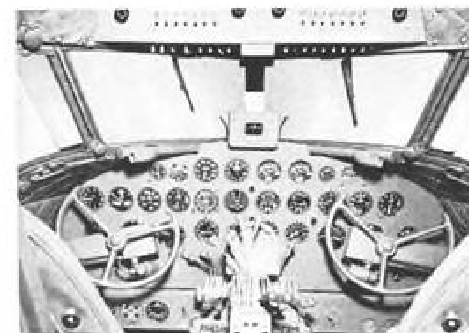
Instrument panel custom-designed and built in a single piece.
