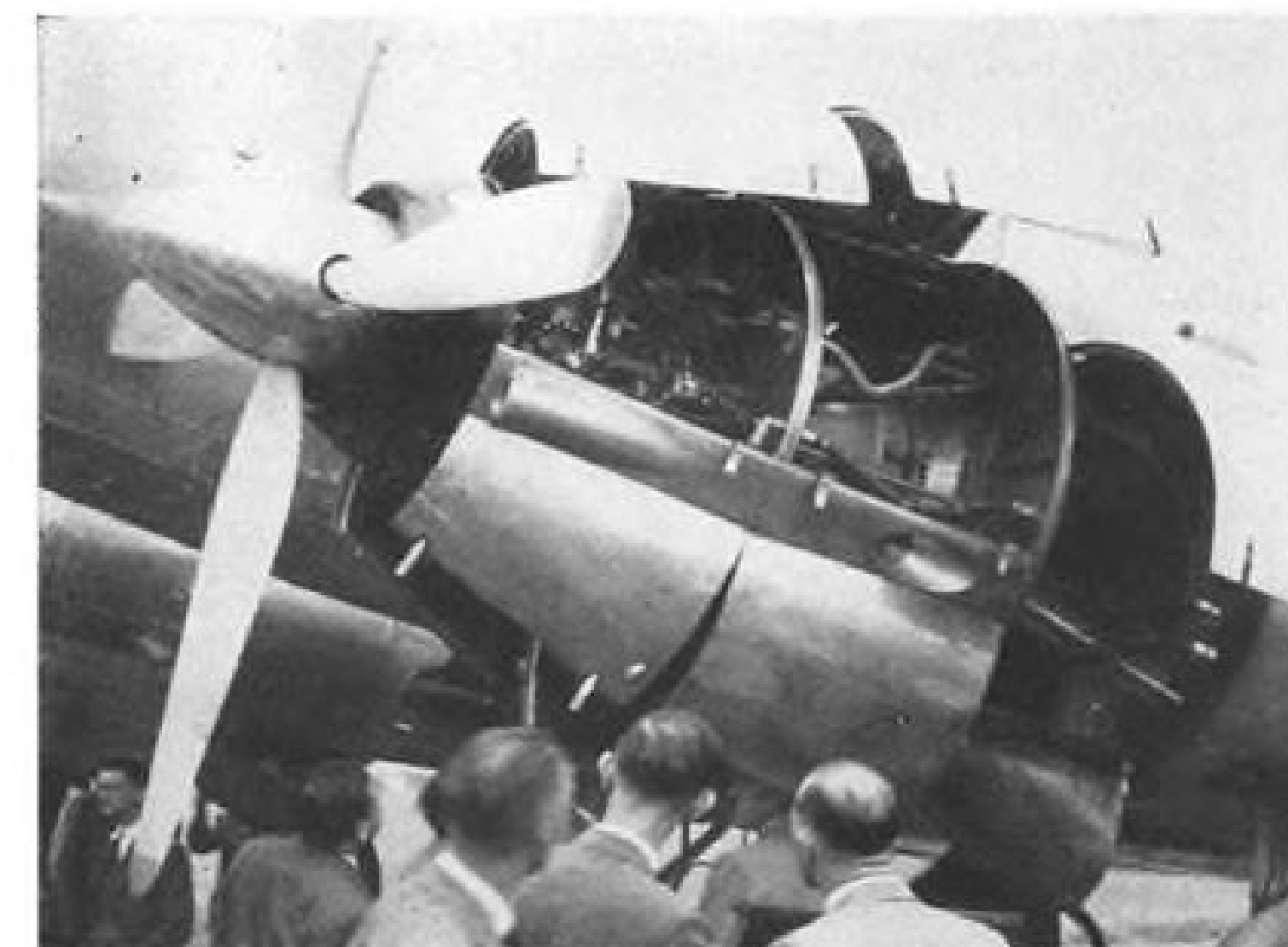
ENGINE ACCESSIBILITY is improved in the Mamba DC-3.
