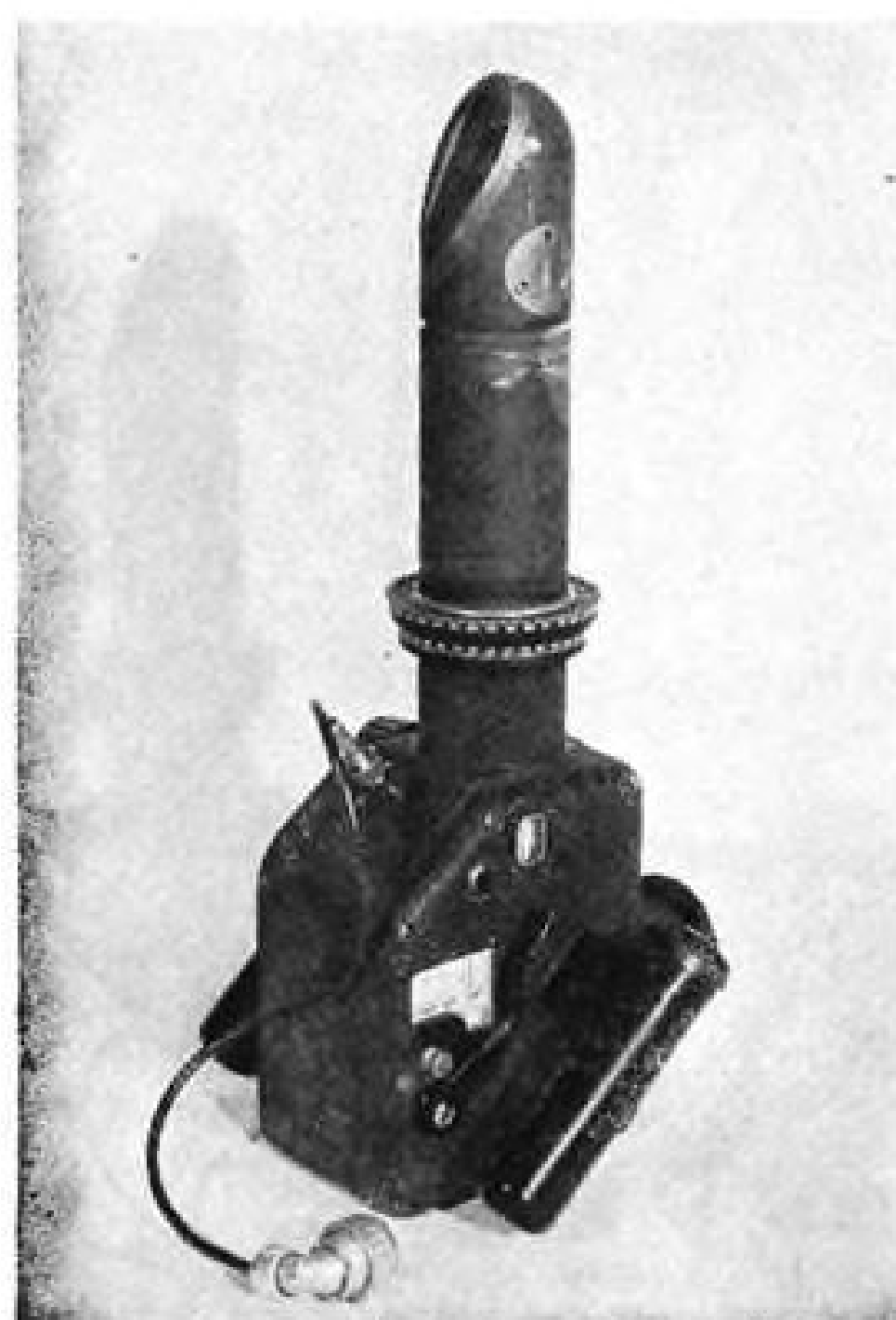
BRITISH: Hughes sextant (left) uses bubble horizon with different lighting for day and night operation. Tube similarly fits mount (right), projects about 3 in. above skin of aircraft. Cabin pressure sealing plate is seen in mid-position.
