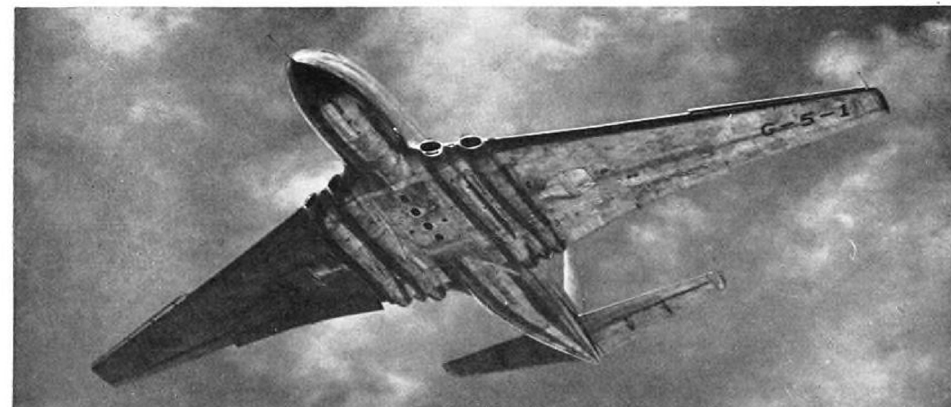
WITH LEADING EDGE SLATS fully open and flaps partly down, the Comet displays wing profile during takeoff. Meanwhile . .
