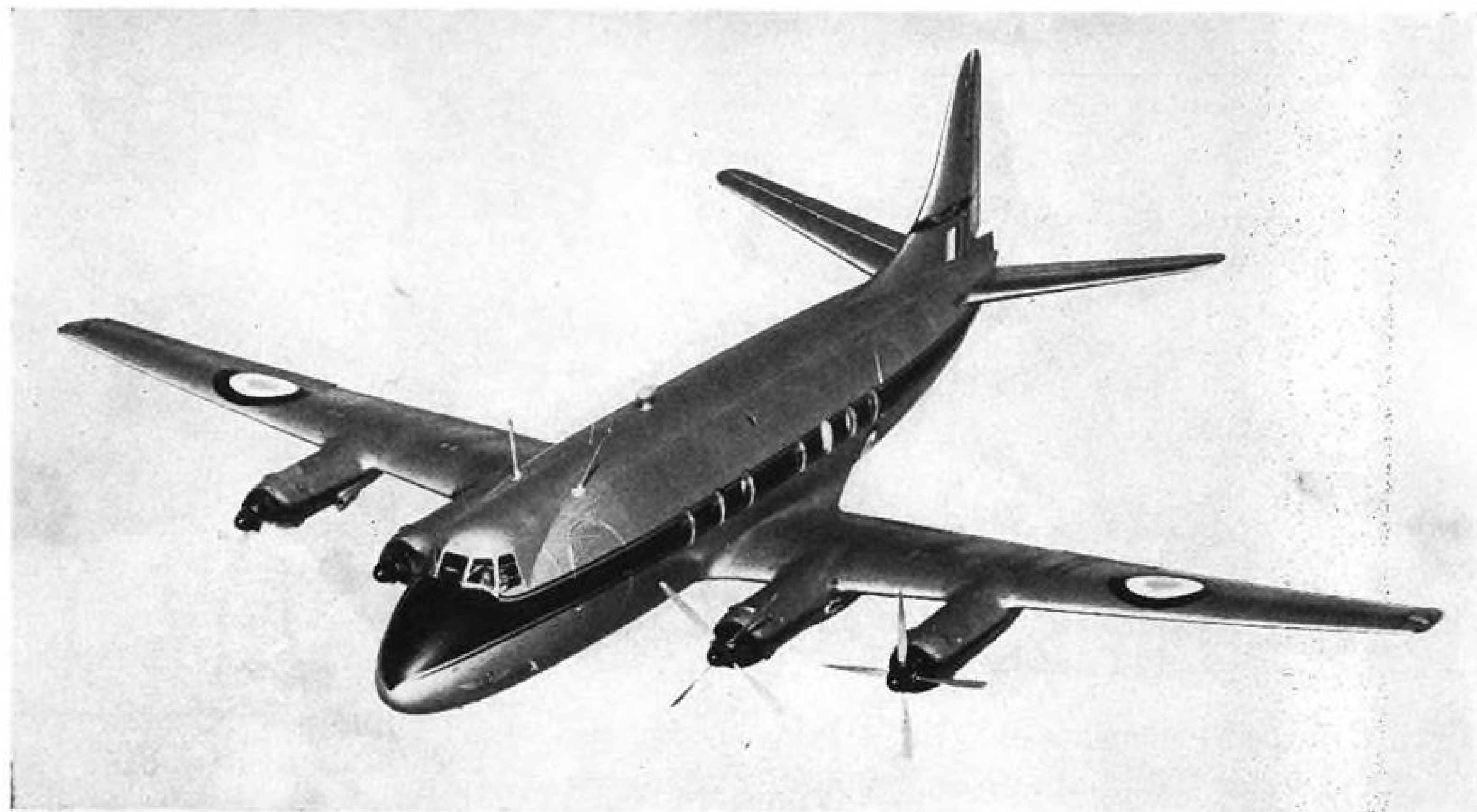
TWO-ENGINE CONTROL of Viscount, both props on same side feathered, is indicated by amount of rudder needed to fly straight.
