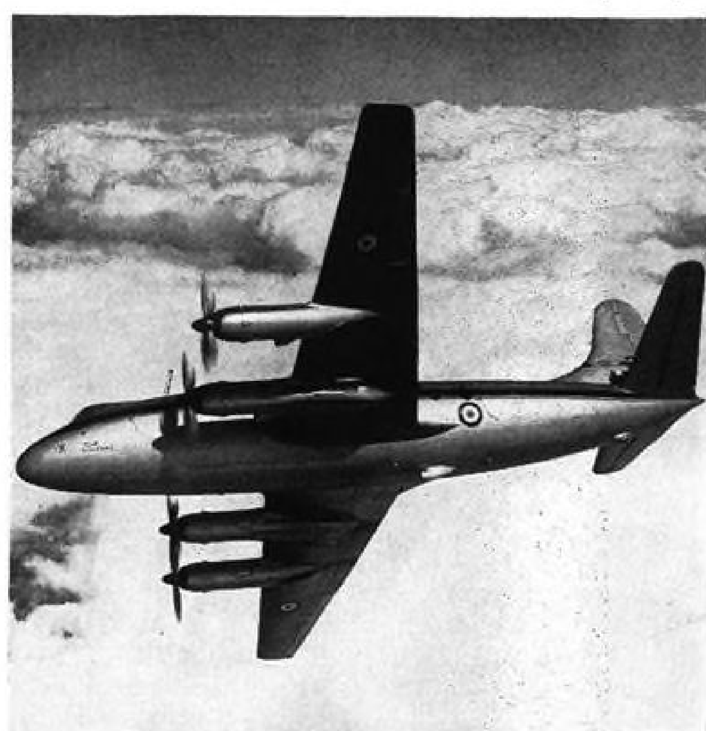
LONG NACELLES of Viscount have tailpipe at base.
