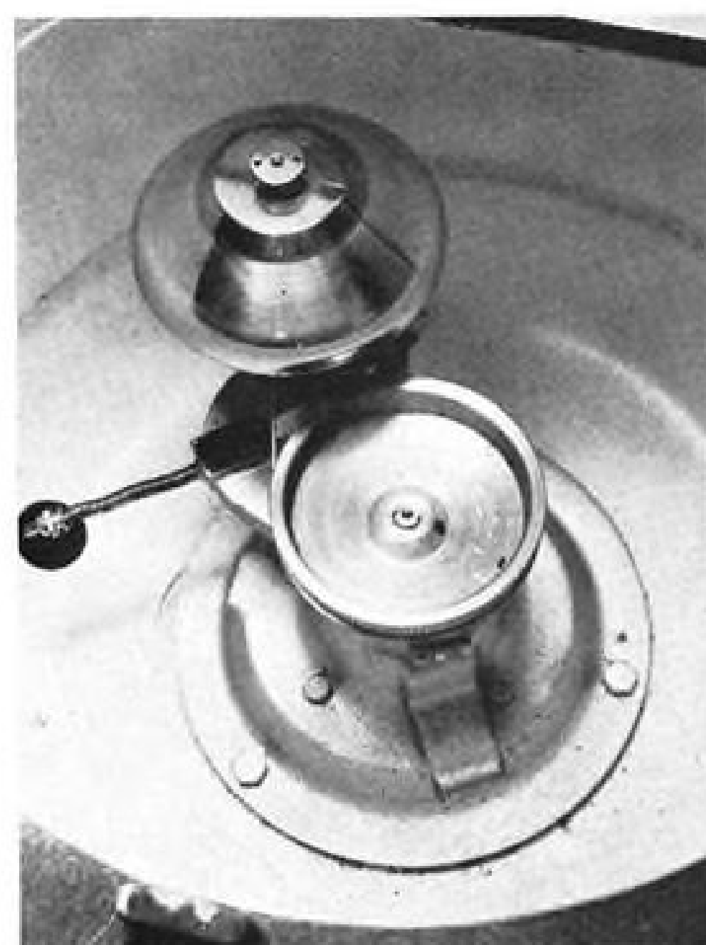
The motor-driven centrifuge is used to produce continuous acceleration of thousands of Gs for tube test. This procedure gives good overall quality check for ruggedness.
