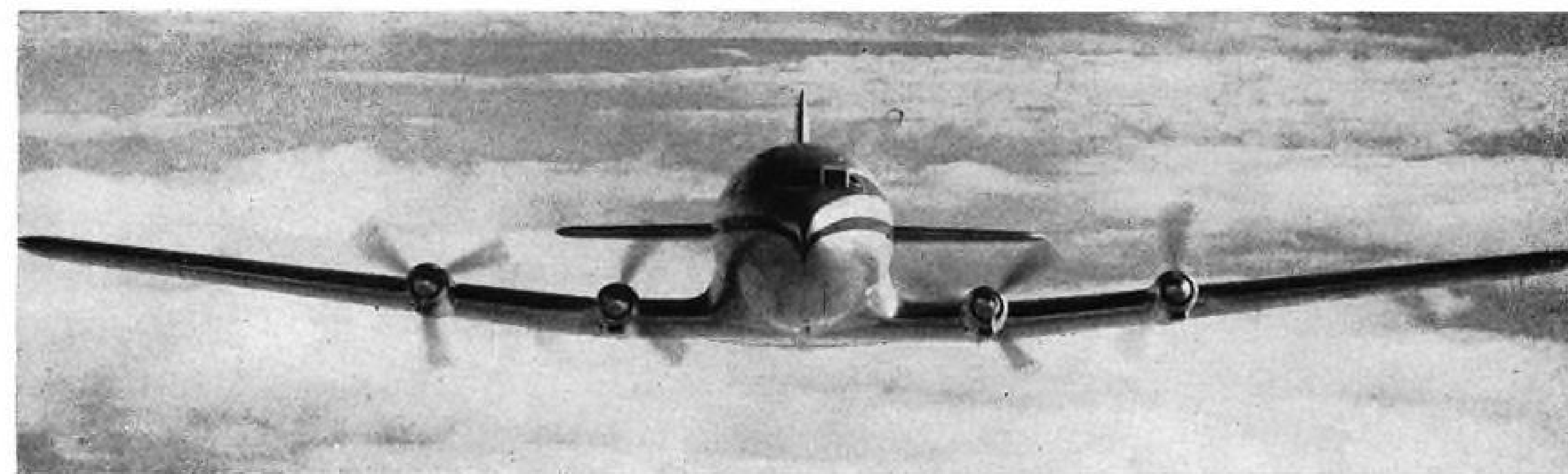
LOW DRAG design made possible by turboprop engines is apparent in head-on view of Apollo, with nacelles hardly thicker than wing.
