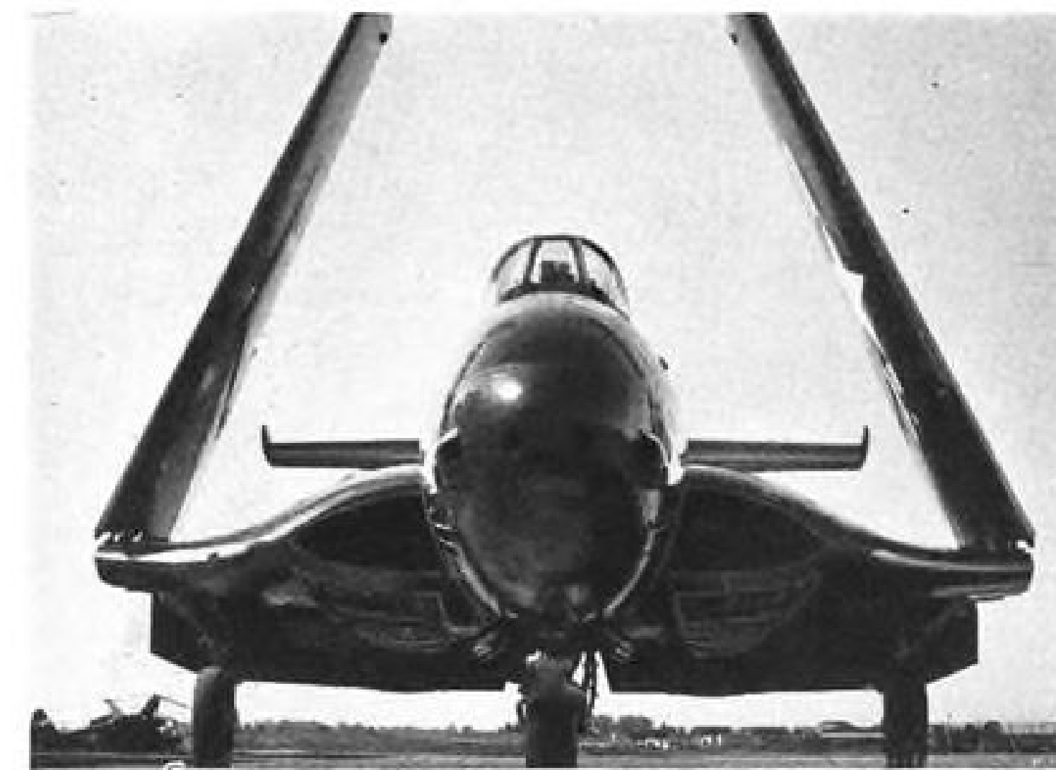
ACCESS DOORS on underside of wing aid in engine removal.
