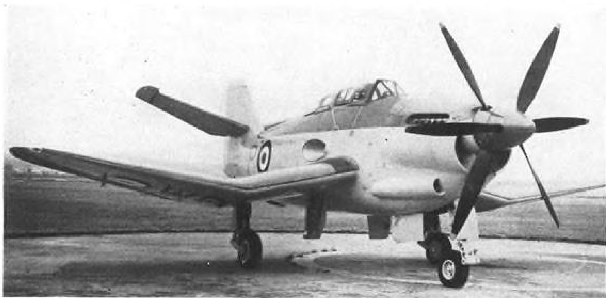
BLACKBURN Y.A.5 built to same specification. Note steep dihedral of Y.A.5's stabilizer.
