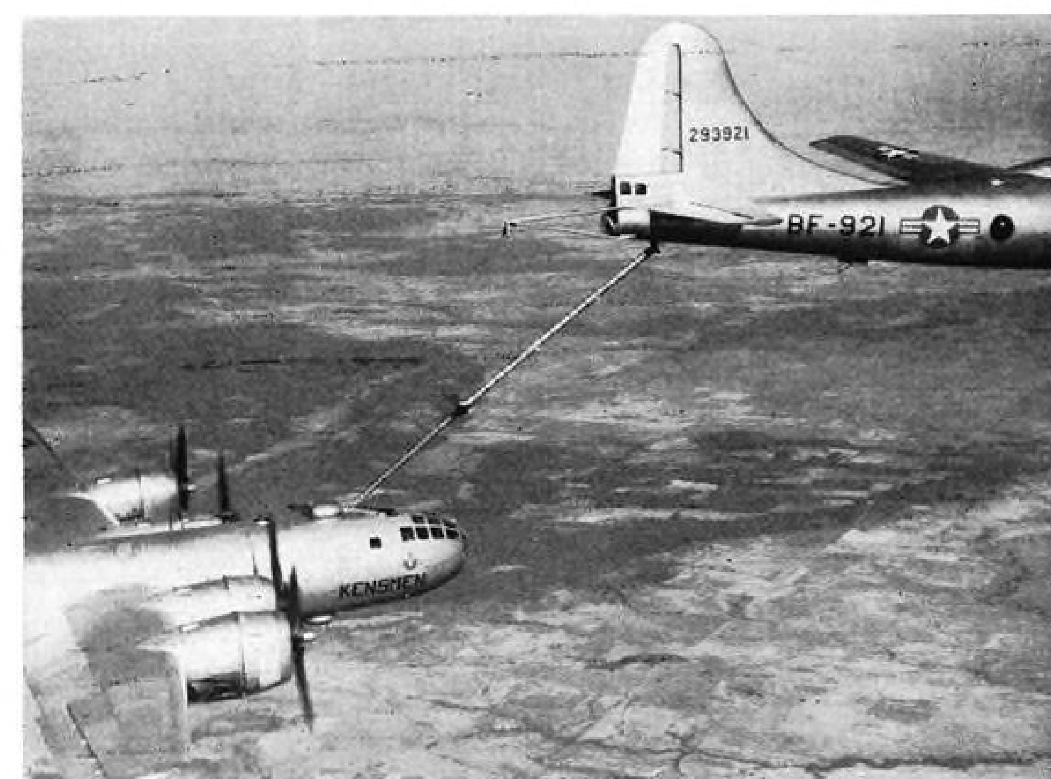
TANKER steers tube to socket in receiver plane and the transfer of fuel can begin.
