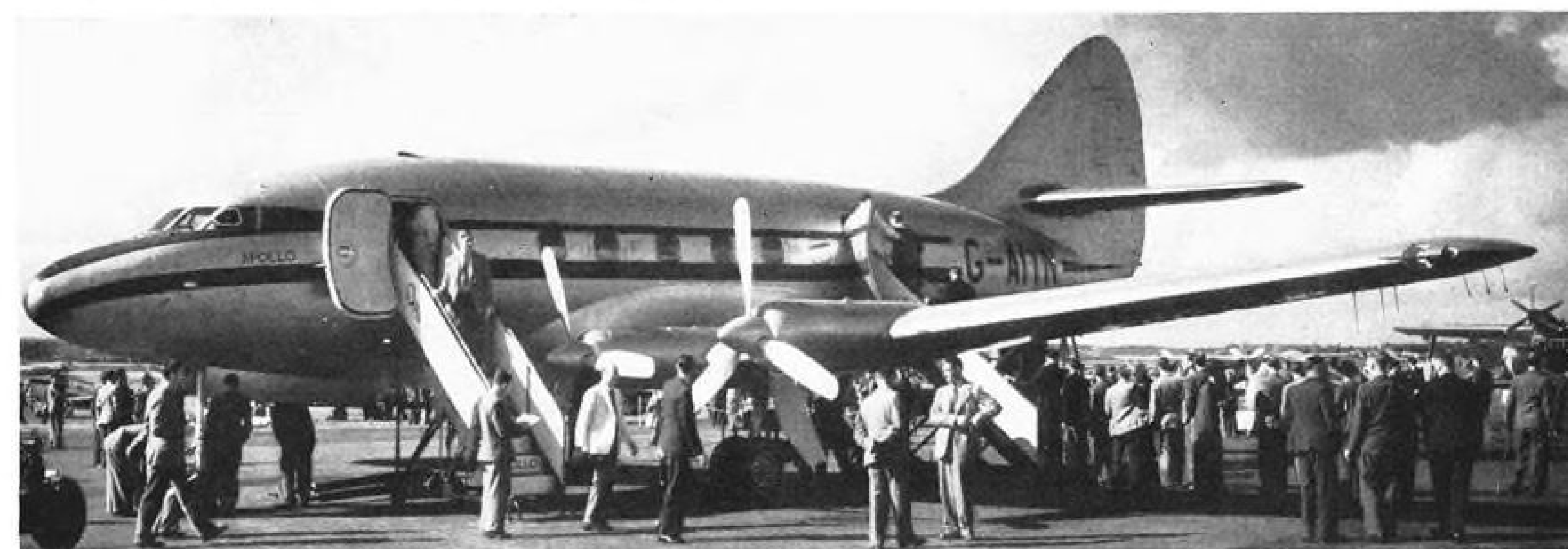
APOLLO LOADING of its 28-32 passengers can be accomplished easily and quickly through doors located both fore and aft of wing.
