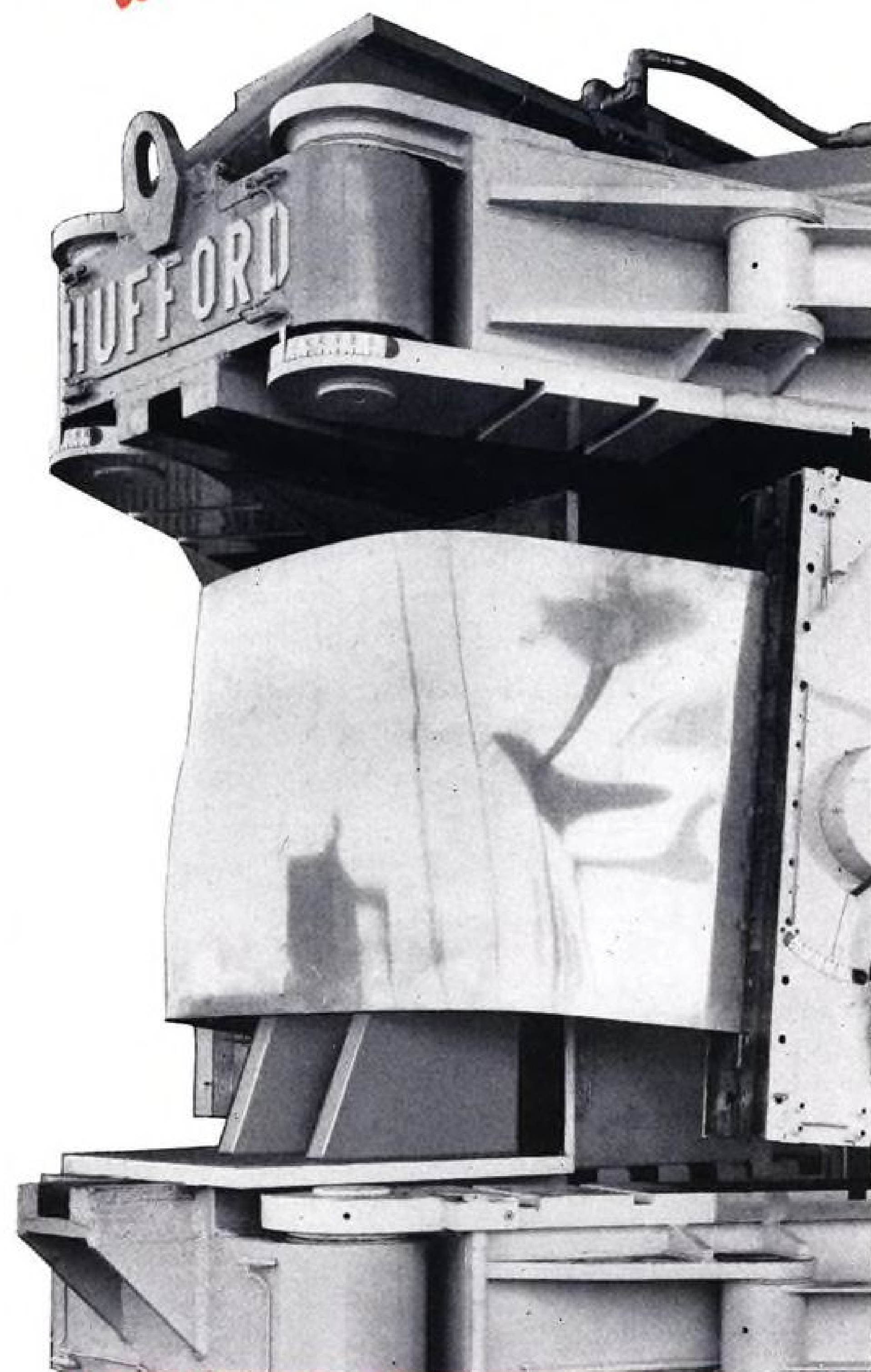
All modern Hufford machines handle both sheets and extrusions. Above are typical contours formed from extrusions. At right, model 46 stretch-wrap forms a large sheet.
