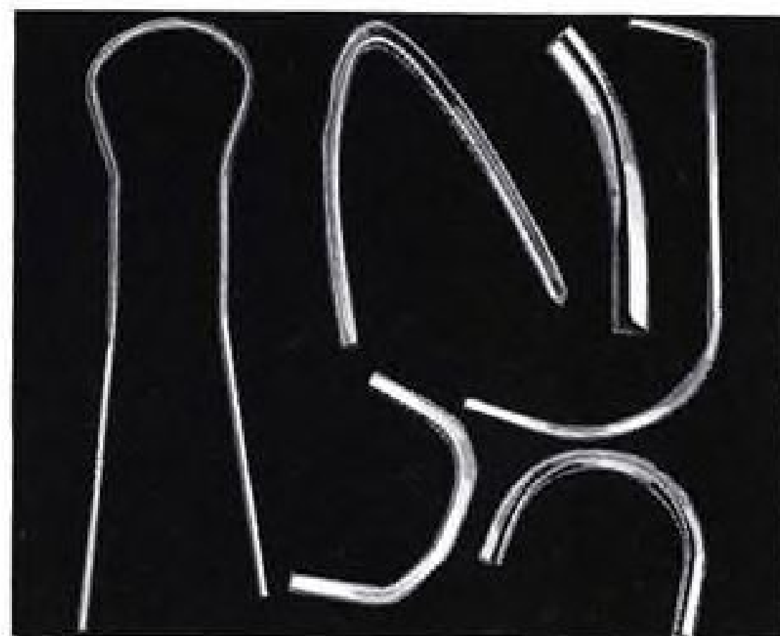
All modern Hufford machines handle both sheets and extrusions. Above are typical contours formed from extrusions. At right, model 46 stretch-wrap forms a large sheet.
