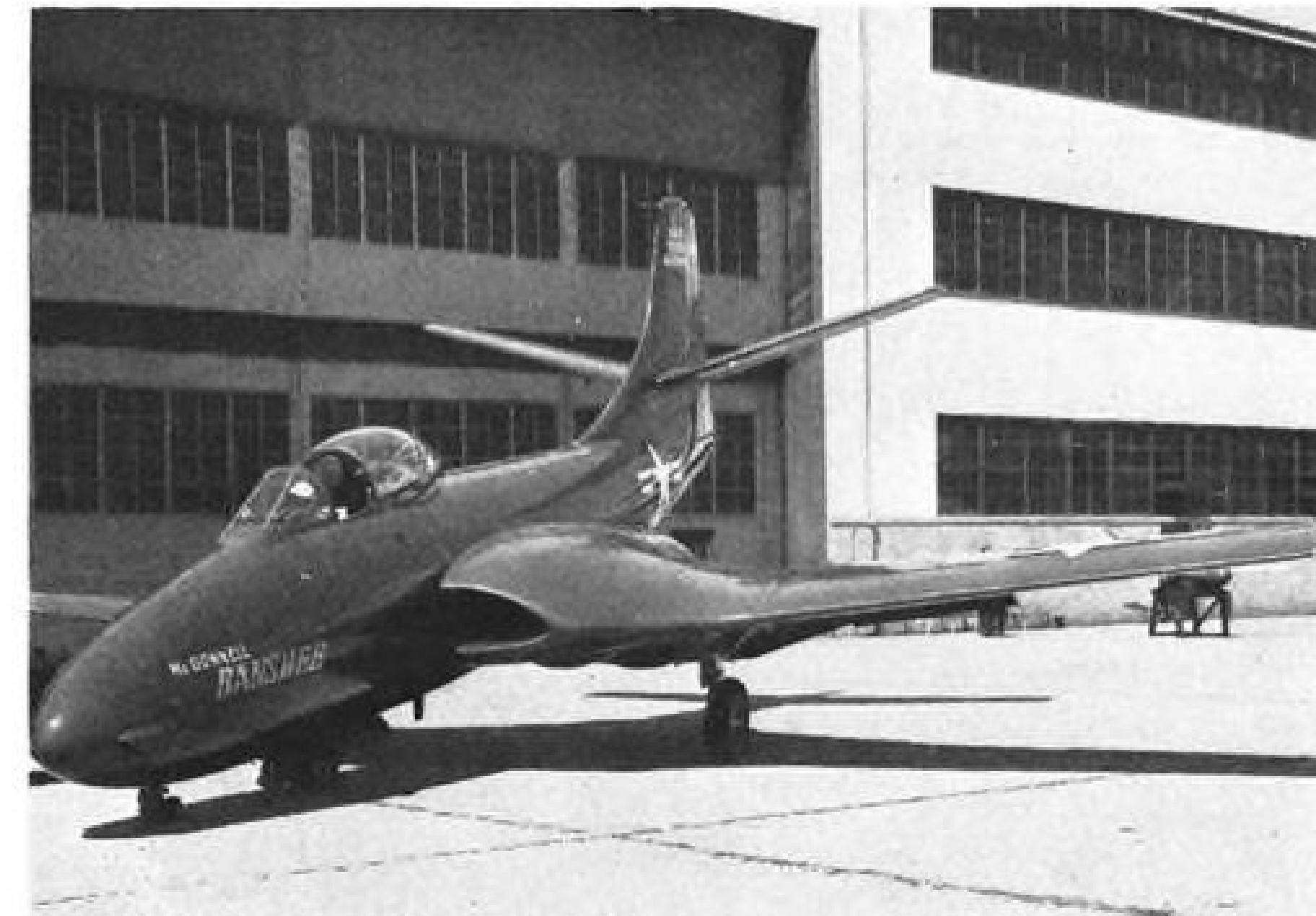
KNEELING GEAR on nosewheel simplifies problem of stowage on carrier deck.
