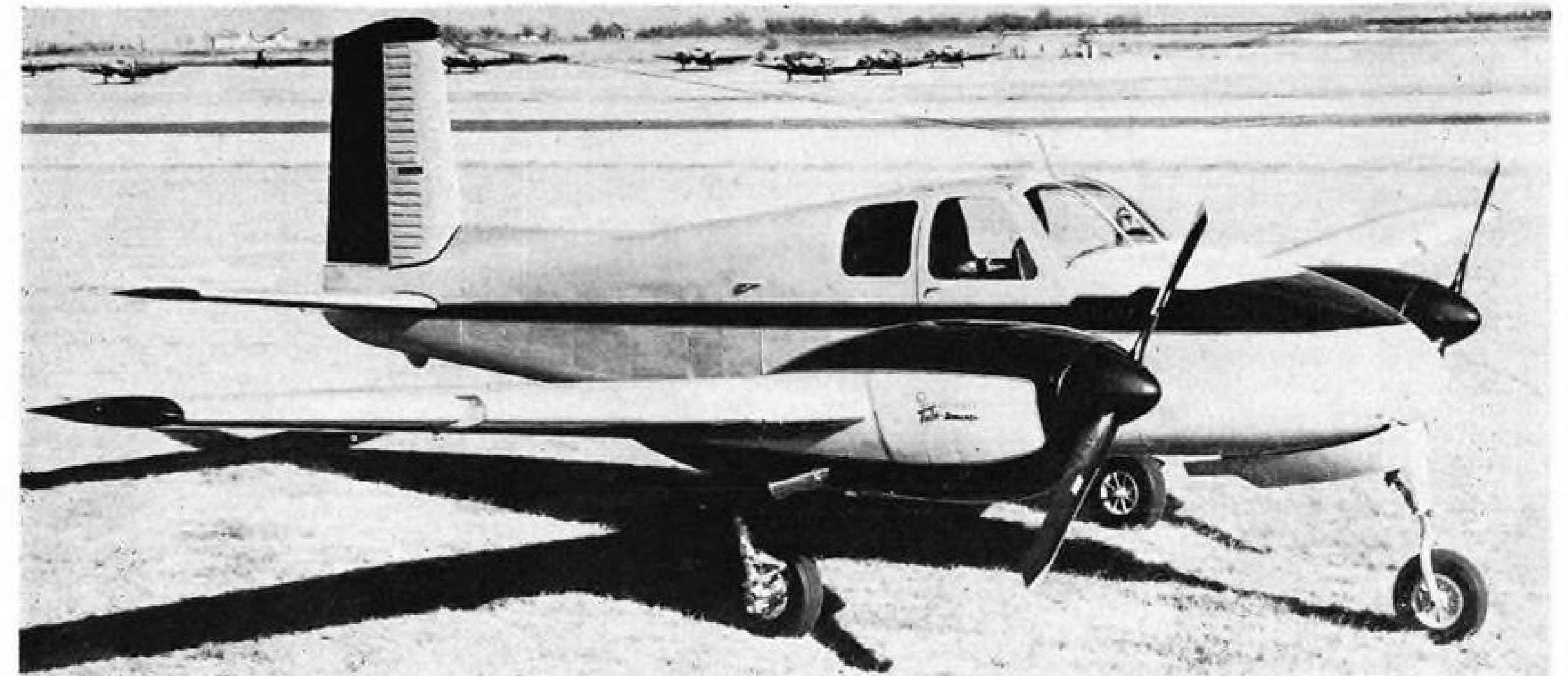
CONVENTIONAL SINGLE TAILFIN on Twin Bonanza replaces V-tail of smaller Bonanza. Craft is rated for 180 mph. cruising speed.
