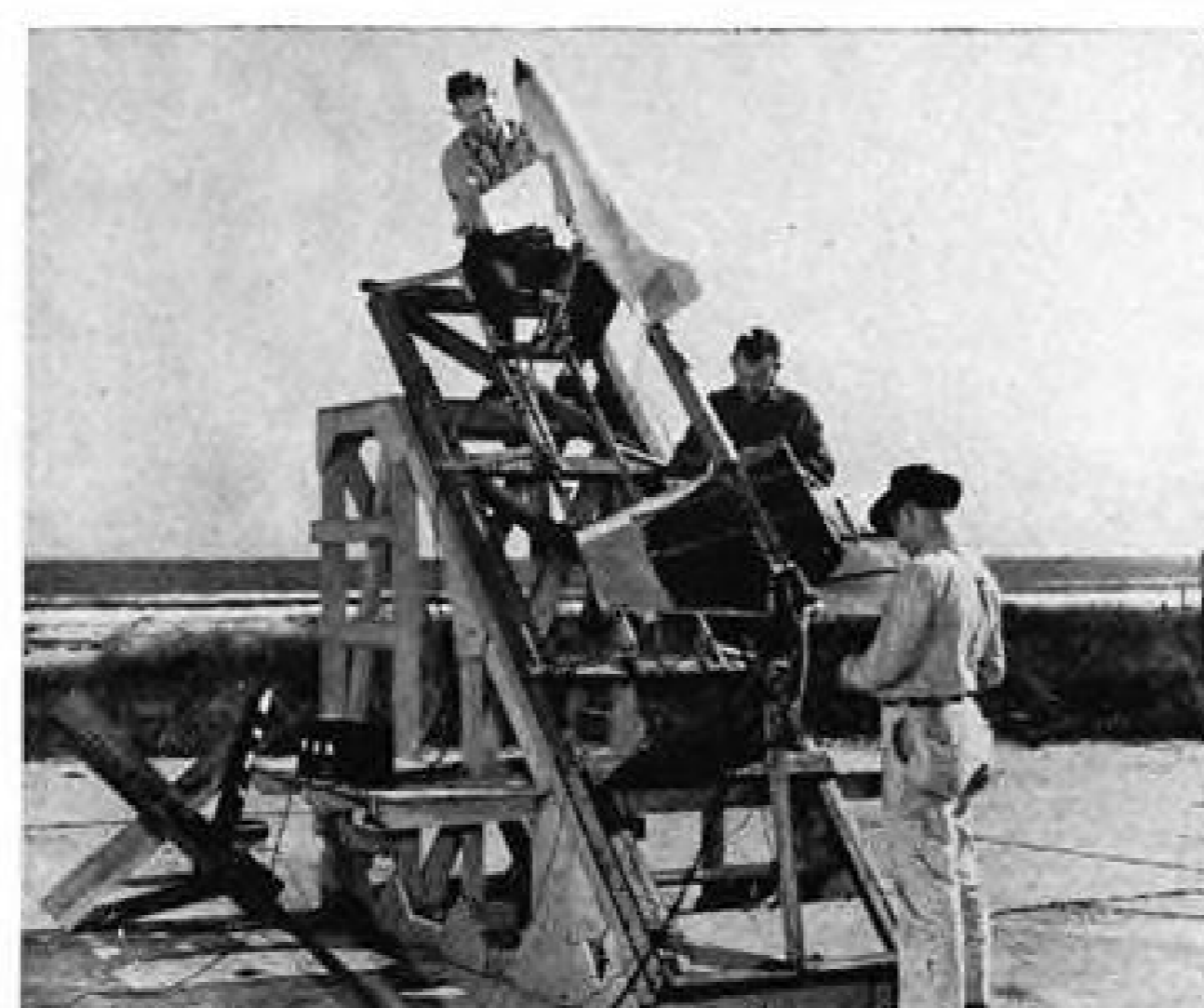
in preparation for launching, telemeters longitudinal and normal accelerations from which lift and drag data can be computed.
