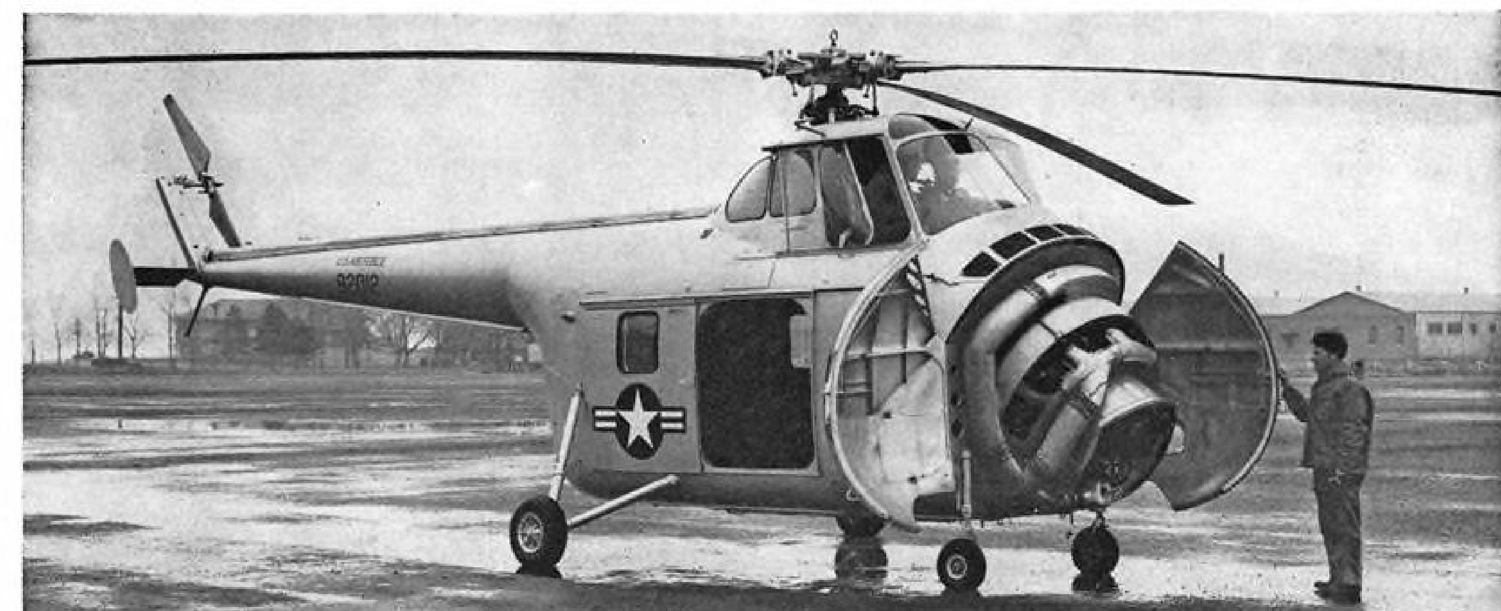
RADICAL FEATURES in helicopter design are shown in H-19: Clamshell doors for engine accessibility; large cabin below flight deck.
