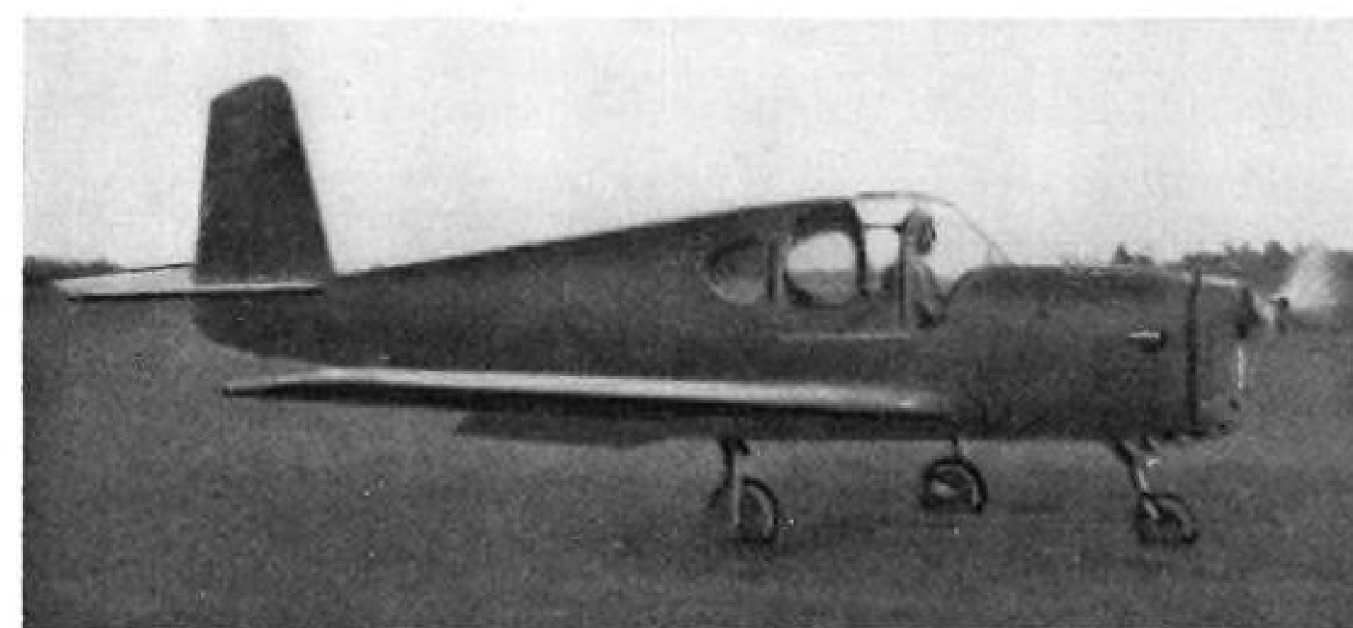
PRETI P.110 four-placer is of all-wood construction and is powered by a 140-hp. Alfa Romeo. Gross weight is about 2200 lb., top speed about 170 mph., and range is 621 mi.
