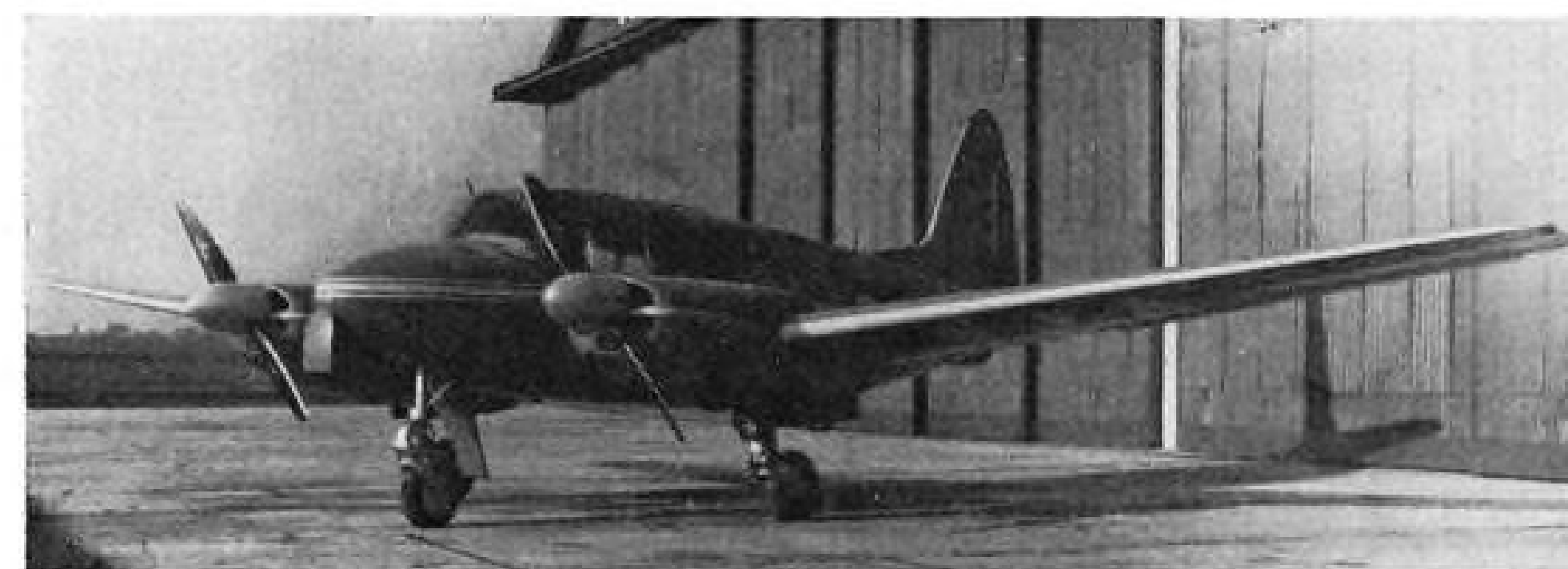
MACCHI MB.320 is new Italian 6-place light transport powered by two 185-hp. Continentals. Of all-metal construction, craft is said to have top speed of about 200 mph.
