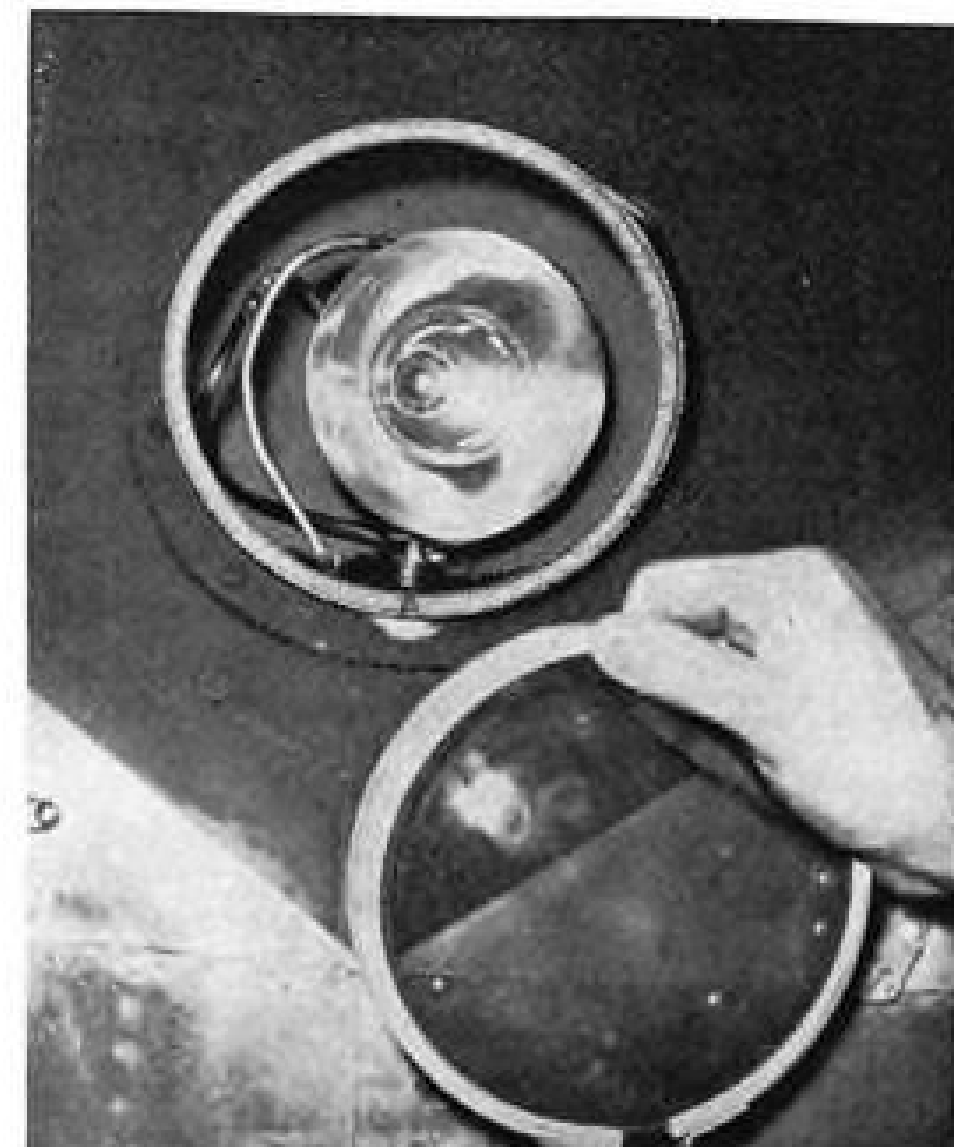
EXPERIMENTAL INSTALLATION of 10,000-candlepower sweep beam light on DC-3. Closeup shows light with red glass removed.
