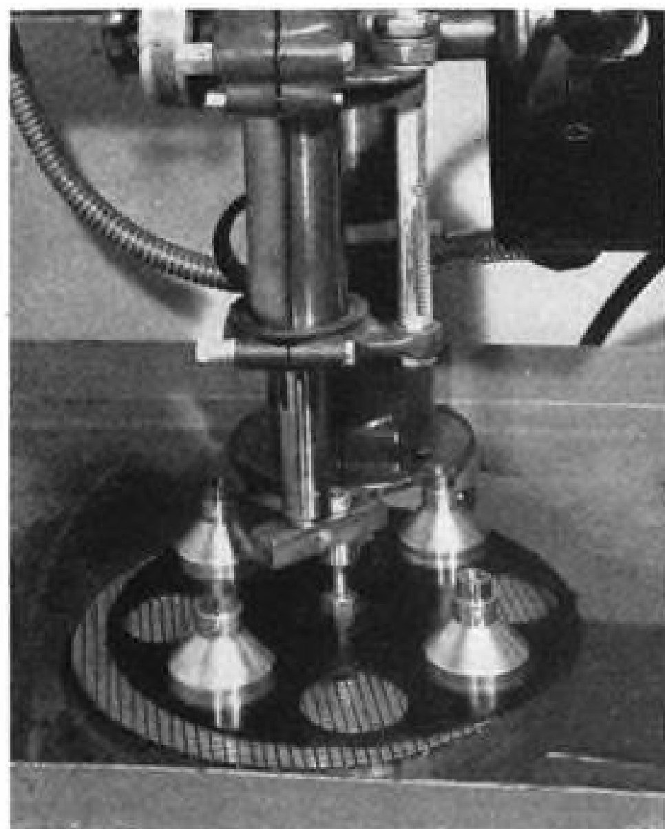
Another satisfactory lapping apparatus is the "inkwell" model. Four assembled units are shown ready to be driven over lap.
