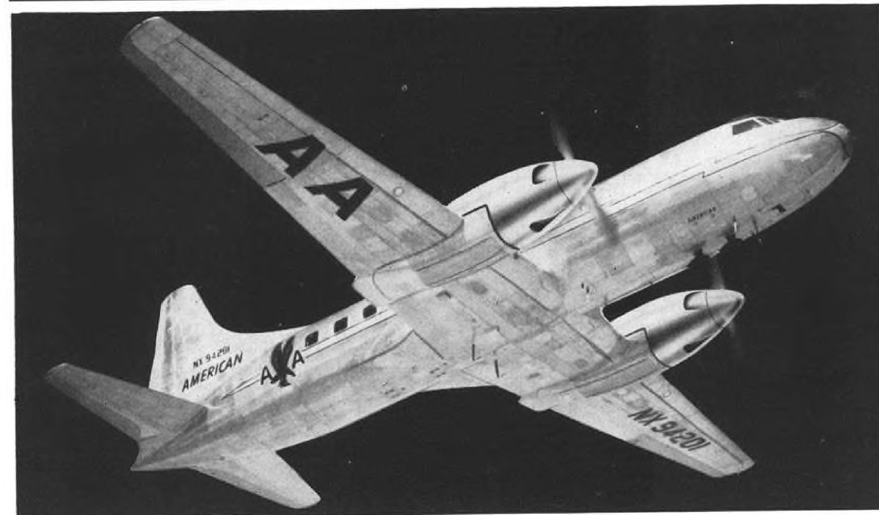
TURBOPROP ENGINES, sketched on photo of typical Convair-Liner, are power packages forward and above heavy black lines.
