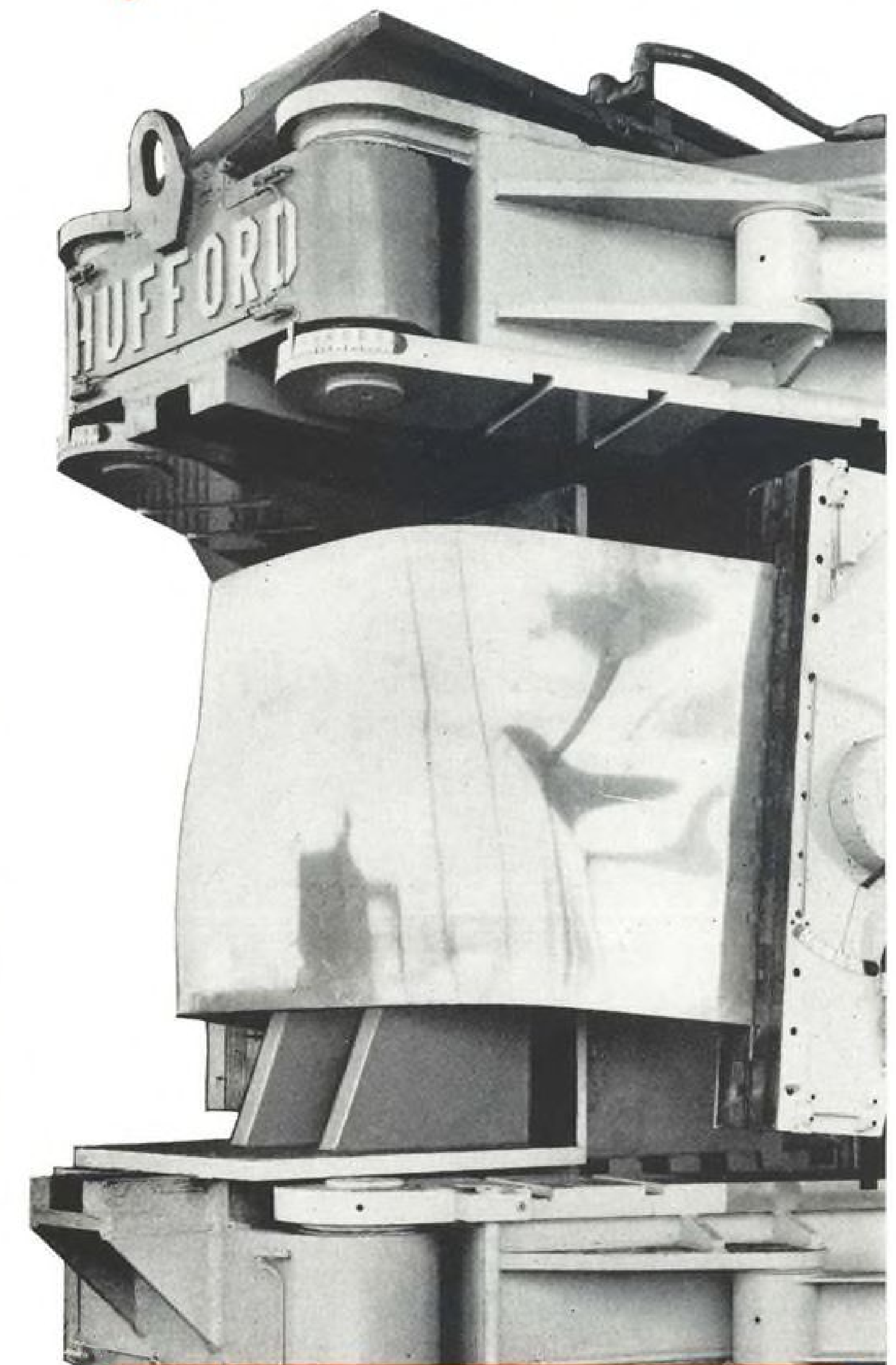
All modern Hufford machines handle both sheets and extrusions. Above are typical contours formed from extrusions. At right, model 46 stretch-wrap forms a large sheet.
