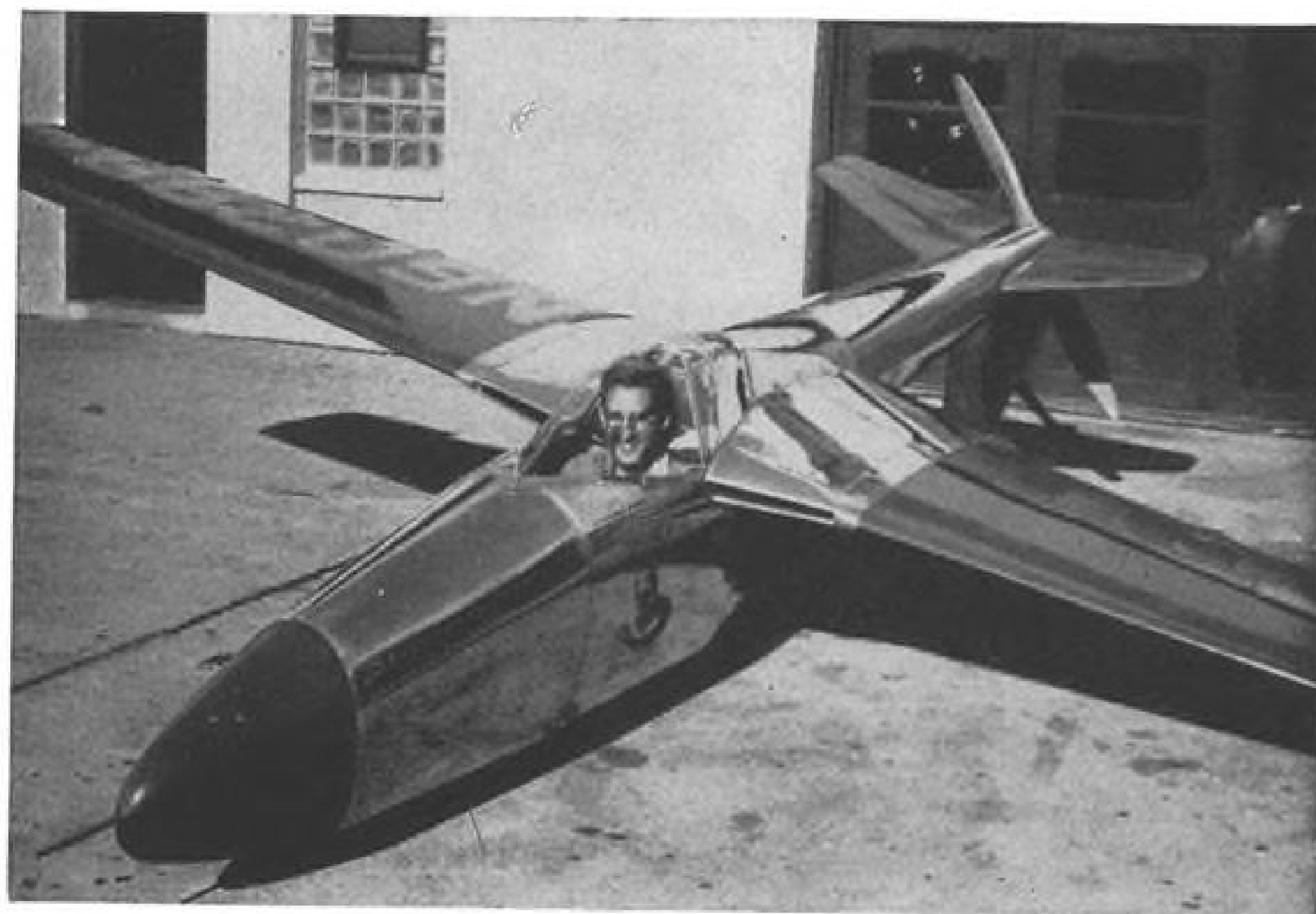
. . . Designer Paul M. Schroeder (in cockpit) who reports that his plane has 220-mph. top speed using buried Continental driving extension shaft to prop mounted behind tail.
