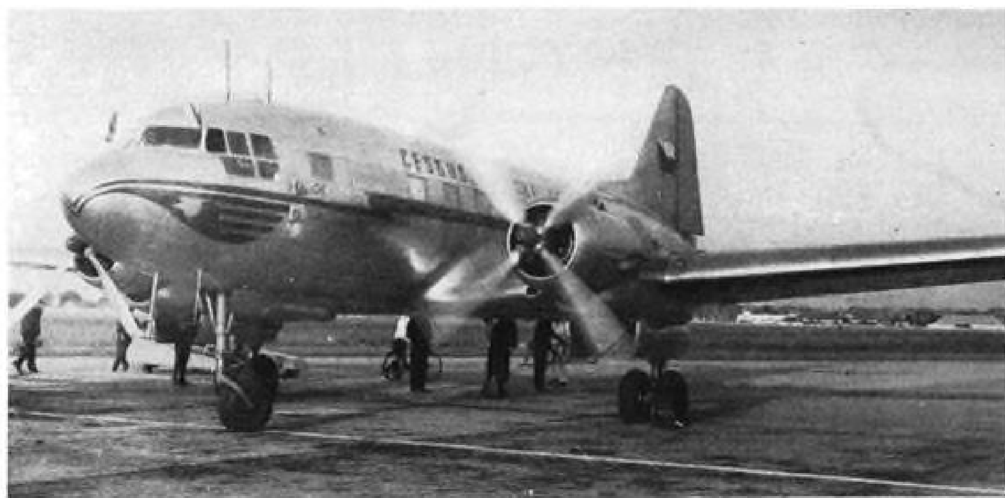
IL 12 uses four-bladed props, has excellent visibility downward from cockpit.
