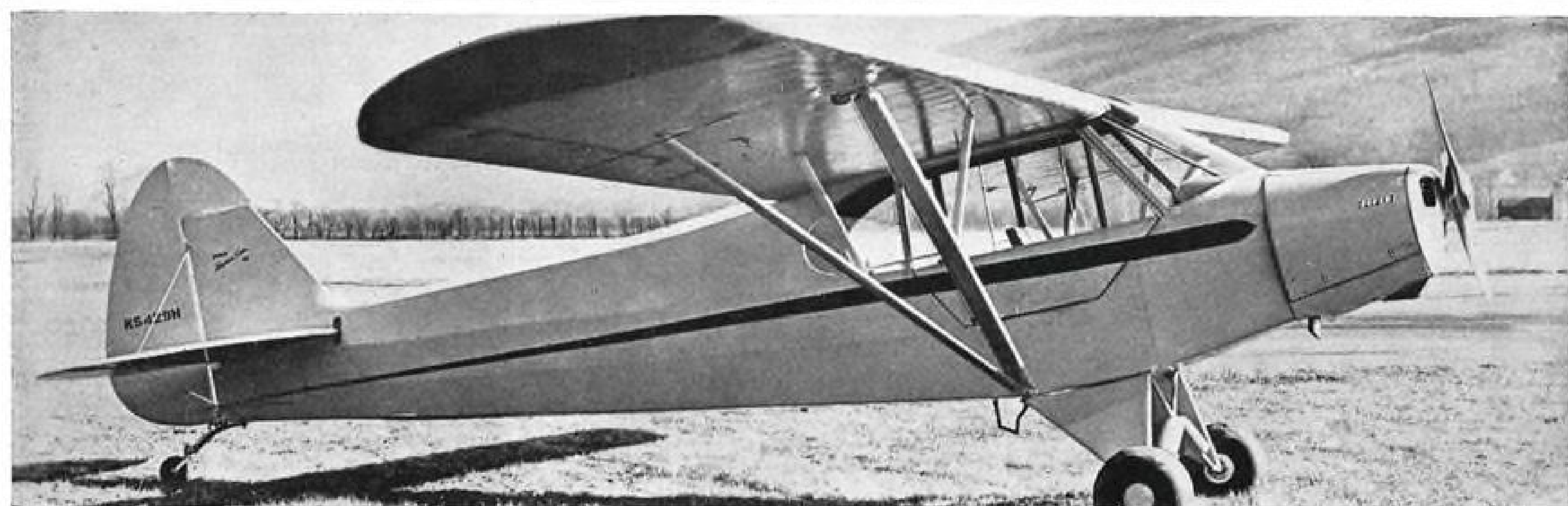
PIPER'S 1950 SUPER CUB carries 400-lb. in bulky loads. Flaps and balanced elevators are standard on Lycoming-engine version.
