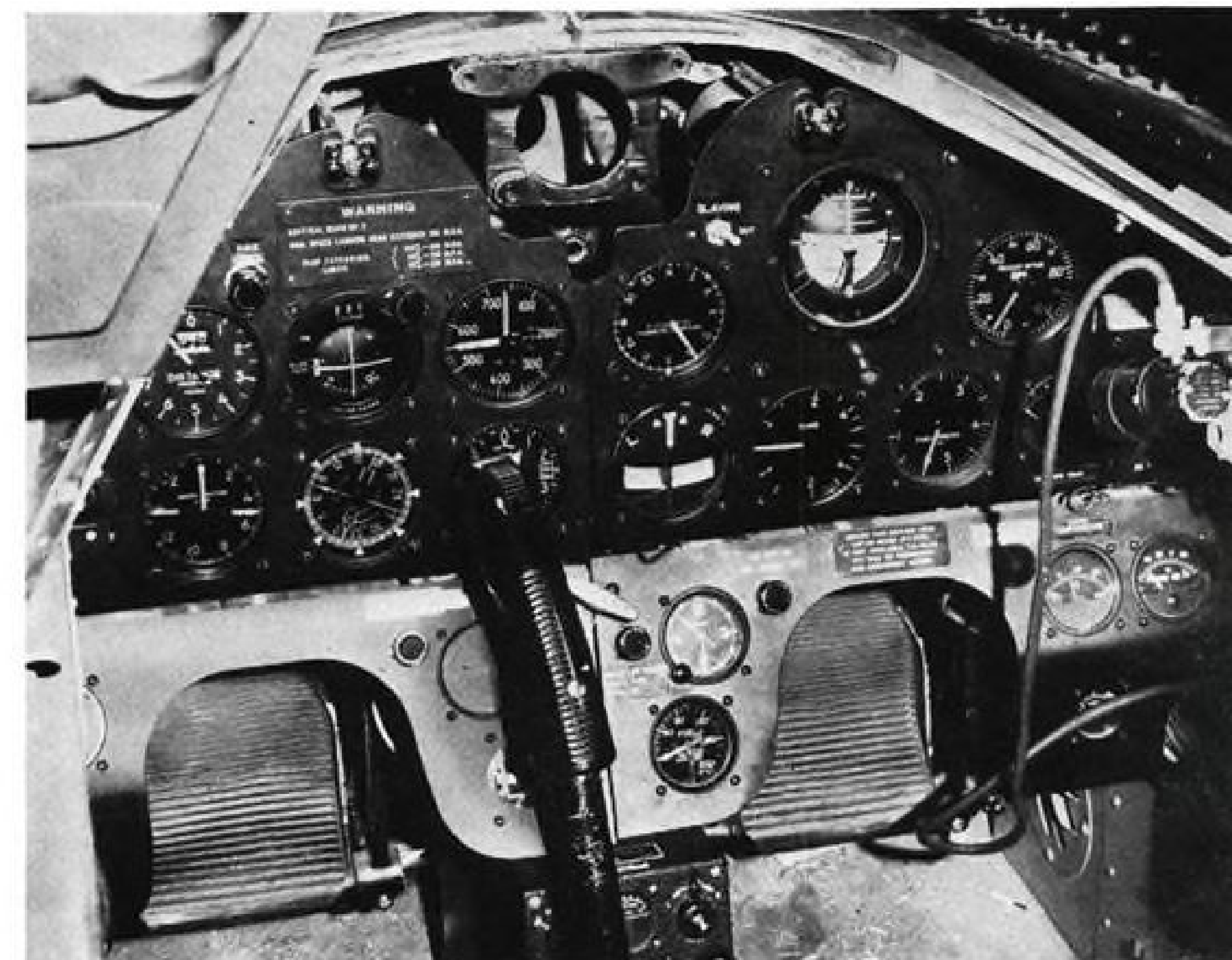
STUDENT "flies" with this full array of jet fighter instruments and controls. Connected to electronic-servo system they react precisely as in real flight, while . . .
