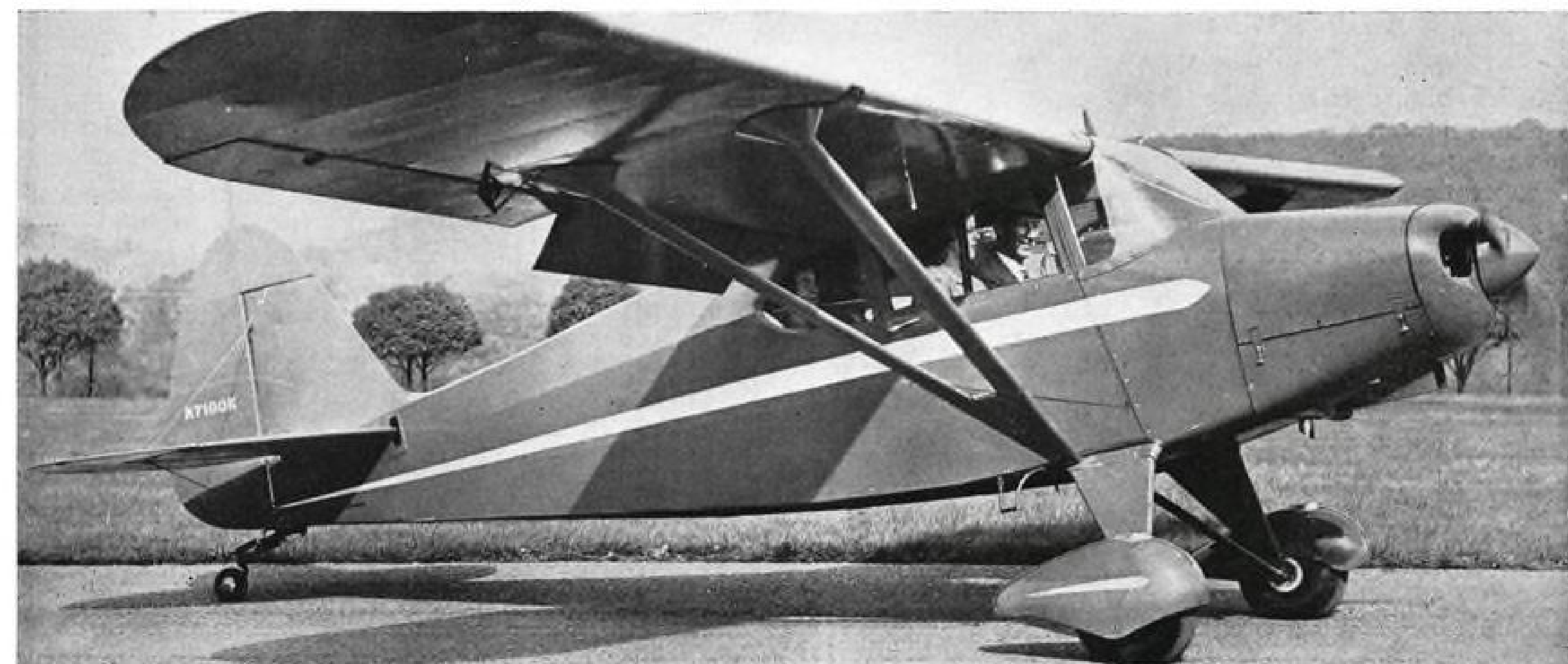
PIPER PACER shows detail improvement over Clipper, including better streamlining. The 135-hp. Lycoming model has Aeromatic prop.
